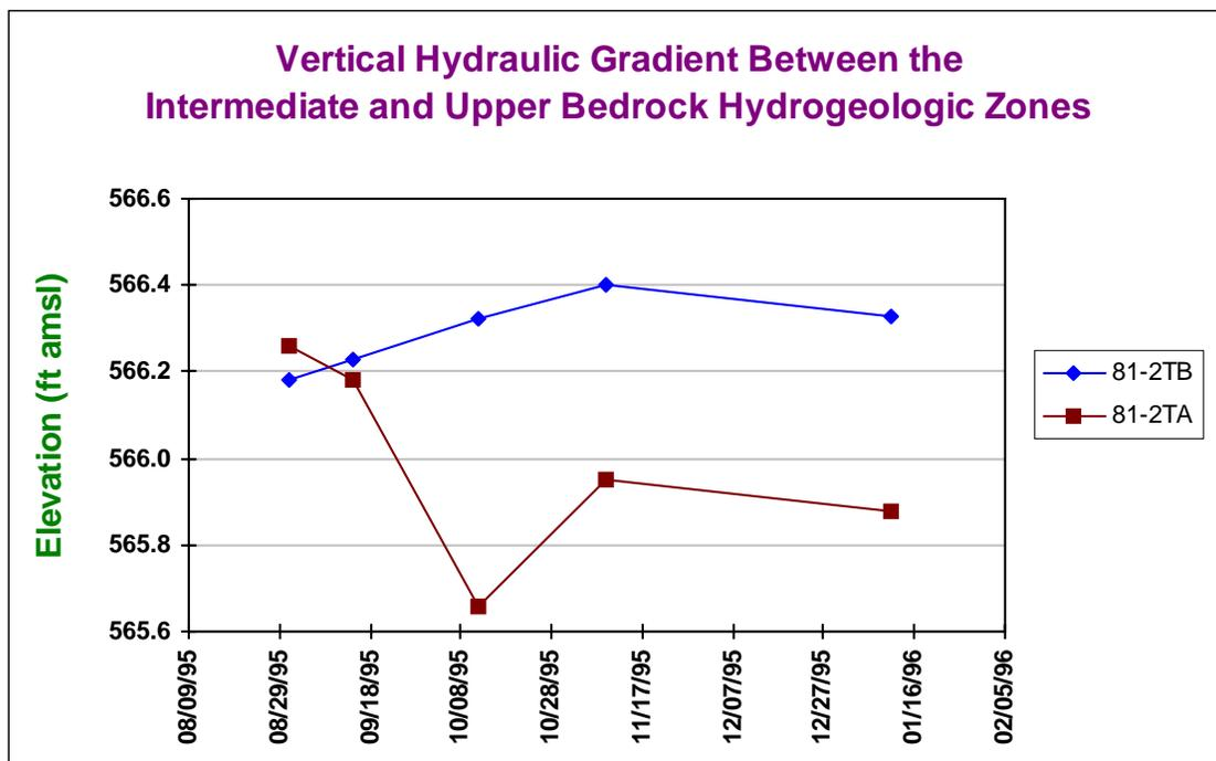
**Figure 6-22. Vertical Hydraulic Gradient Between the Intermediate and Upper Bedrock Zones Within the Tonawanda Study Area. The Intermediate Zone Well Is Denoted by Blue Diamonds, While the Upper Bedrock Zone Well Is Denoted by Brown Squares.**
