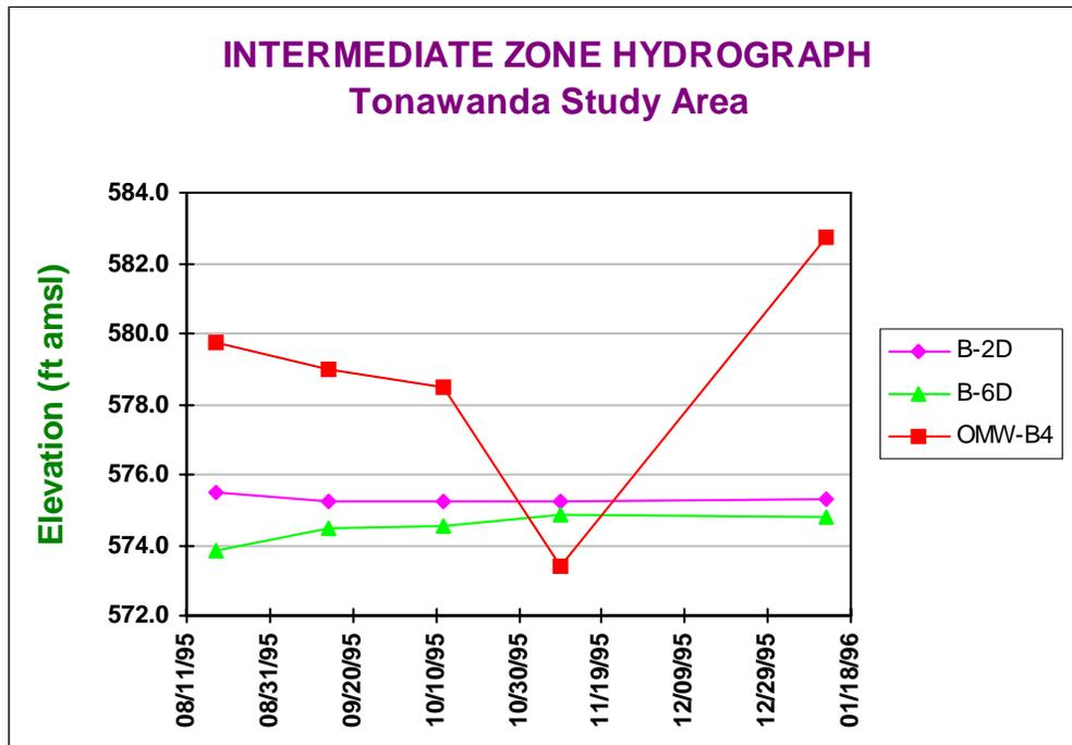
**Figure 6-9. Intermediate Zone Hydrograph for the Tonawanda Study Area. Solid Lines Denote Glaciolacustrine Wells.**
