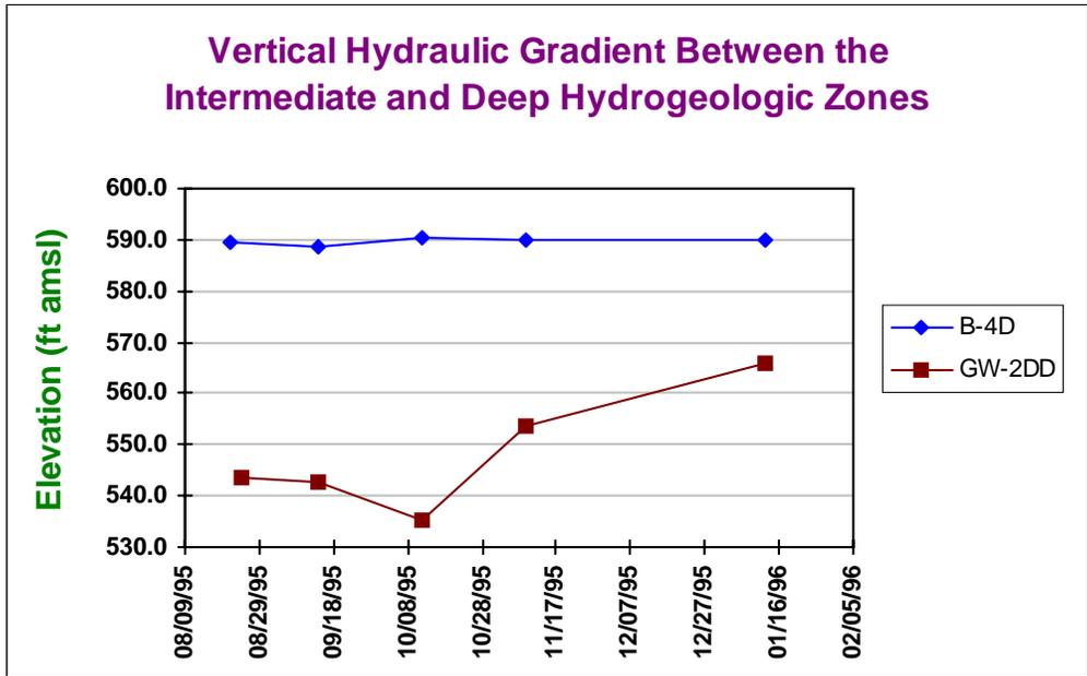
Figure 6-19. Vertical Hydraulic Gradient Between the Intermediate and Deep Zones Within the Tonawanda Study Area. The Intermediate Zone Well Is Denoted by Blue Diamonds, While the Deep Zone Well Is Denoted by Brown Squares.
