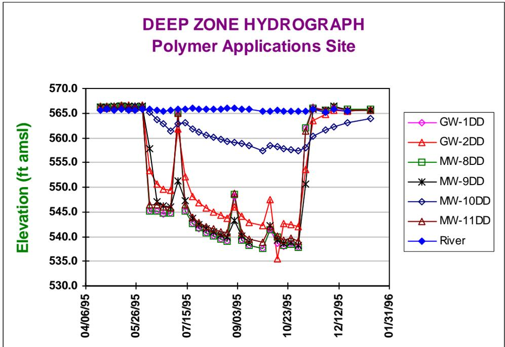
Figure 6-15. Deep Zone Hydrograph for the Tonawanda Study Area.
