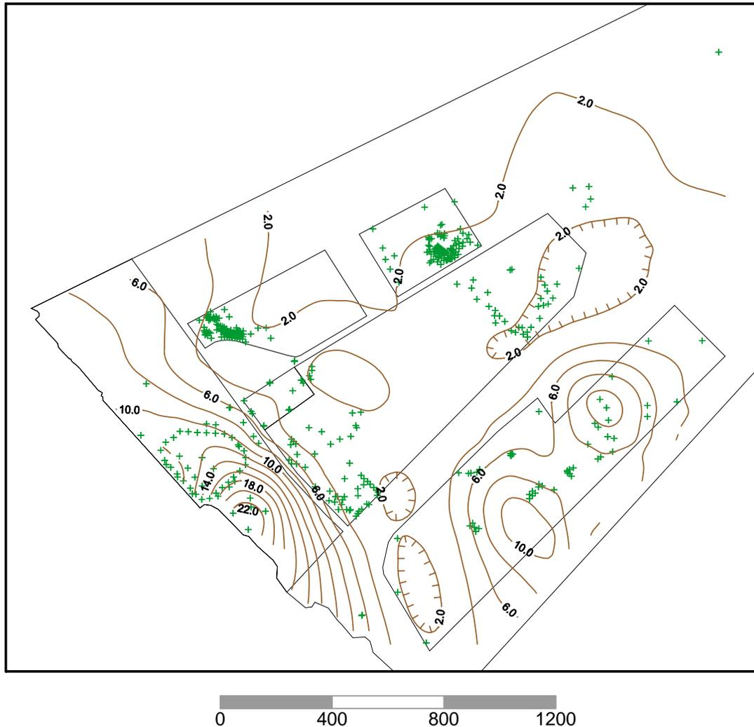
**Figure 5-3. Fill Thickness Contour of the Study Area. Boring, Monitoring Well and Test Pit Locations are Shown as Crosses. Scale in Meters.**
