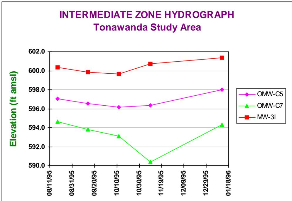
Figure 6-8. Intermediate Zone Hydrograph for the Tonawanda Study Area. Solid Lines Denote Glaciolacustrine Wells.
