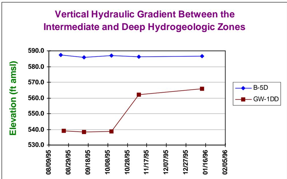
Figure 6-20. Vertical Hydraulic Gradient Between the Intermediate and Deep Zones Within the Tonawanda Study Area. The Intermediate Zone Well Is Denoted by Blue Diamonds, While the Deep Zone Well Is Denoted by Brown Squares.
