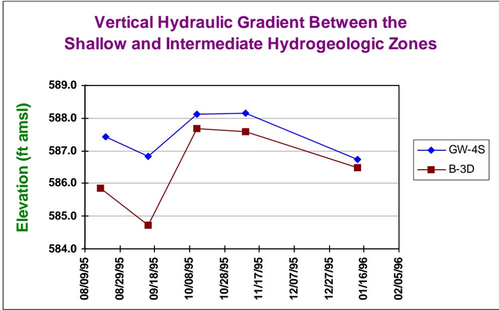
**Figure 6-12. Vertical Hydraulic Gradient Between the Shallow and Intermediate Zones Within the Tonawanda Study Area. The Shallow Zone Well Is Denoted by Blue Diamonds, While the Intermediate Zone Well Is Denoted by Brown Squares.**
