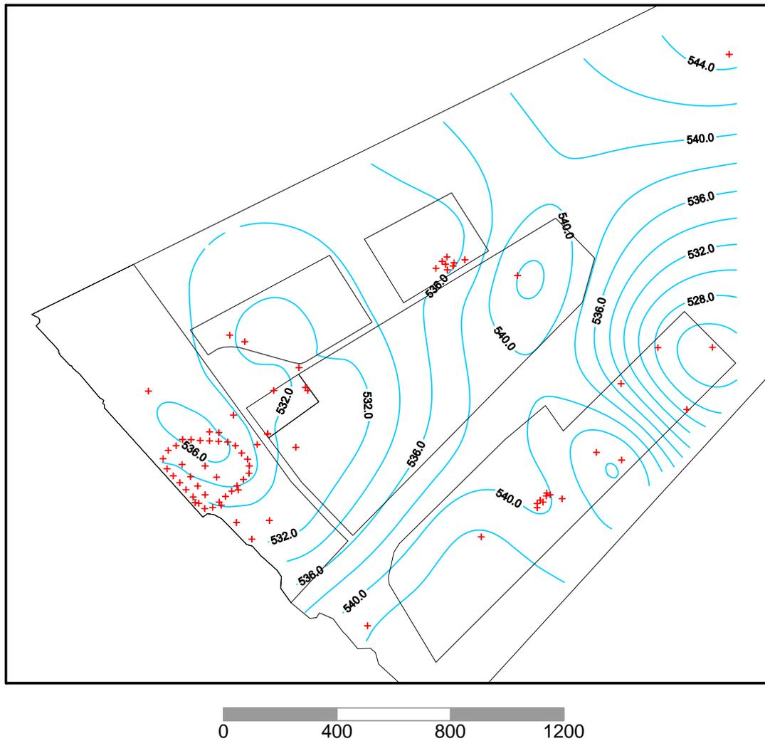
**Figure 5-7. Glacial Till Surface Contour of the Study Area. Boring and Monitoring Well Locations are Shown as Crosses. Scale in Meters.**
