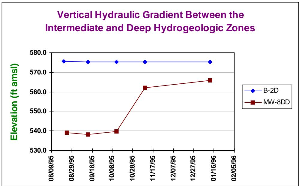
Figure 6-18. Vertical Hydraulic Gradient Between the Intermediate and Deep Zones Within the Tonawanda Study Area. The Intermediate Zone Well Is Denoted by Blue Diamonds, While the Deep Zone Well Is Denoted by Brown Squares.
