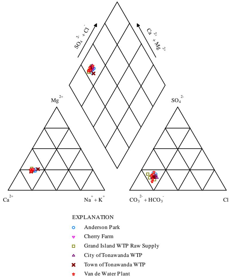
**Figure 7-1. Piper Diagram Showing the Ionic Composition of Water from the Niagara River in the Tonawanda Area.**
