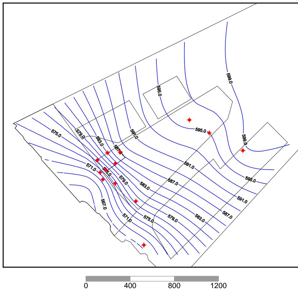
**Figure 6-10. Intermediate Zone Groundwater Flow Across the Study Area on September 14, 1995. Wells are Shown as Red Crossed Dots. Scale in Meters.**
