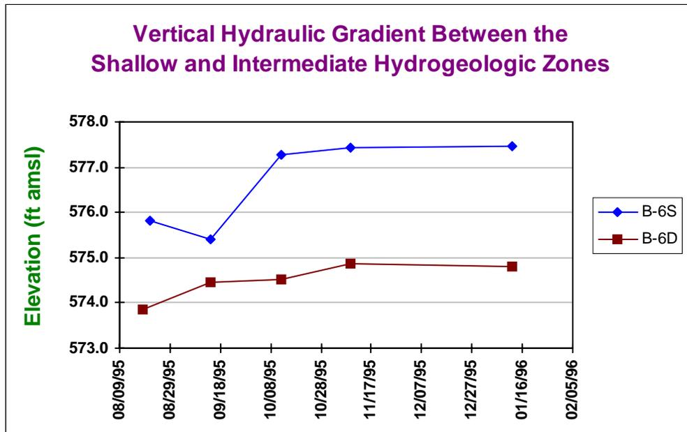
**Figure 6-14. Vertical Hydraulic Gradient Between the Shallow and Intermediate Zones Within the Tonawanda Study Area. The Shallow Zone Well Is Denoted by Blue Diamonds, While the Intermediate Zone Well Is Denoted by Brown Squares.**
