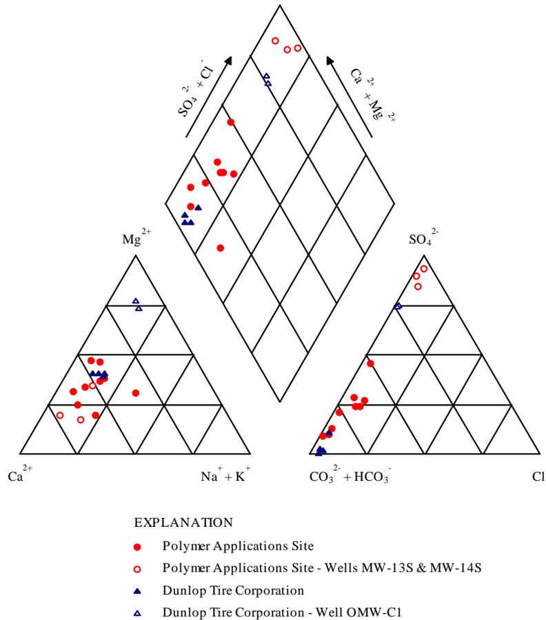
**Figure 7-4. Piper Diagram Showing the Ionic Composition of Water from the Shallow Hydrogeologic Zone Within the Tonawanda Study Area.**
