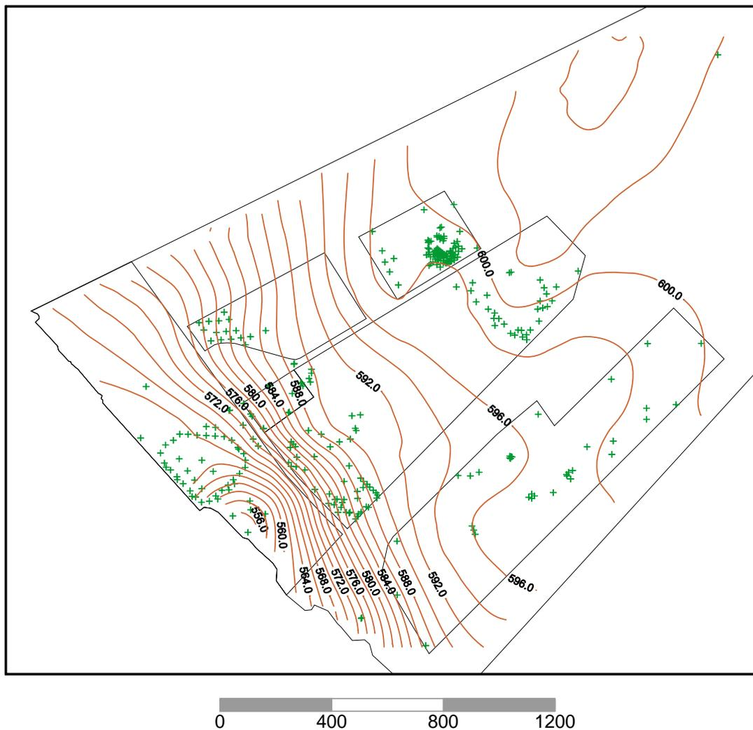
**Figure 5-4. Native Soil Surface Contour of the Study Area. Boring, Monitoring Well and Test Pit Locations are Shown as Crosses. Scale in Meters.**
