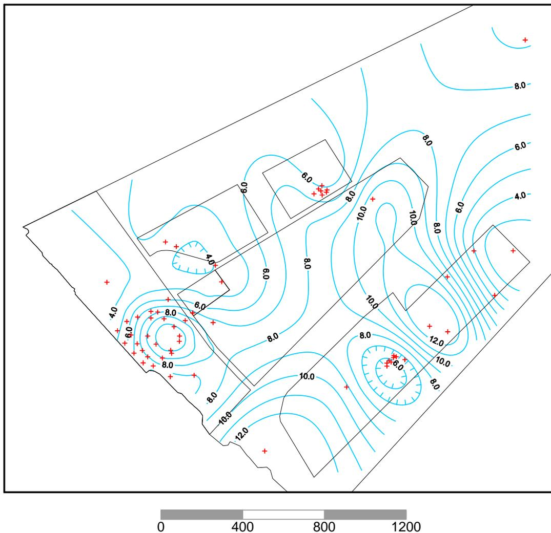
**Figure 5-6. Glacial Till Thickness Contour of the Study Area. Boring and Monitoring Well Locations are Shown as Crosses. Scale in Meters.**
