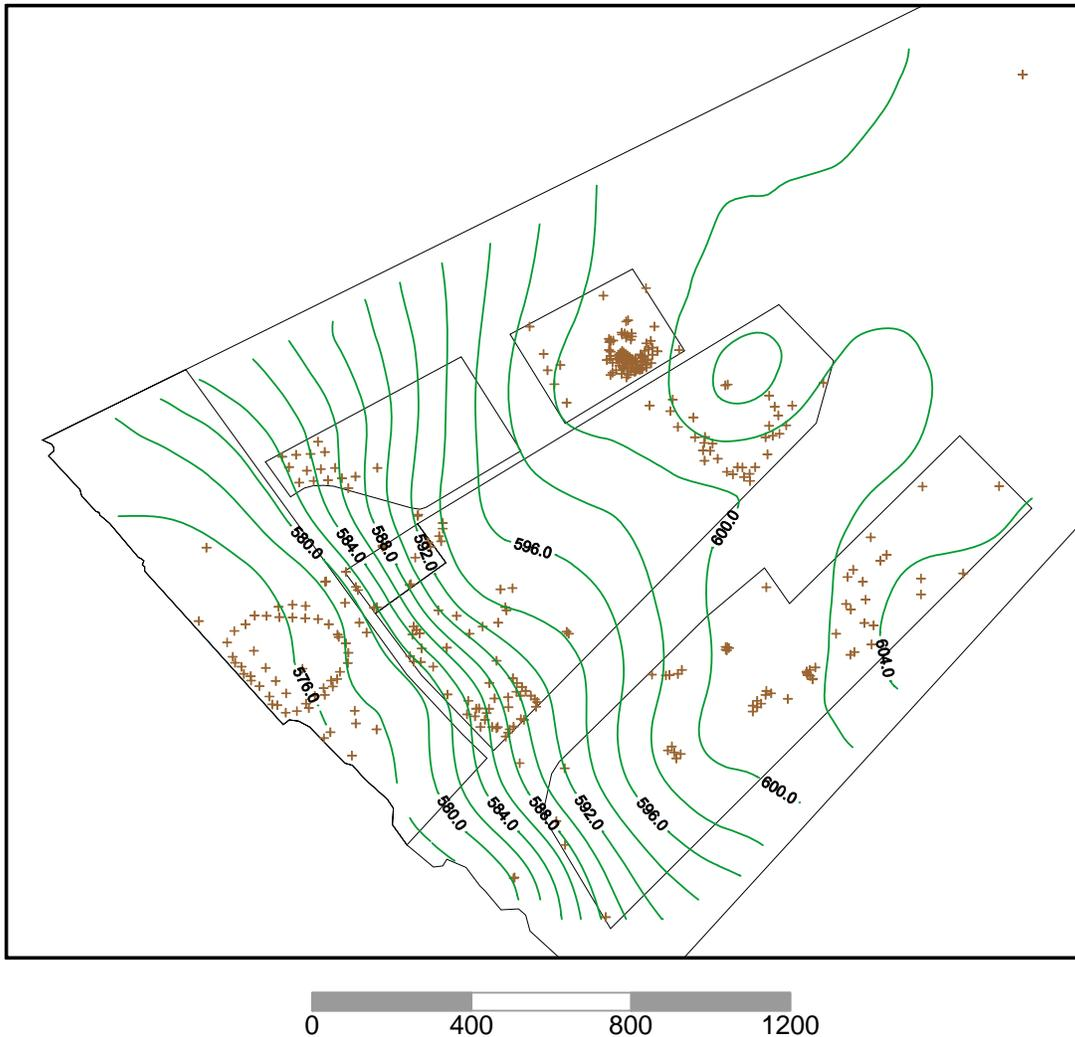
**Figure 5-5. Surface Topography Contour of the Study Area. Boring, Monitoring Well and Test Pit Locations are Shown as Crosses. Scale in Meters.**
