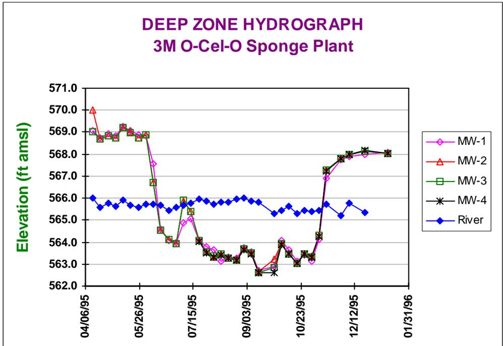
Figure 6-17. Deep Zone Hydrograph for the Tonawanda Study Area.
