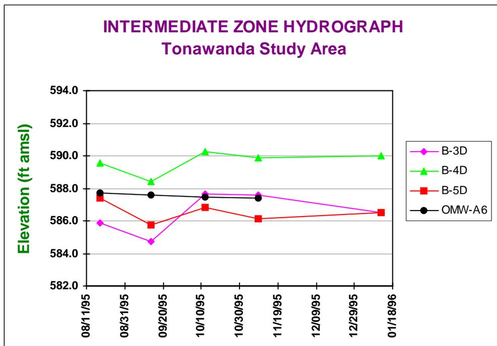
**Figure 6-6. Intermediate Zone Hydrograph for the Tonawanda Study Area. Solid Lines Denote Glaciolacustrine Wells.**
