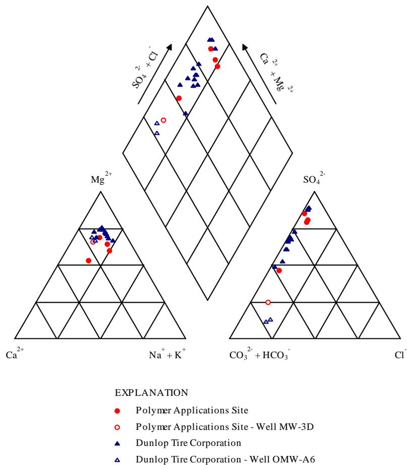
**Figure 7-5. Piper Diagram Showing the Ionic Composition of Water from the Intermediate Hydrogeologic Zone Within the Tonawanda Study Area.**
