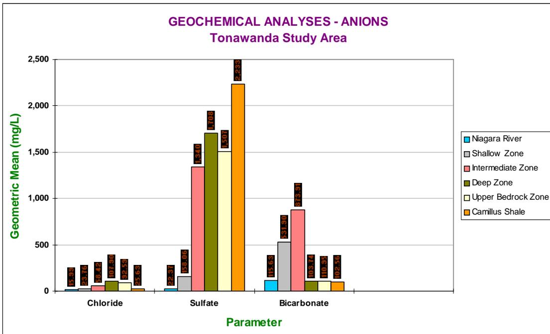
**Figure 7-2. Major Cation and Anion Data from the Study Area Showing Variations in Geometric Means for the Hydrogeologic Zones Evaluated in this Study.**
