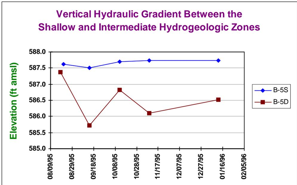
**Figure 6-13. Vertical Hydraulic Gradient Between the Shallow and Intermediate Zones Within the Tonawanda Study Area. The Shallow Zone Well Is Denoted by Blue Diamonds, While the Intermediate Zone Well Is Denoted by Brown Squares.**
