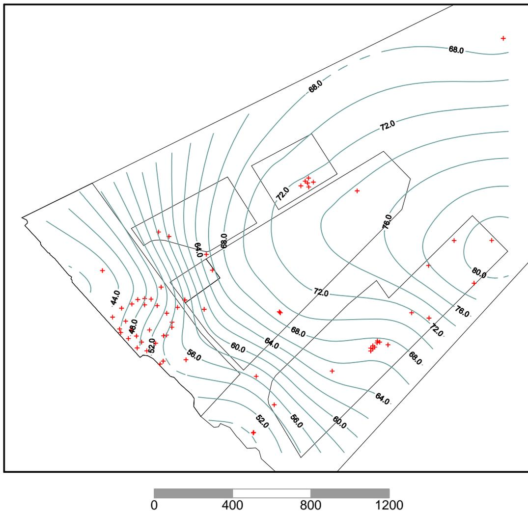
**Figure 5-8. Depth to Bedrock Contour of the Study Area. Boring and Monitoring Well Locations are Shown as Crosses. Scale in Meters.**
