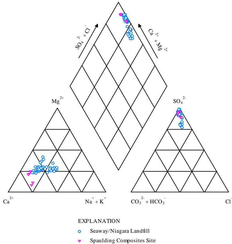
**Figure 7-8. Piper Diagram Showing the Ionic Composition of Water from the Upper Camillus Shale Bedrock in the Tonawanda Area.**
