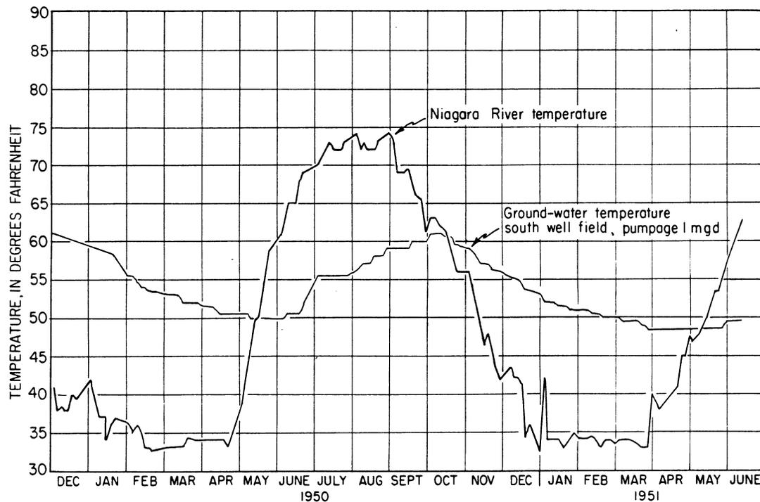
**Figure 3-3. Temperatures of Niagara River Water and Groundwater Extracted by the E.I. DuPont Yerkes Plant. From La Sala (1968).**
