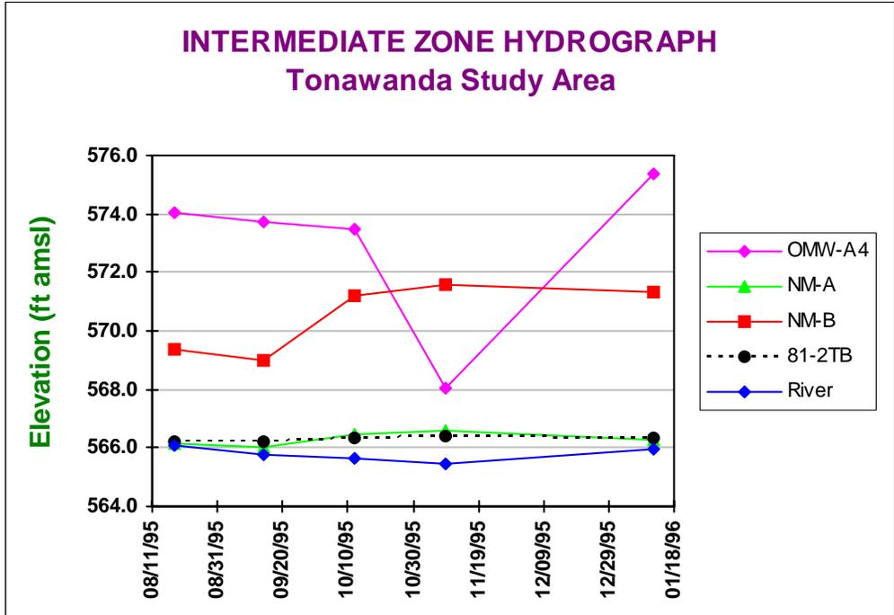
Figure 6-7. Intermediate Zone Hydrograph for the Tonawanda Study Area. Dashed Lines Denote Alluvium Wells. Solid Lines Denote Glaciolacustrine Wells.
