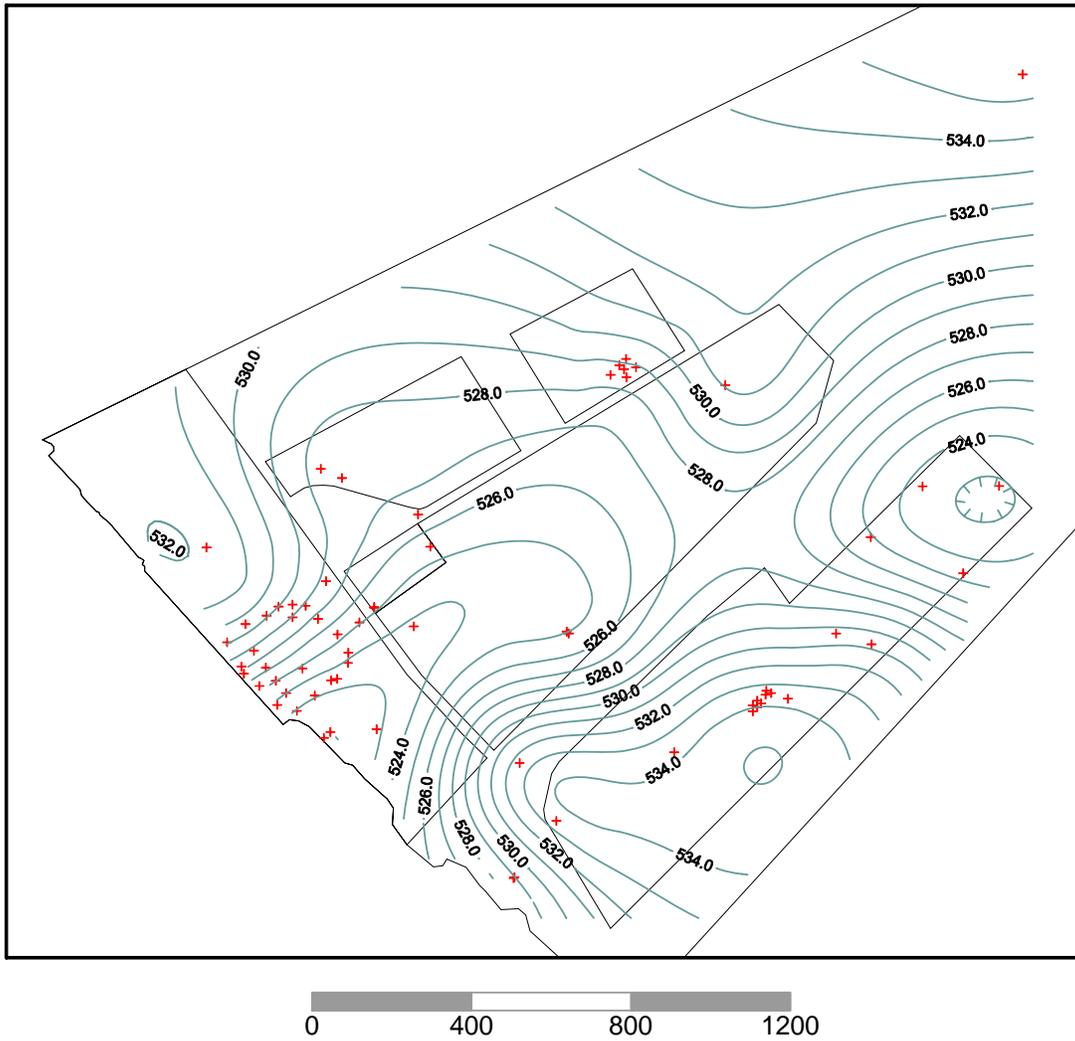
**Figure 5-9. Bedrock Surface Contour of the Study Area. Boring and Monitoring Well Locations are Shown as Crosses. Scale in Meters.**
