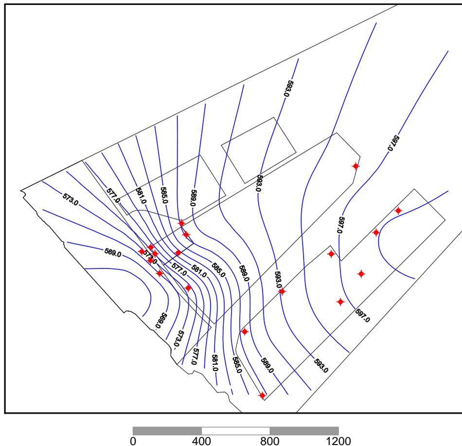
**Figure 6-4. Shallow Zone Groundwater Flow Across the Study Area on September 14, 1995. Wells are Shown as Red Crossed Dots. Scale in Meters.**
