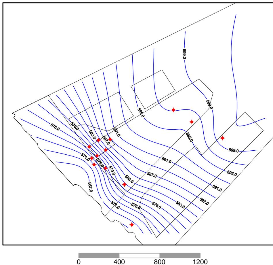
**Figure 6-11. Intermediate Zone Groundwater Flow Across the Study Area on January 12, 1996. Wells are Shown as Red Crossed Dots. Scale in Meters.**
