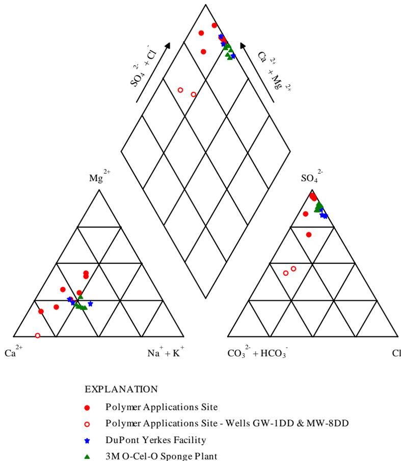
**Figure 7-6. Piper Diagram Showing the Ionic Composition of Water from the Deep Hydrogeologic Zone Within the Tonawanda Study Area.**
