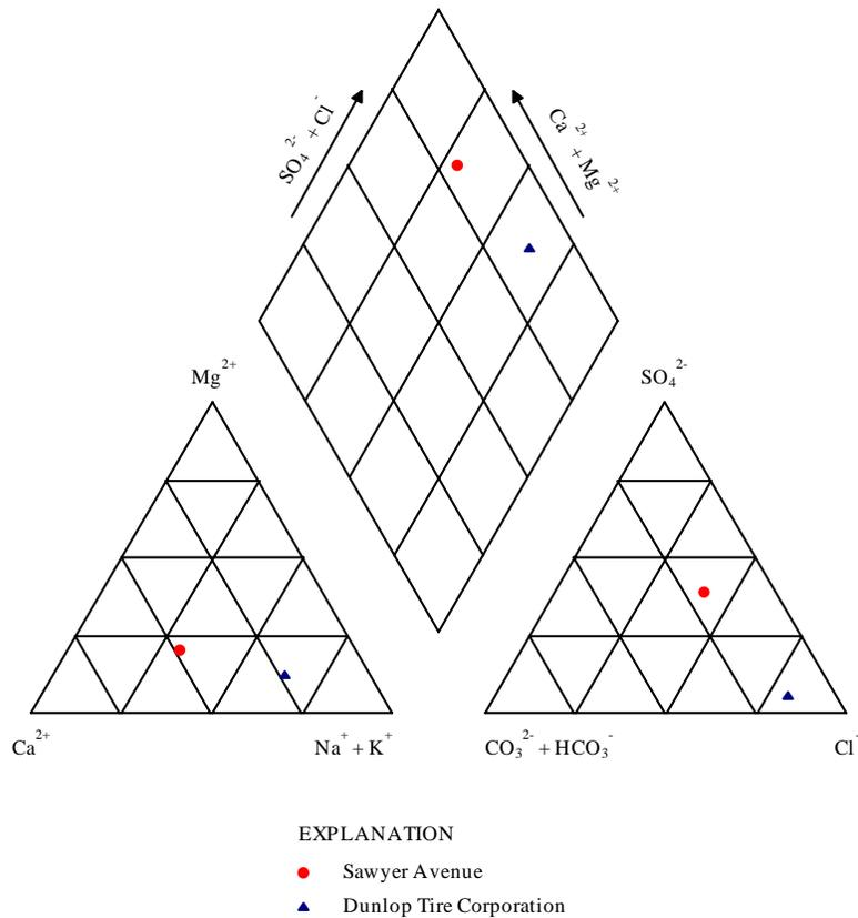
**Figure 7-3. Piper Diagram Showing the Ionic Composition of Water from the Wetlands Within the Tonawanda Study Area.**
