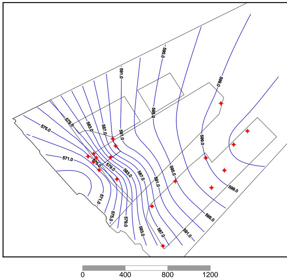
**Figure 6-5. Shallow Zone Groundwater Flow Across the Study Area on November 9, 1995. Wells are Shown as Red Crossed Dots. Scale in Meters.**
