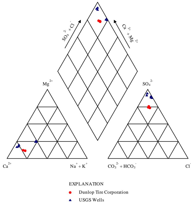
**Figure 7-7. Piper Diagram Showing the Ionic Composition of Water from the Upper Bedrock Hydrogeologic Zone Within the Tonawanda Study Area.**
