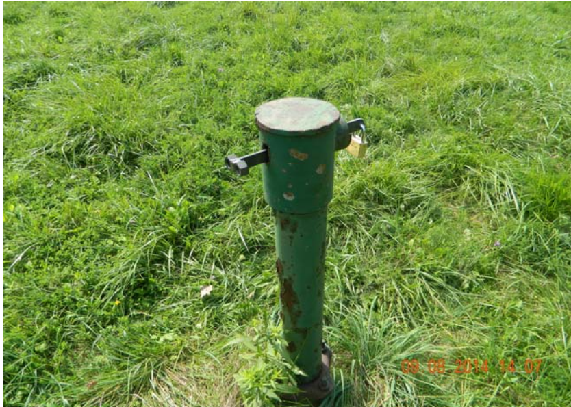
Repaired well cap anchor bolt and replacement lock on MW-6B
