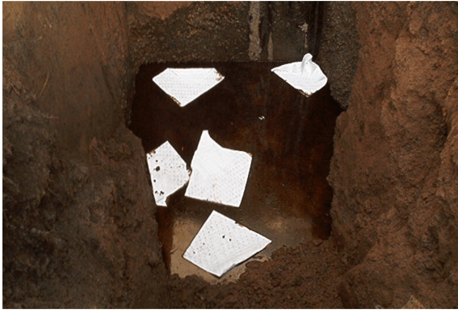
Figure 2-58. Photograph showing the NAPL encountered along the outside wall of the Spauldite Sheet basement. View looking northwest. Photograph taken by Glenn May on September 28, 2004.
