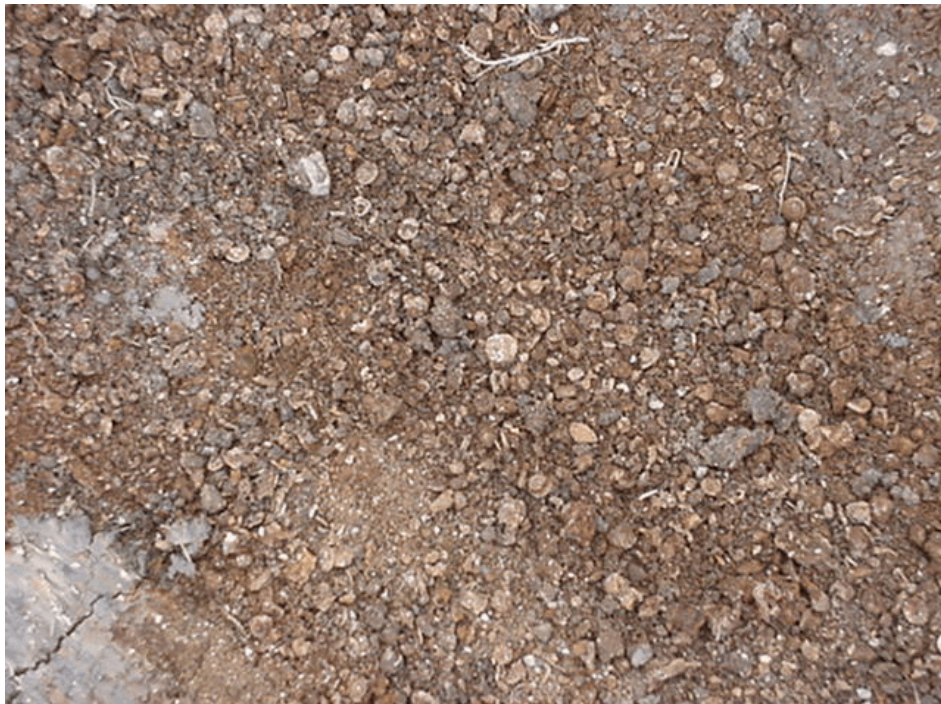
Figure 2-50. Photograph showing a closeup of the button ash underlying the clean soil stockpile. Photograph taken by Glenn May on August 26, 2004.
