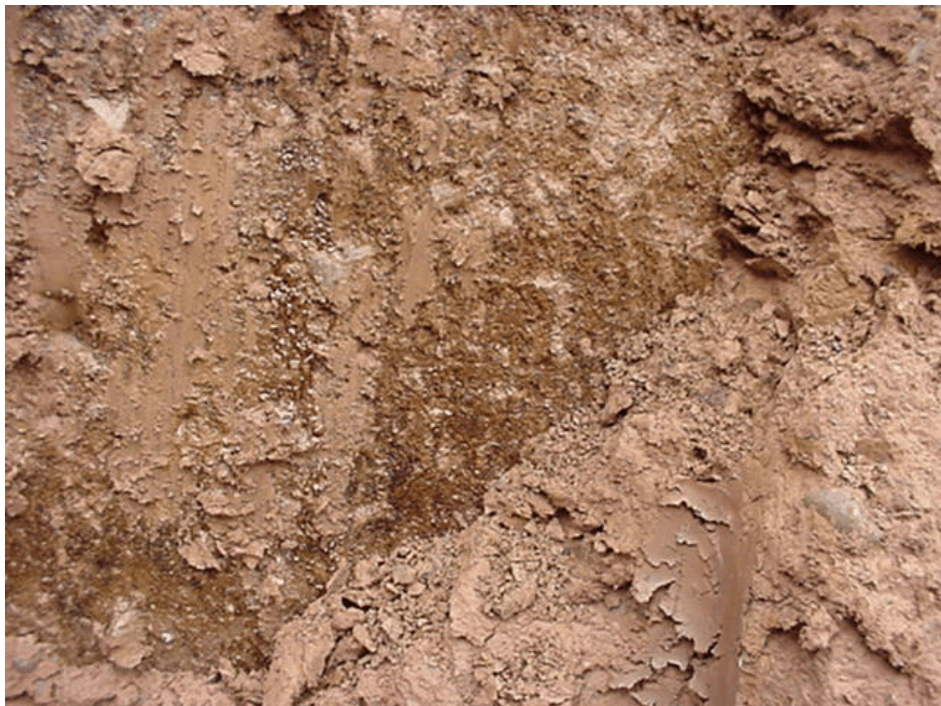
Figure 2-63. Photograph showing NAPL in a vertical dessication crack. View looking northeast. Photograph taken by Glenn May on October 21, 2004.
