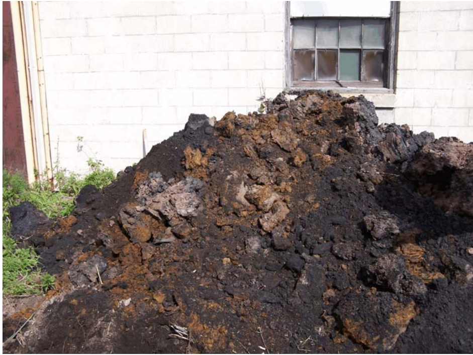
Figure 4-53. Photograph showing the grinding waste, ash and slag fill from the former ditch near the Boiler House. View looking northeast. Photograph taken by Glenn May on September 27, 2006.
