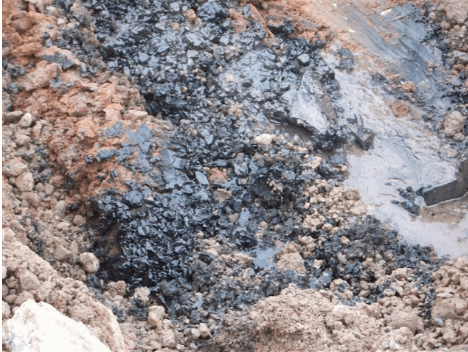
Figure 2-7. Photograph showing NAPL contaminated bedding along a floor drain under the Spauldite Sheet Basement. Photograph taken by Brian Hutzler on February 12, 2010.
