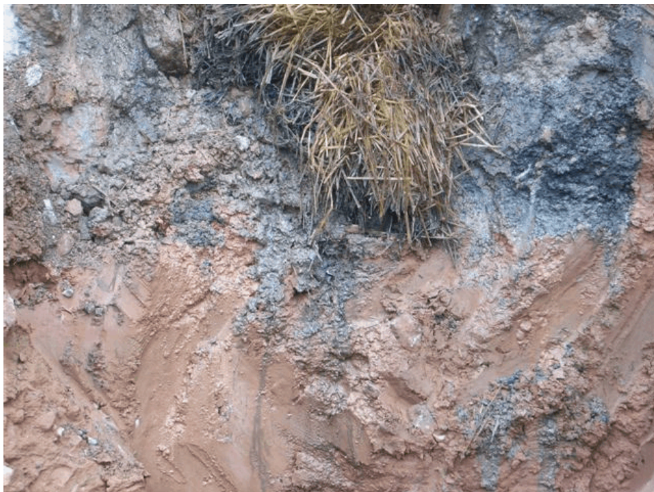
Figure 2-22. Photograph showing NAPL contaminated soil under the K-Line Storm Sewer where it exits the south foundation wall of the Saw Room. Photograph taken by Brian Hutzler on February 19, 2010.
