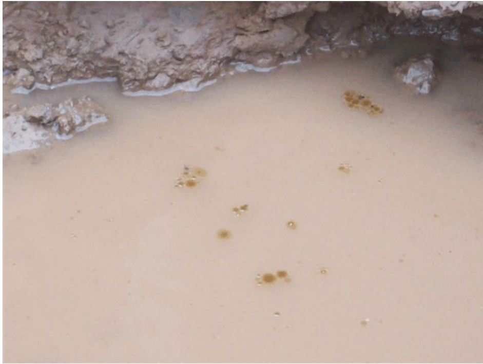
Figure 2-23. Photograph showing NAPL droplets on water in the K-Line Storm Sewer excavation. Photograph taken by Brian Hutzler on February 19, 2010.
