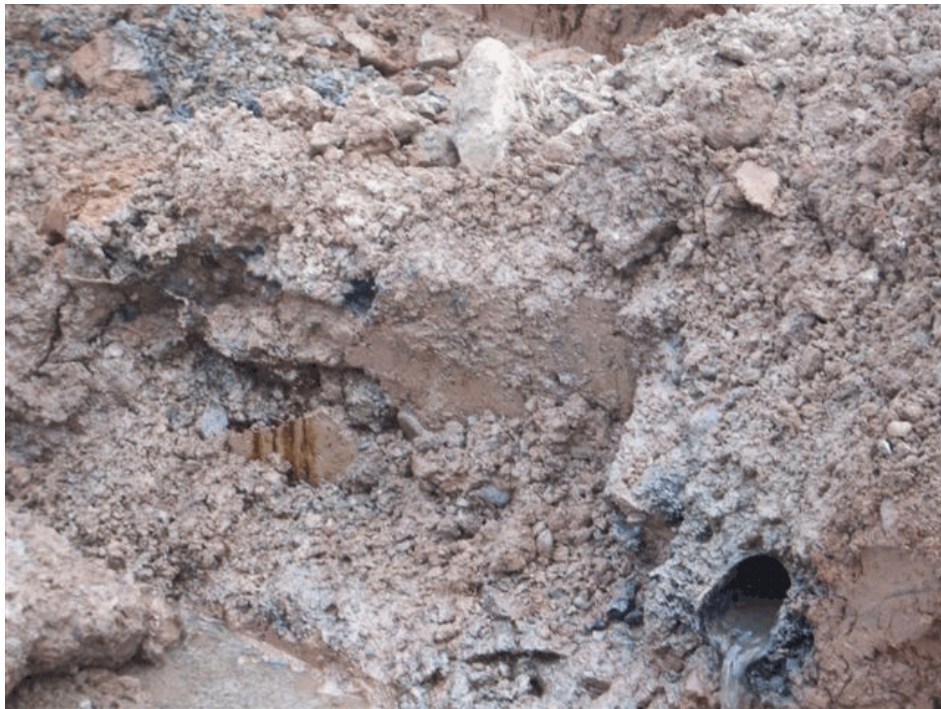
Figure 2-6. Photograph showing NAPL in the bedding along a floor drain under the Spauldite Sheet Basement. Photograph taken by Brian Hutzler on February 12, 2010.
