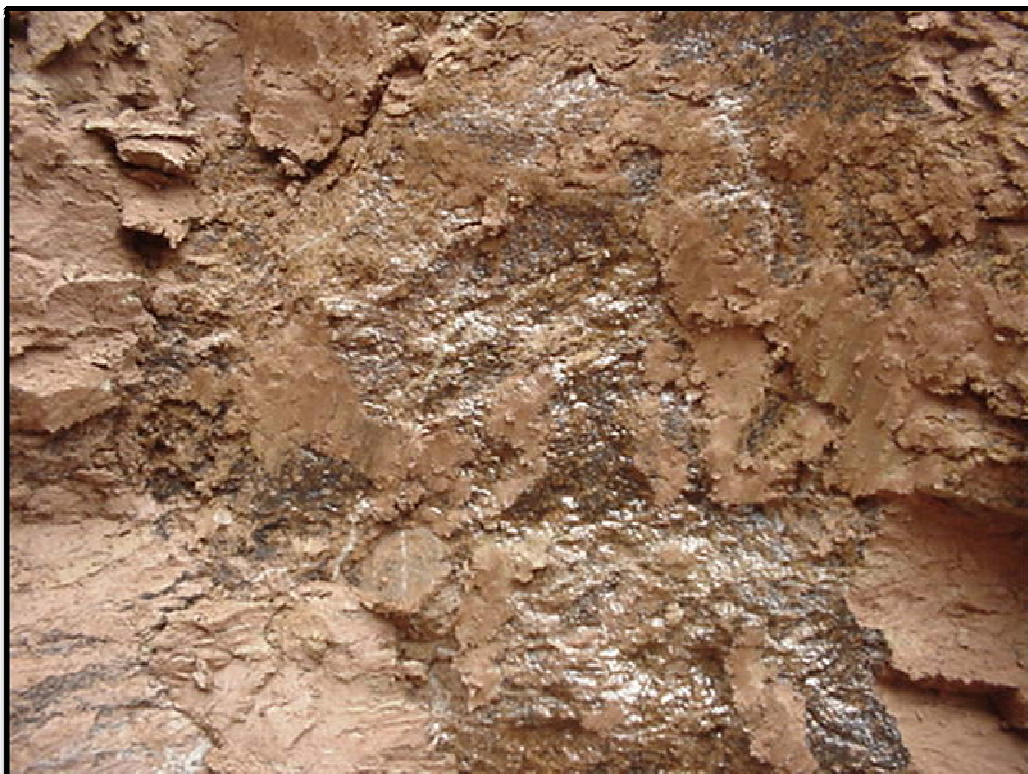
Figure 6-6. Photo showing the presence of NAPL along a vertical desiccation crack in the native silty clay soils that underlie the Spaulding Composites Site.
