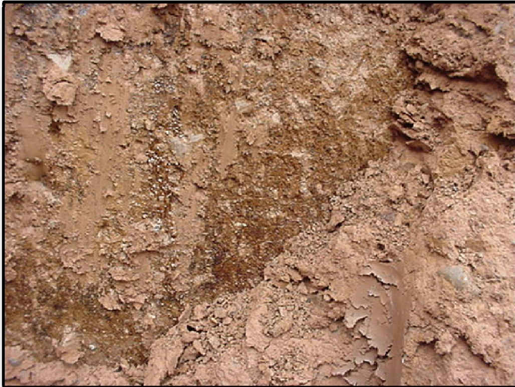
Figure 6-5. Photo showing the presence of NAPL along a vertical desiccation crack in the native silty clay soils that underlie the Spaulding Composites Site.
