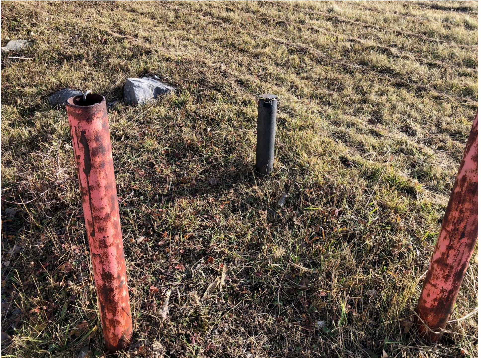
View of the stick-up, steel, protective casing and cover for groundwater monitoring well GW-4, and protective bollards, facing south.
