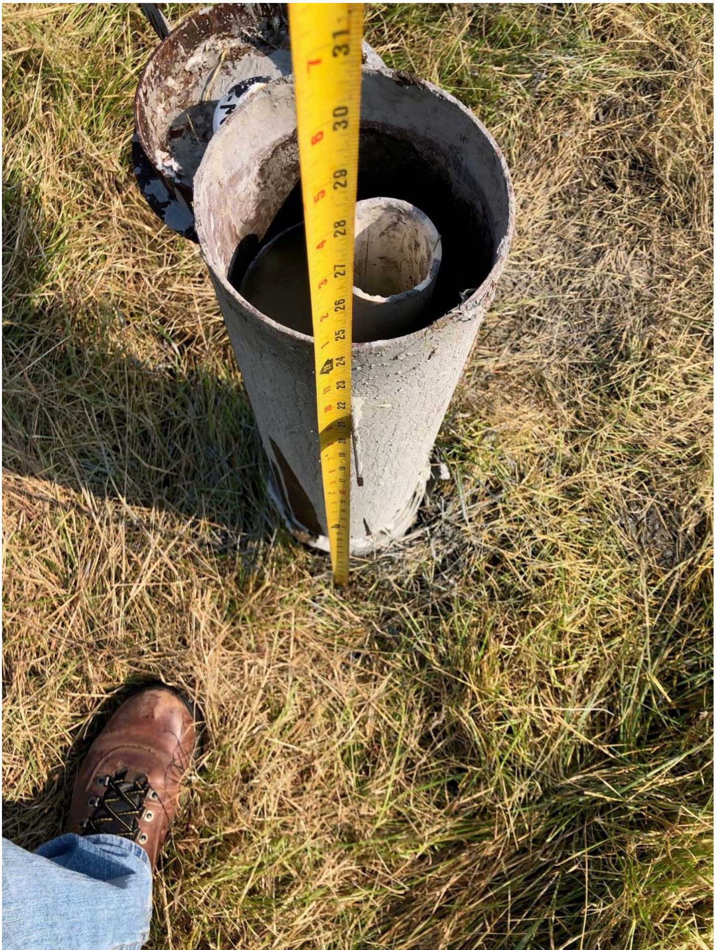
View showing the height (above ground surface) of the protective steel casing surrounding monitoring well GW-2.
