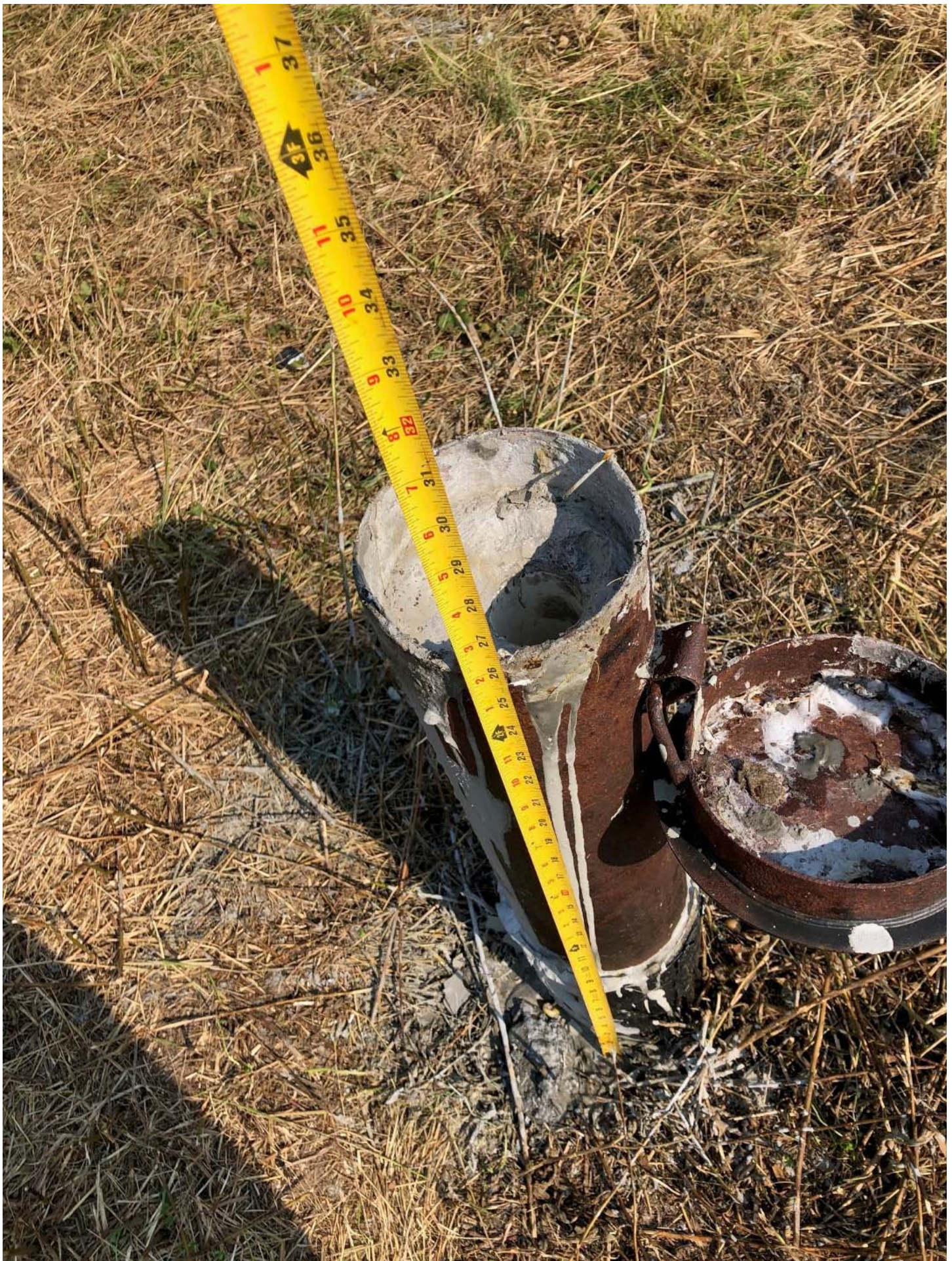
View showing the height (above ground surface) of the protective steel casing surrounding monitoring well GW-5.
