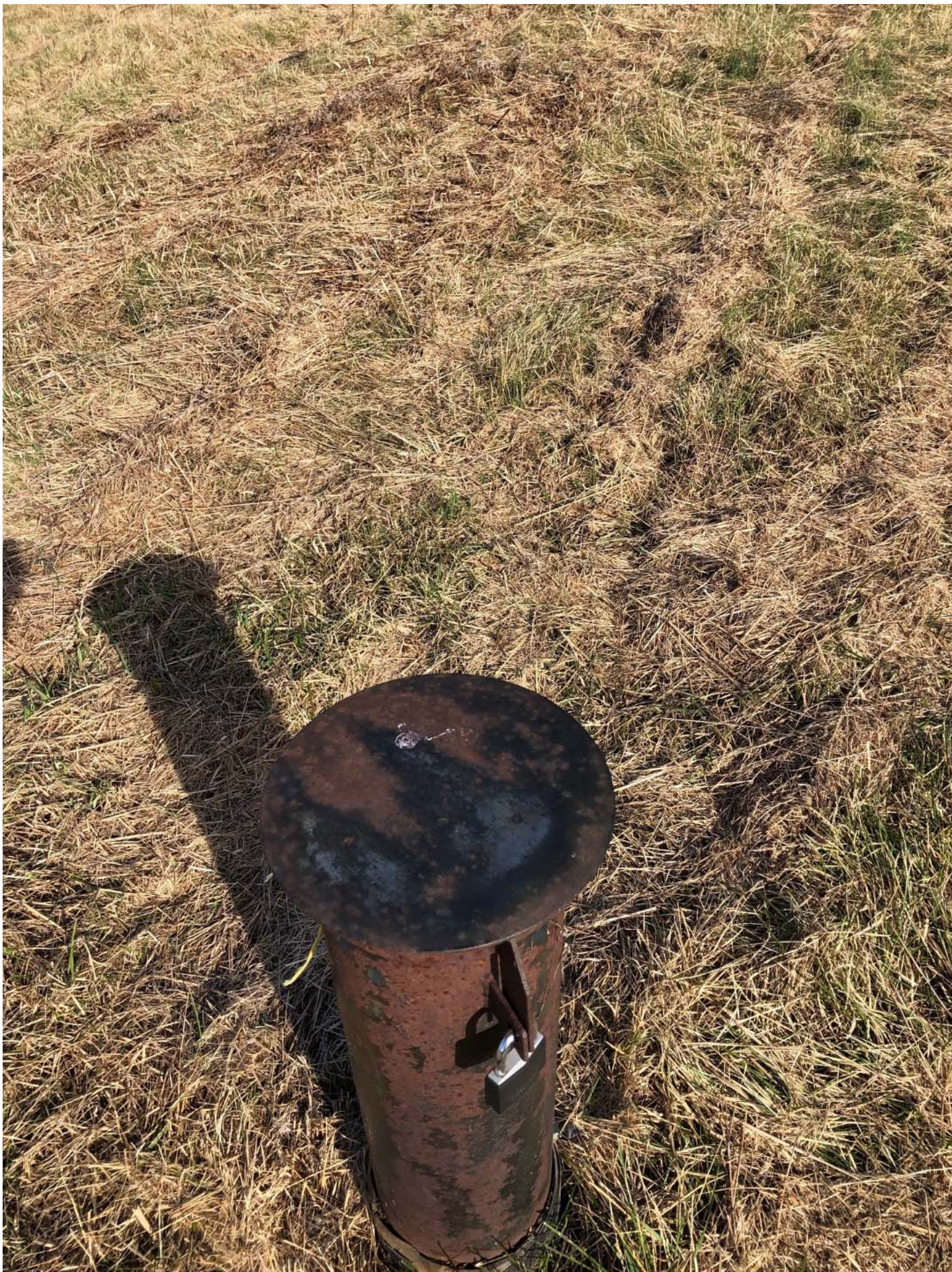
View of the stick-up, steel, protective casing and cover for groundwater monitoring well GW-2, facing southeast.
