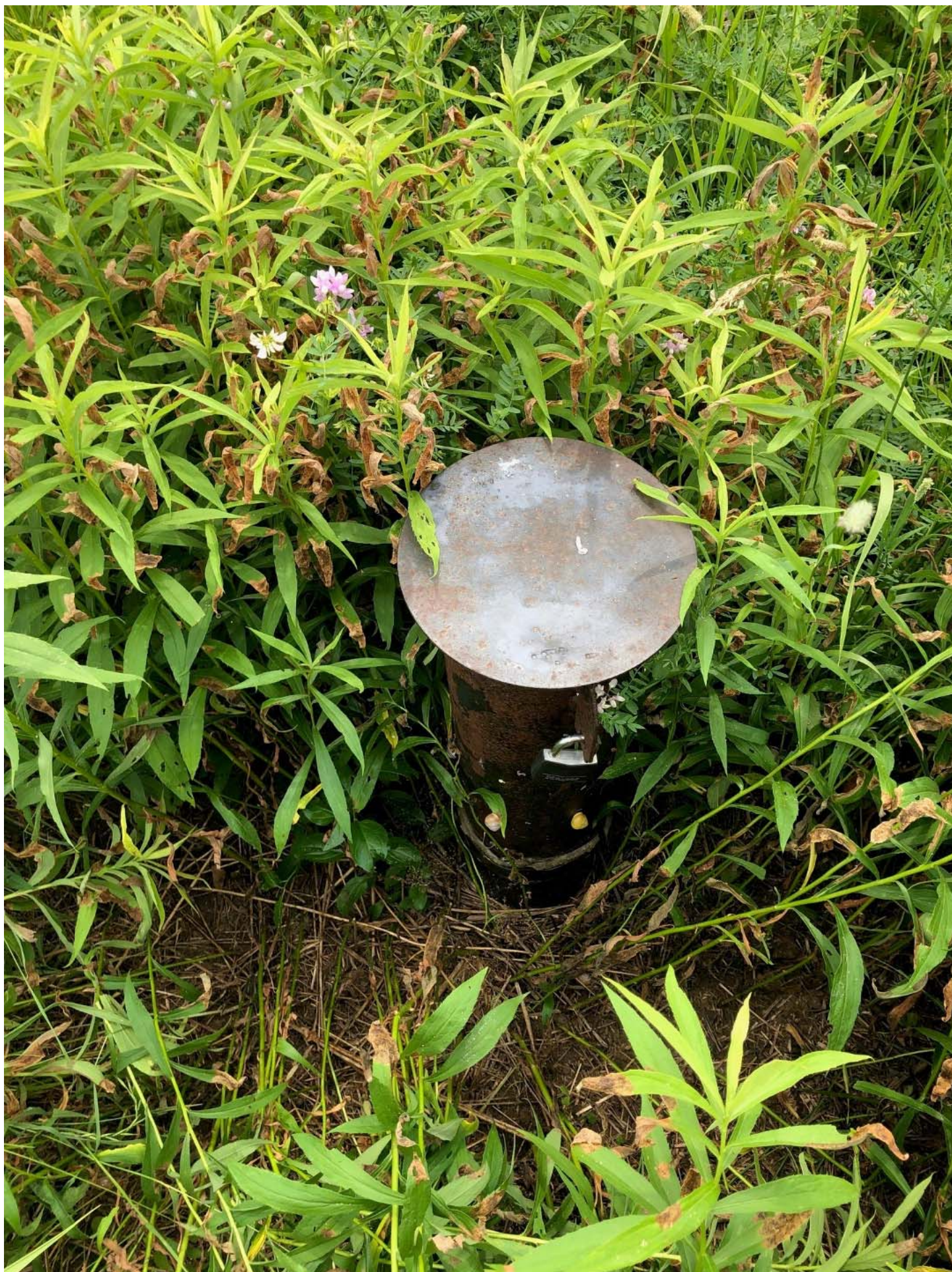
View of the stick-up, steel, protective casing and cover for groundwater monitoring well GW-5.
