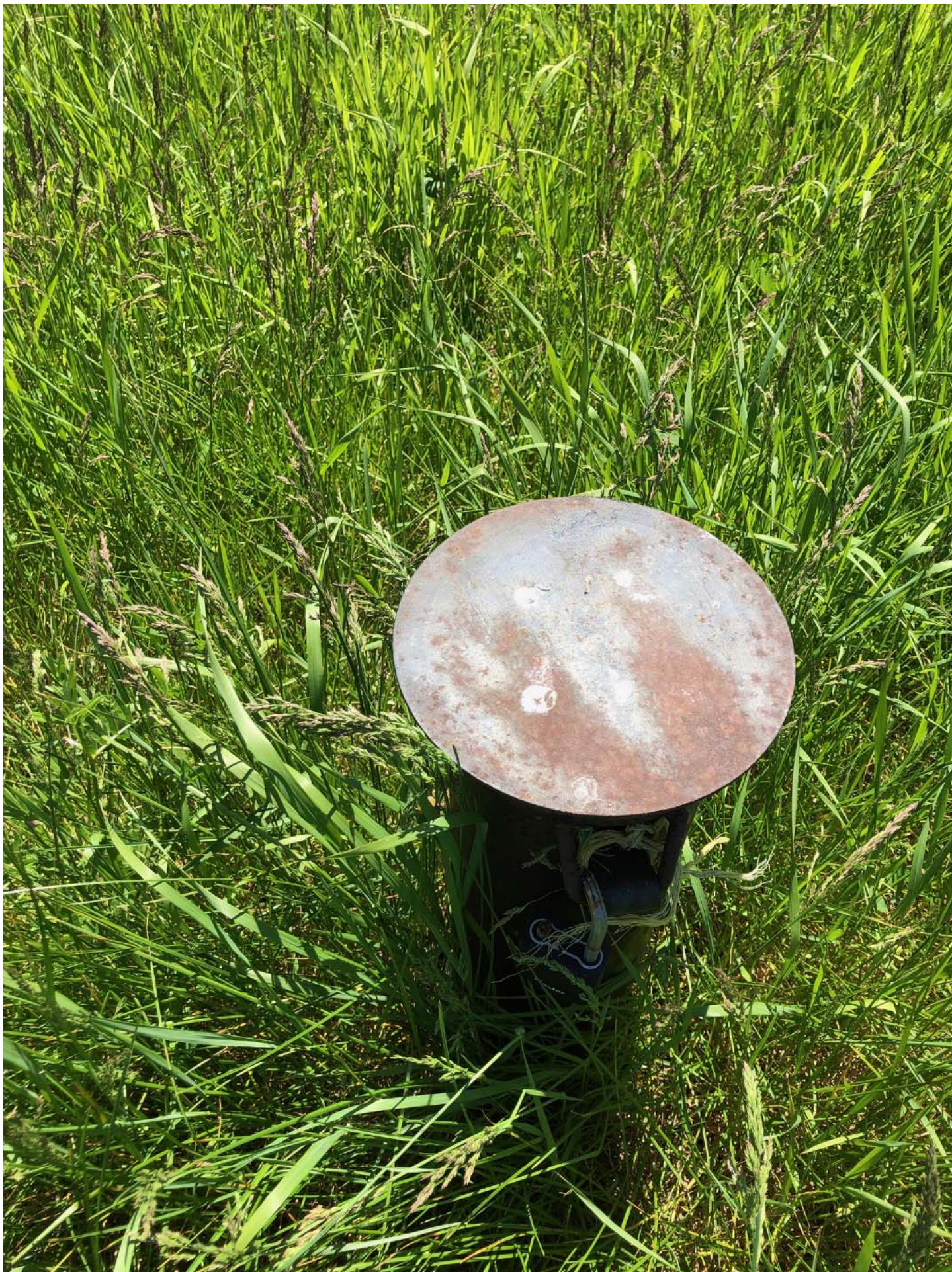
View of the stick-up, steel, protective casing and cover for groundwater monitoring well GW-2, facing northwest.
