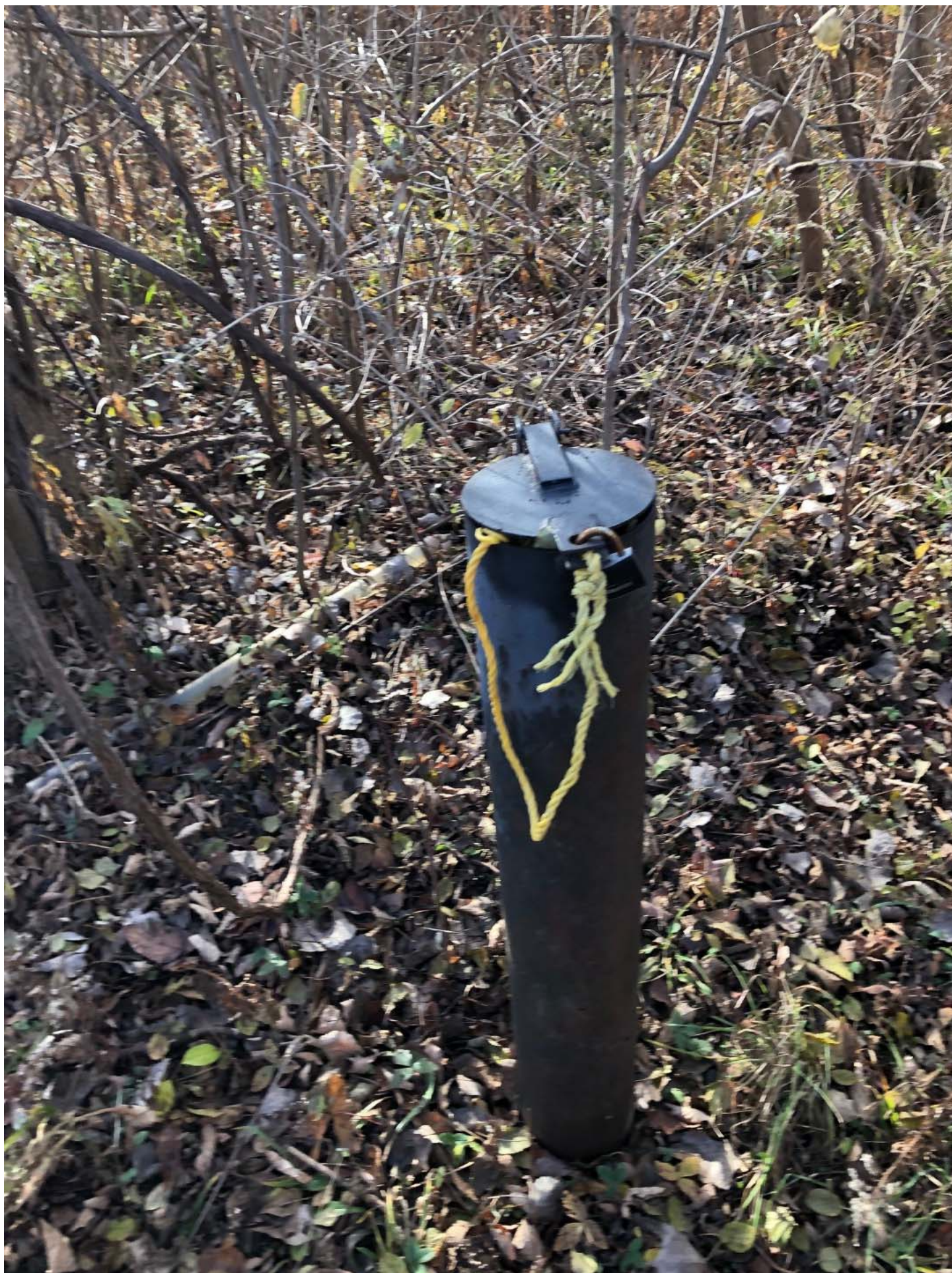
View of the stick-up, steel, protective casing and cover for groundwater monitoring well GW-1, facing southwest.
