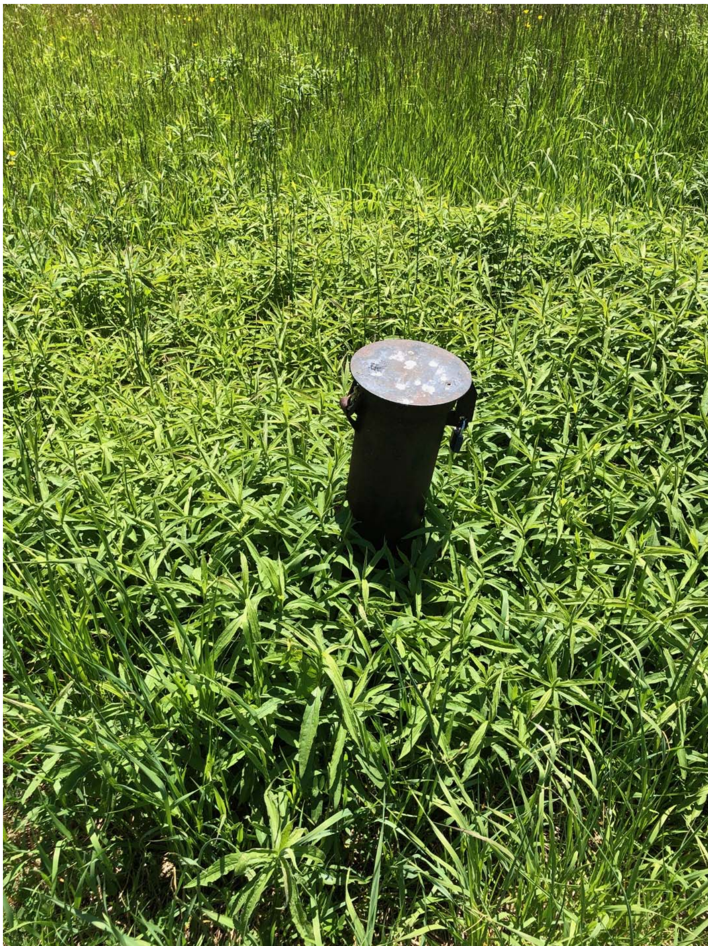
View of the stick-up, steel, protective casing and cover for groundwater monitoring well GW-5, facing north.
