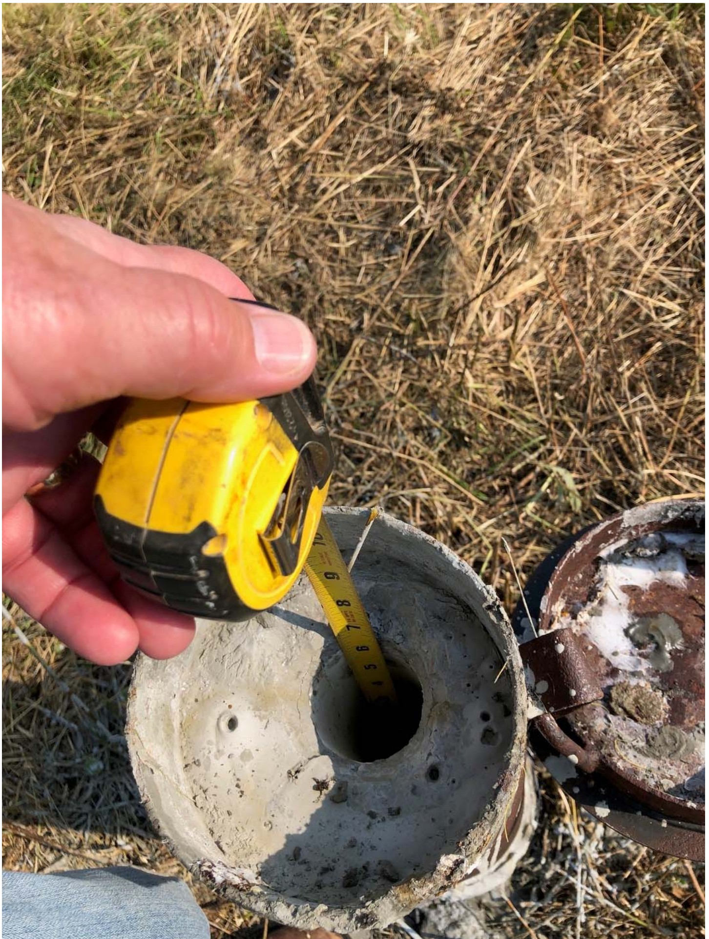
View showing the depth (below the top of PVC casing) to the top of the grout, tremmied into monitoring well GW-5, following monitoring well decommissioning activities.
