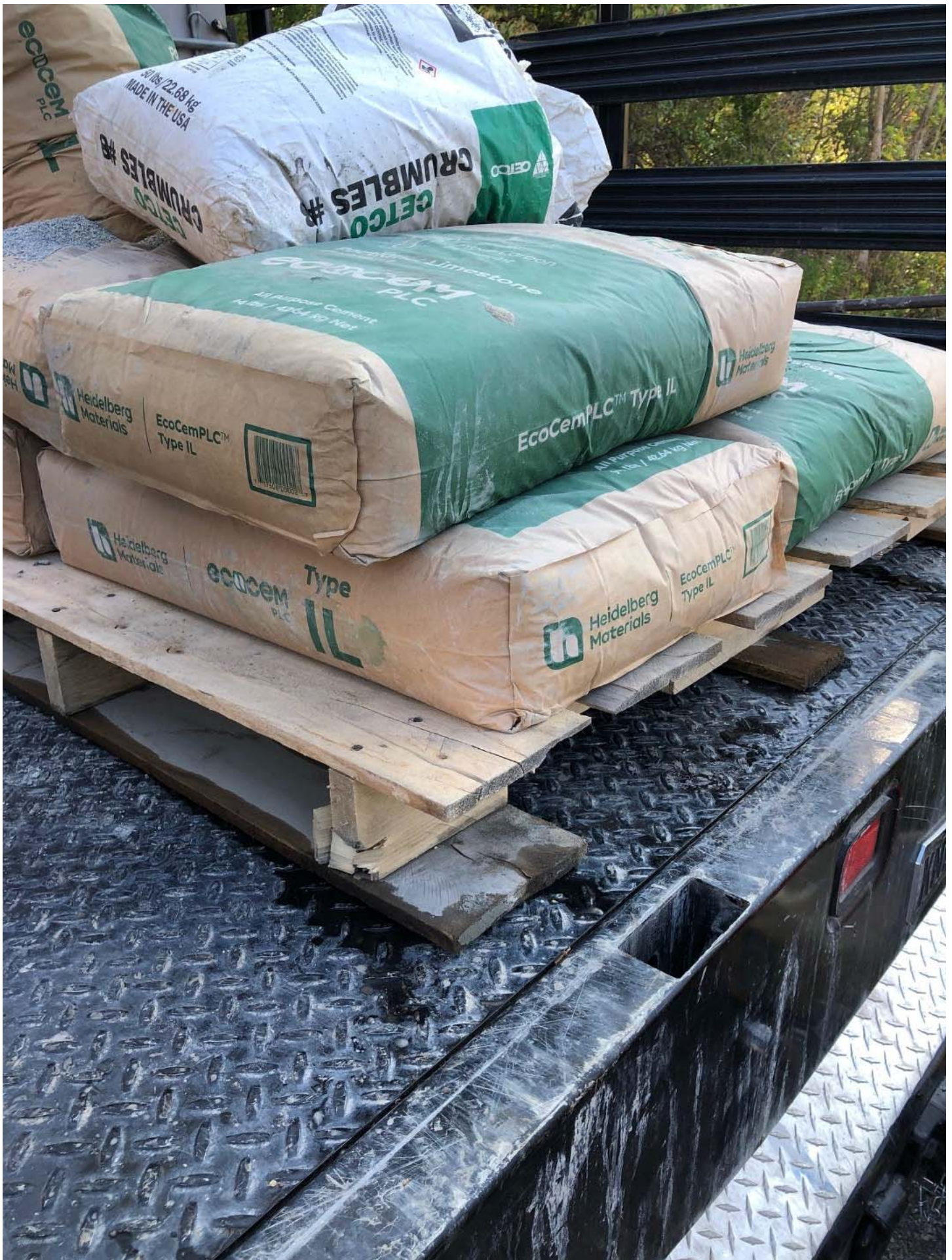
Close-up view of the portland cement and bentonite materials used to tremie grout (decommission) each well screen/casing.
