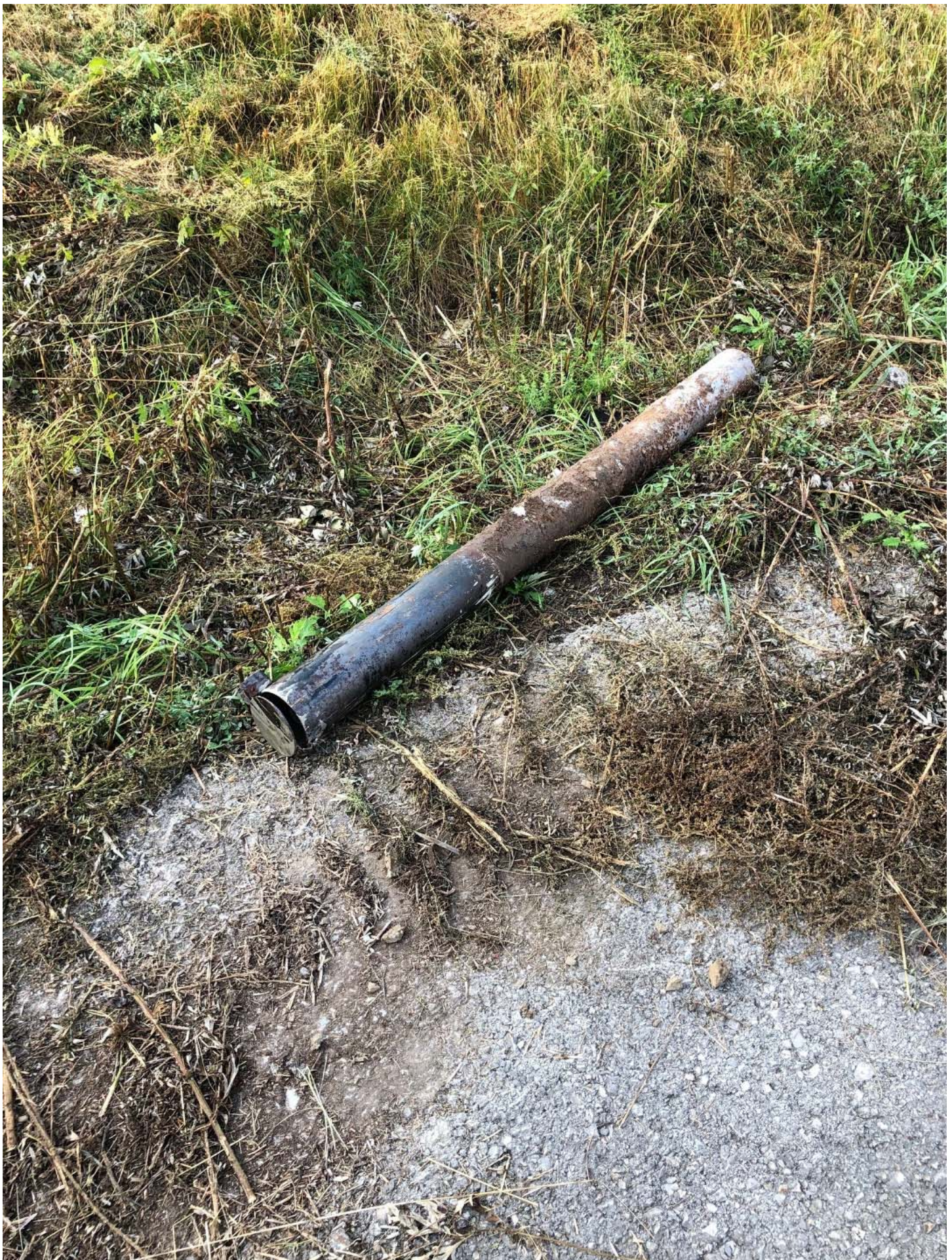
View of the monitoring well GW-4 protective steel casing that was removed from the ground following monitoring well decommissioning.
