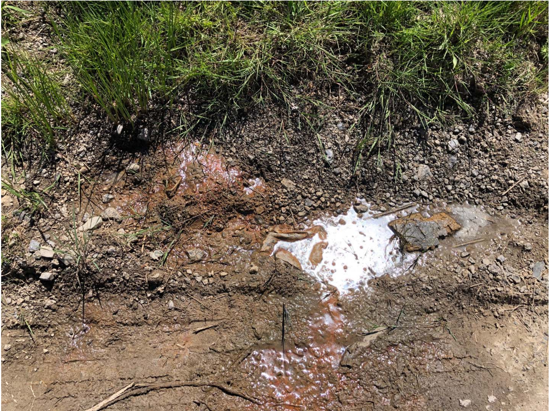
Close-up view of second area of water seepage, and the rust-colored precipitate evident in the standing water.
