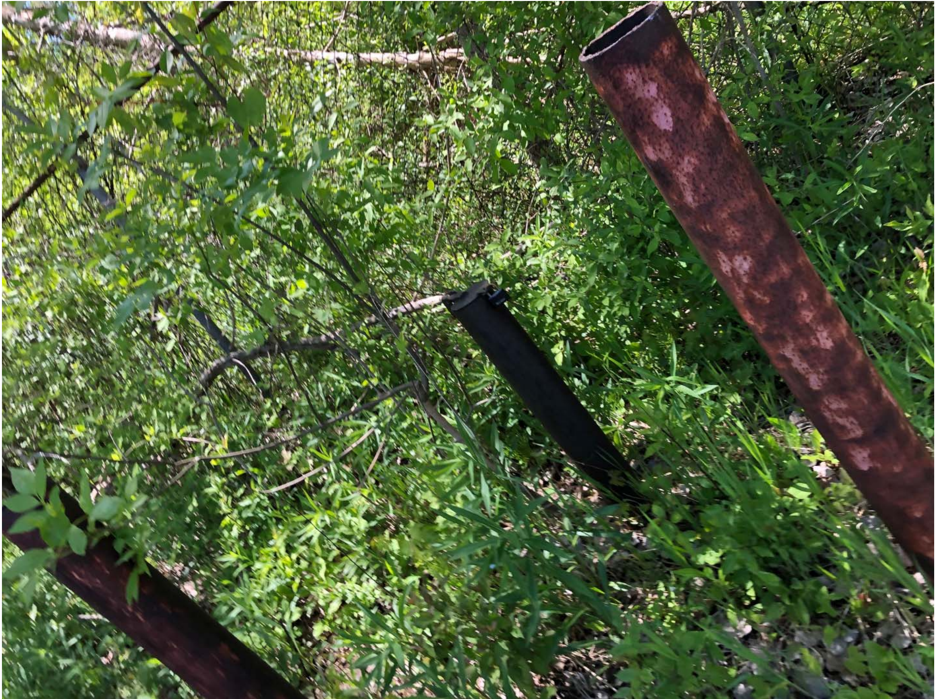
View of the stick-up, steel, protective casing and cover for groundwater monitoring well GW-3, and protective bollards, facing west.
