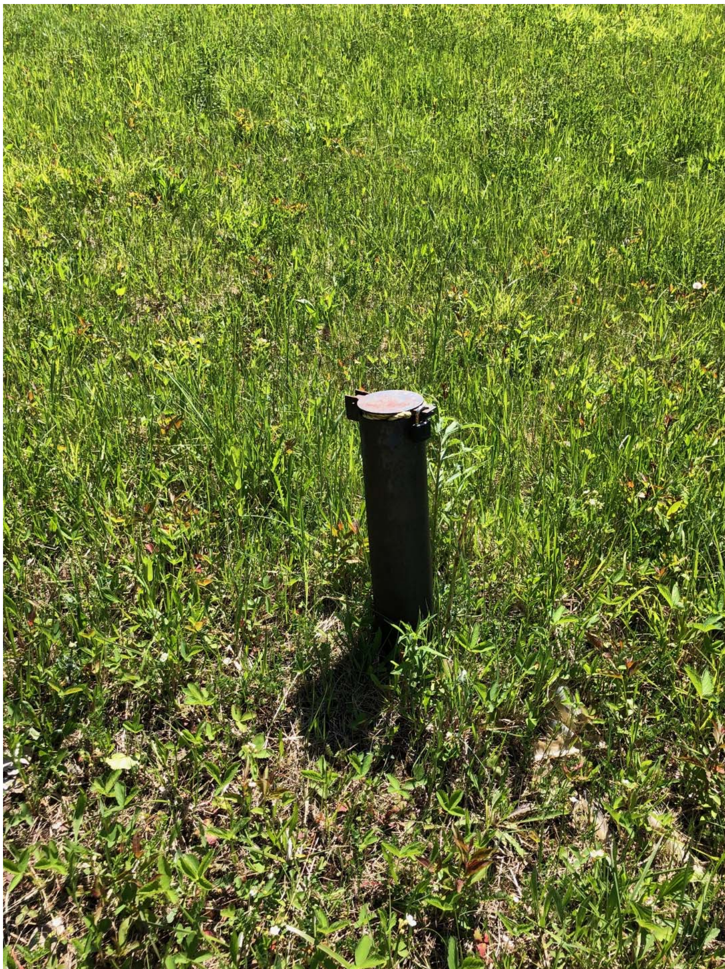
View of the stick-up, steel, protective casing and cover for groundwater monitoring well GW-4, facing southwest.
