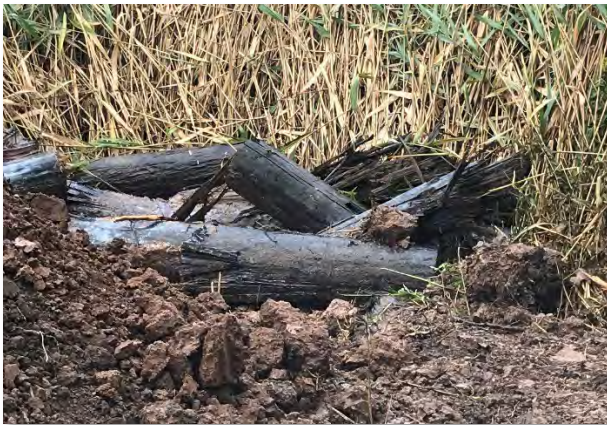
Potentially creosote-treated wood poles pulled from TP-04-2020.
