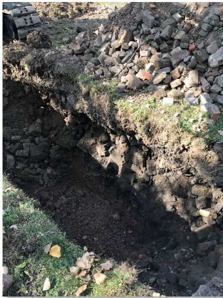
Silt, clay, coke fragments, brick, and concrete at TP-03-2020.
