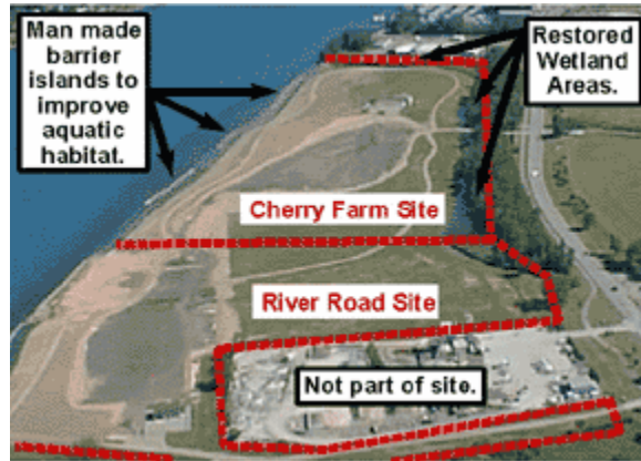
Figure 2. Remedial action construction was completed in September 1999. Operations, maintenance, and monitoring activities are ongoing, including O&M of the ground water extraction and treatment system.
