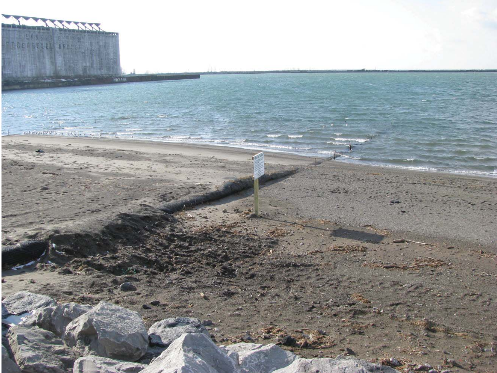
Gallagher Beach Photo 6: Look southwest at test area. Note apparent burial of edge restraint near waterline.
