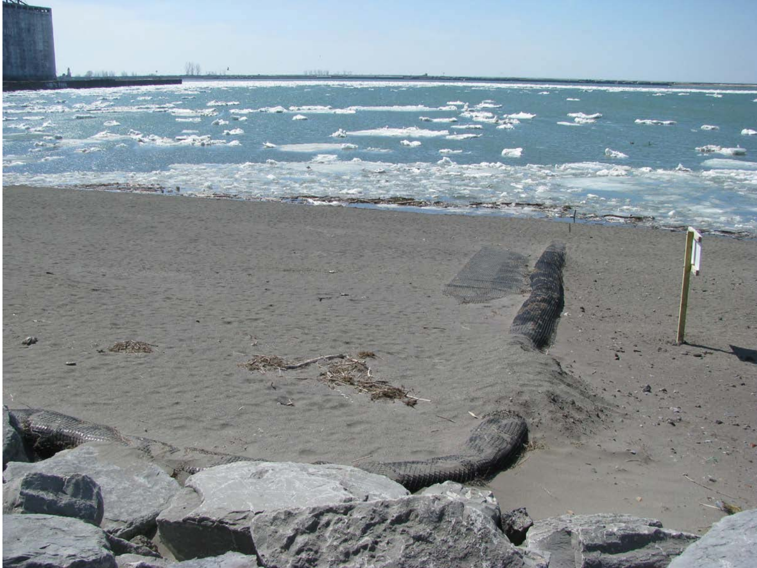
Gallagher Beach Photo 2: Looking west along north edge of test area. Note man-placed mound of sand over the edge restraint, and the exposed lock-down netting. The sand inside the test area there is “higher” than the sand outside.
