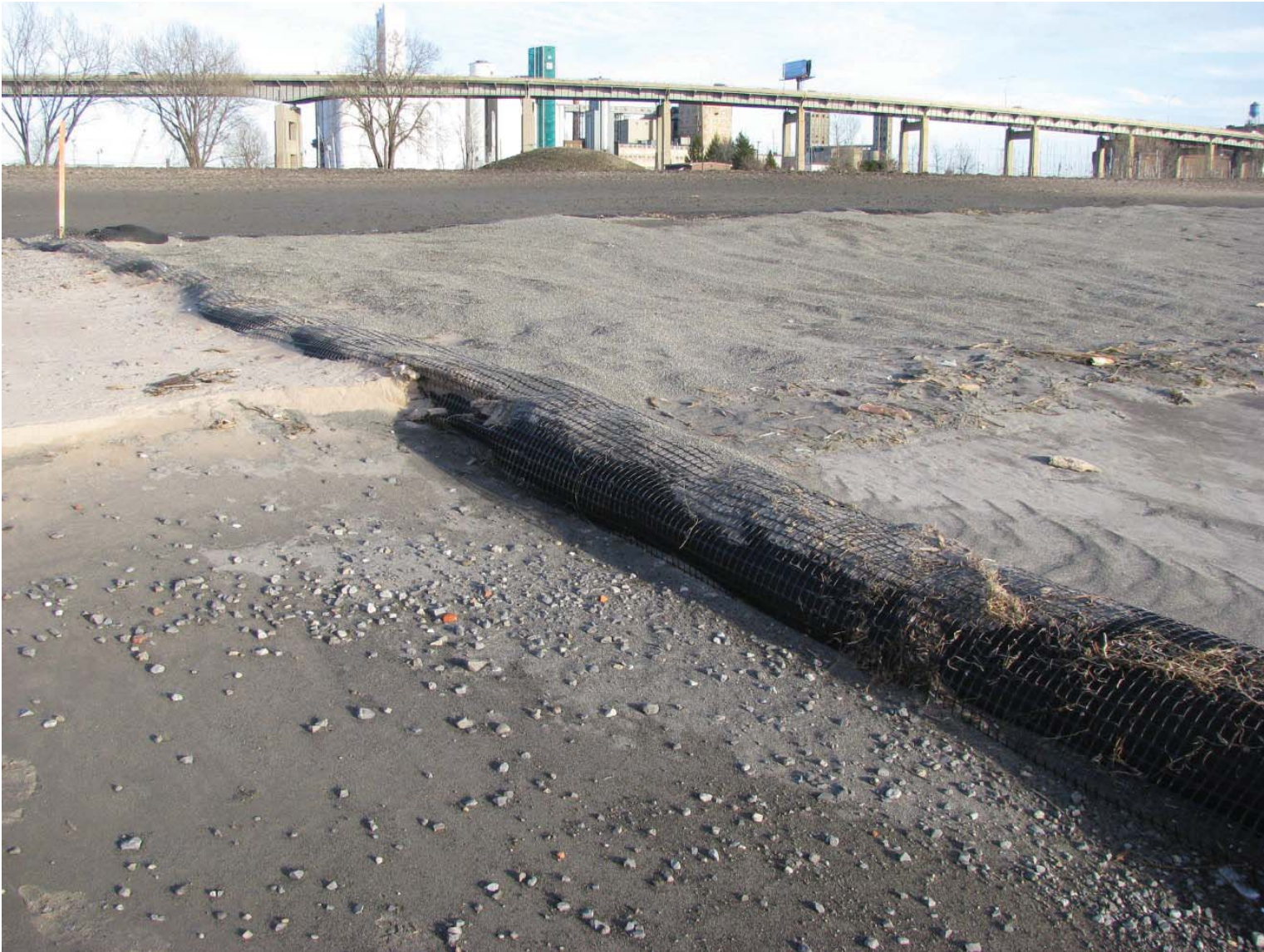
NYPA Parcel Photo 2: Look southeast at the northern edge of the test area. Note the drift line and material segregation within the test area. The scarp outside of the test area (photo left) is evidently how that sand was placed (per ECHDC).
