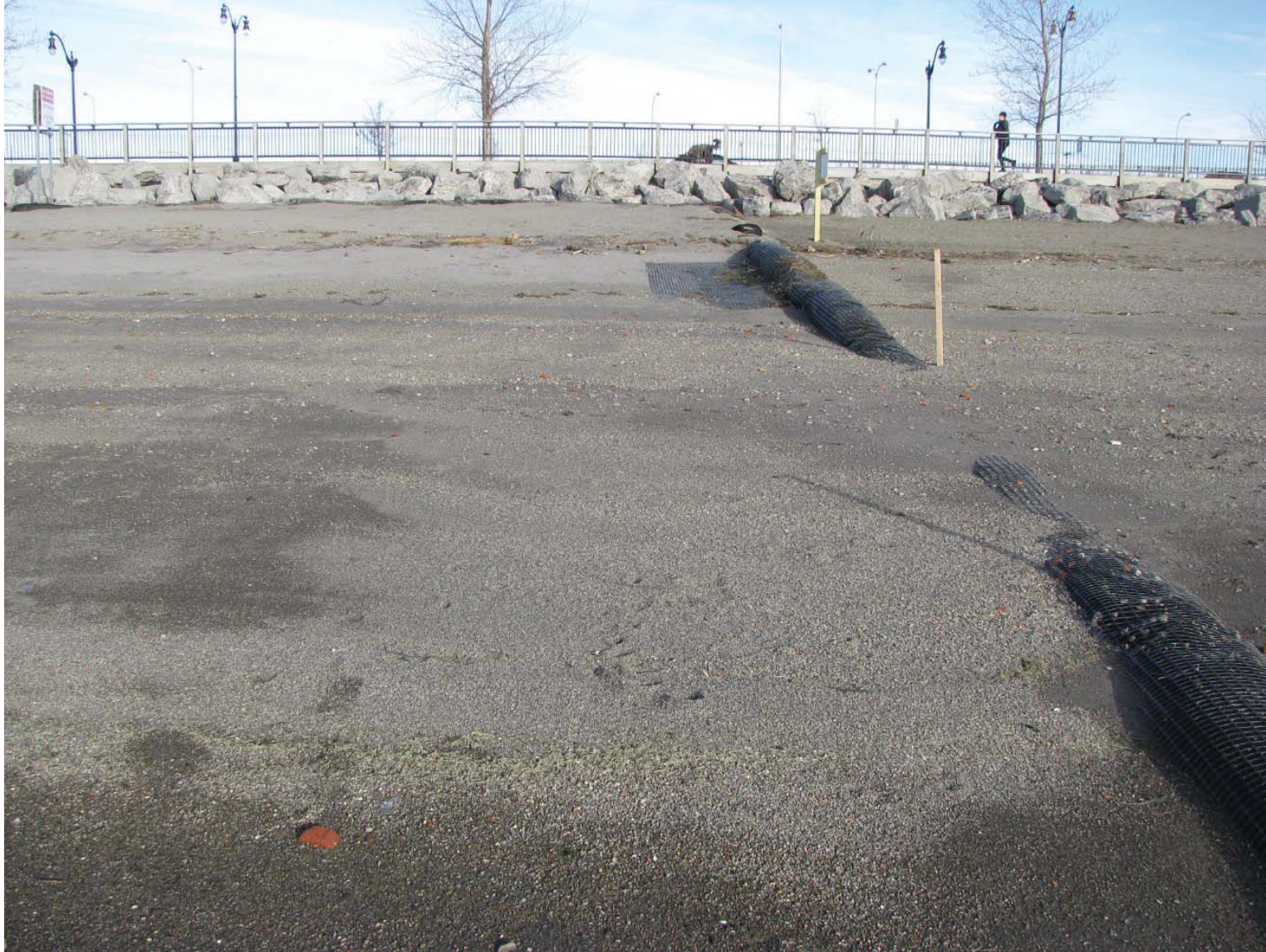
Gallagher Beach Photo 2: Look east at the south upper corner of the test area. Note the downslope movement of sand and the segregation by grain size. Note also drift line and exposed lock-down netting at the top of the eroded area.
