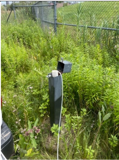
Typical groundwater monitoring well
