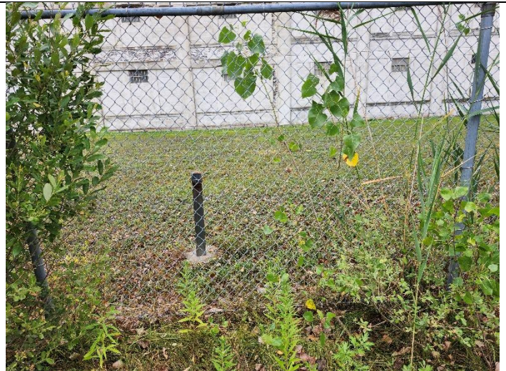
Typical Monitoring Well
