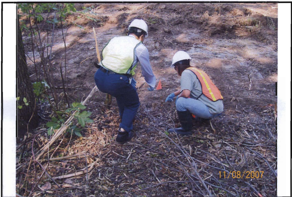
Photograph 4. Post-excavation soil sampling conducted by ERM with split samples taken by USEPA's REAC representative.
