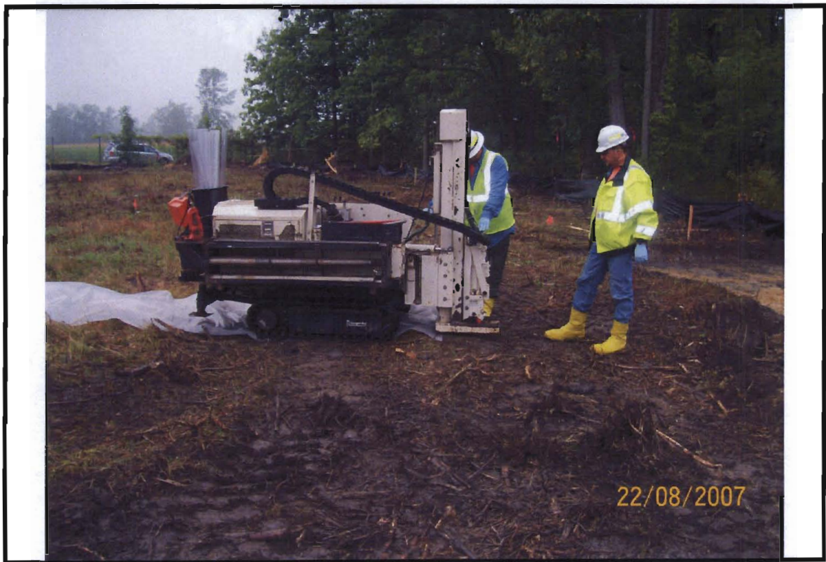
Photograph 11. PCB sampling via Geoprobe.
