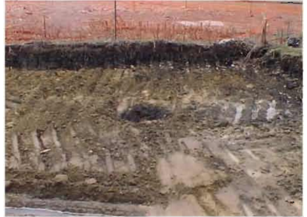
Figure 2 PCB Hotspot Number 4, May 15, 1997 (Note the dark spot in center of picture. Spot suspected to be PCB oil.)
