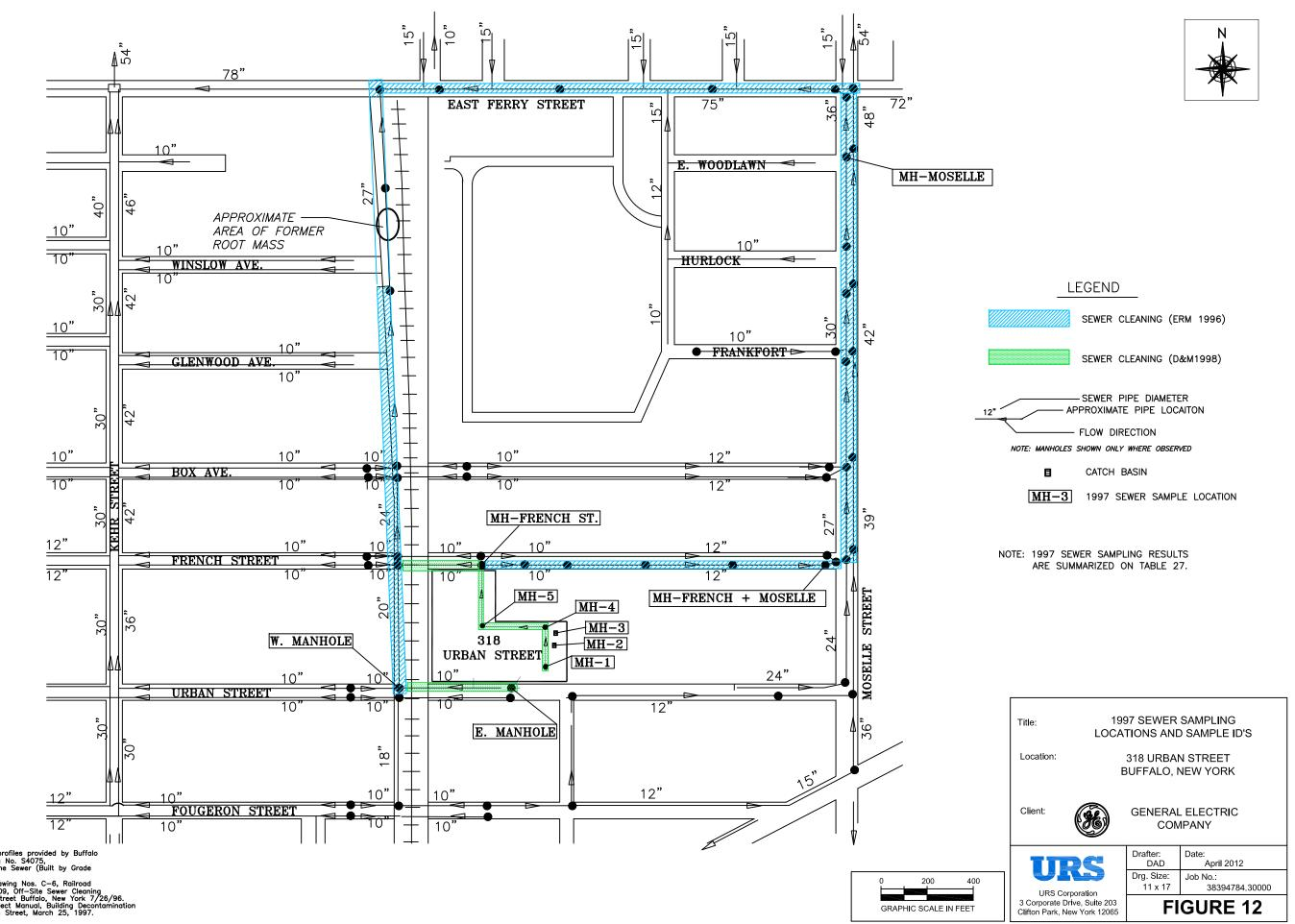
Adapted from sewer maps and profiles provided by Buffalo Sewer Authority including Drawing No. 54075, New York Central R.R. – Belt Line Sewer (Built by Grade Crossing Commission – 1910). Adapted from ERM-Northeast Drawing Nos. C-6, Railroad Sewer Pian 3/30/97, and CL-009, Off-Site Sewer Cleaning Location Vicinity of 318 Urban Street Buffalo, New York 7/26/96. Both drawings are from the Project Manual, Building Decontaminatic and Soil Remediation, 318 Urban Street, March 25, 1997.
