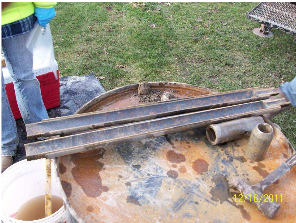
Figure 6: View of split spoon core 6'-8' bgs at EE-3 (No Recovery)
