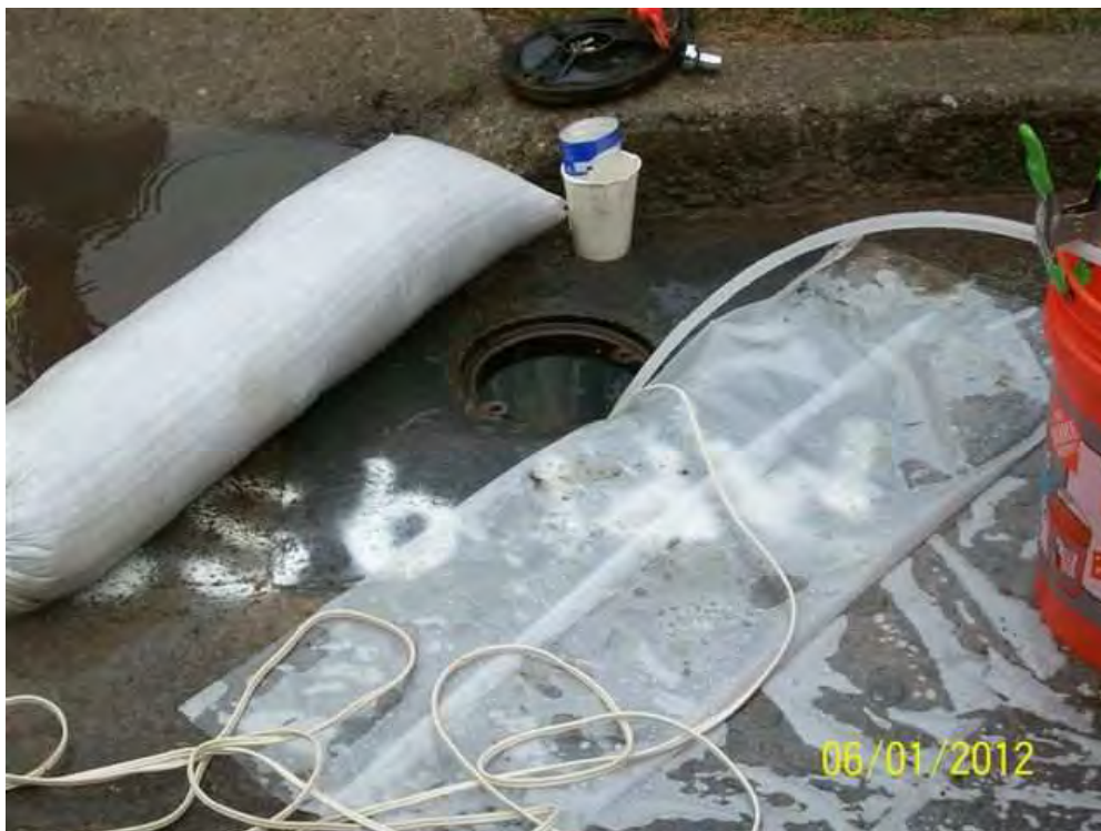
Figure 7: View of development of well MPI-9S-R, well bailed continuously with cups during development (Looking N)
