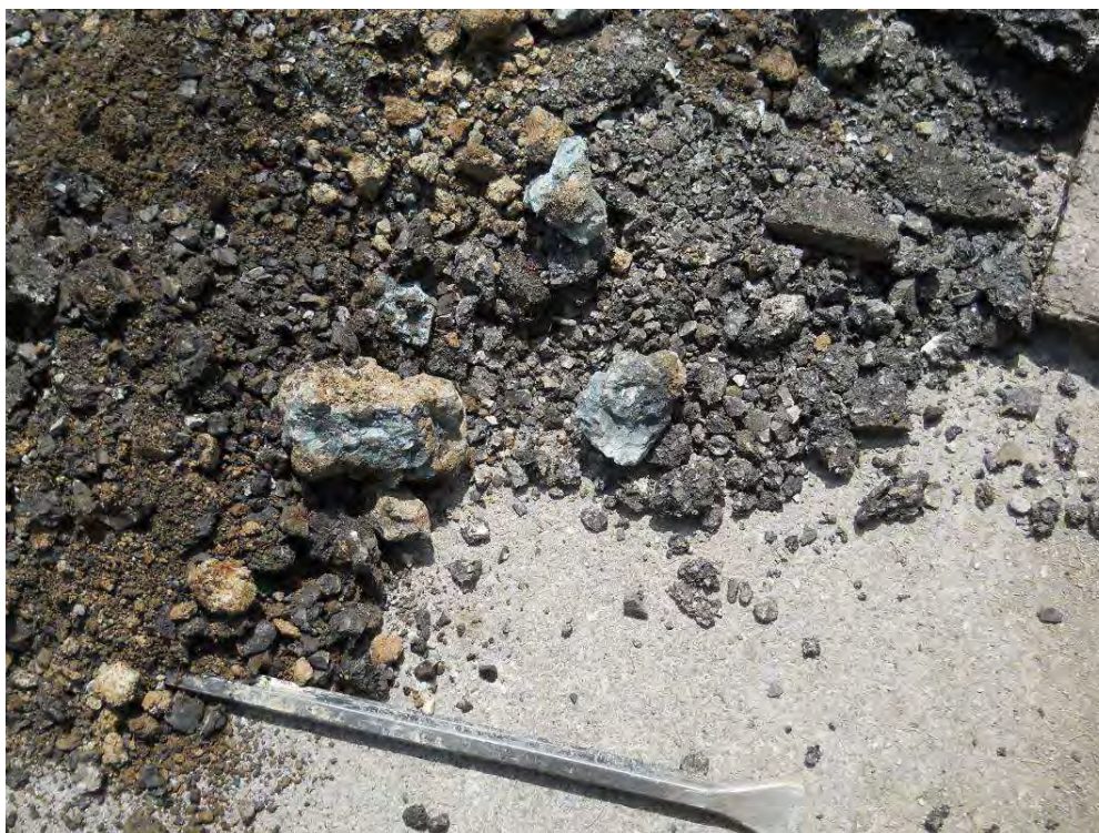
Figure 6: View of slag that was pulled out of borehole ESI-5-R (Looking down, PM)
