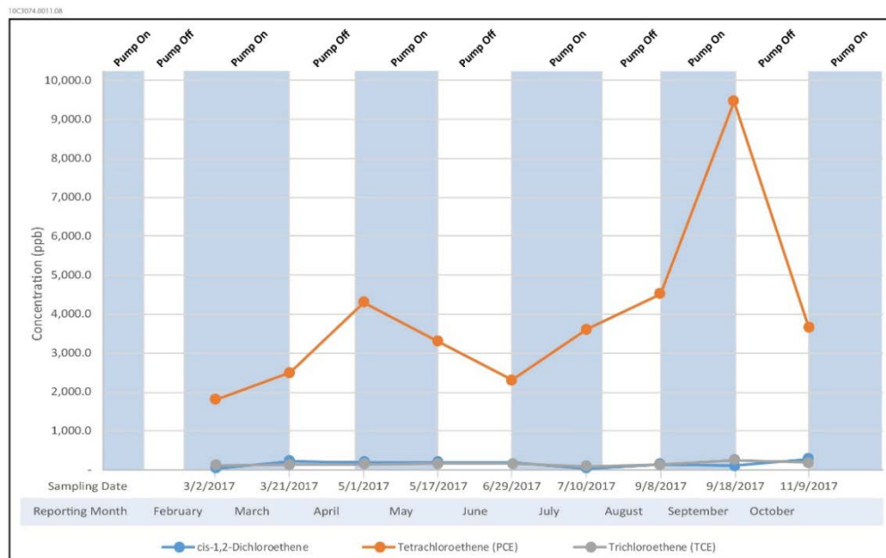
Figure 3-6 2017 Pulsed-Pumping Program Groundwater Sampling Results for Groundwater Pumping Well PW-6
