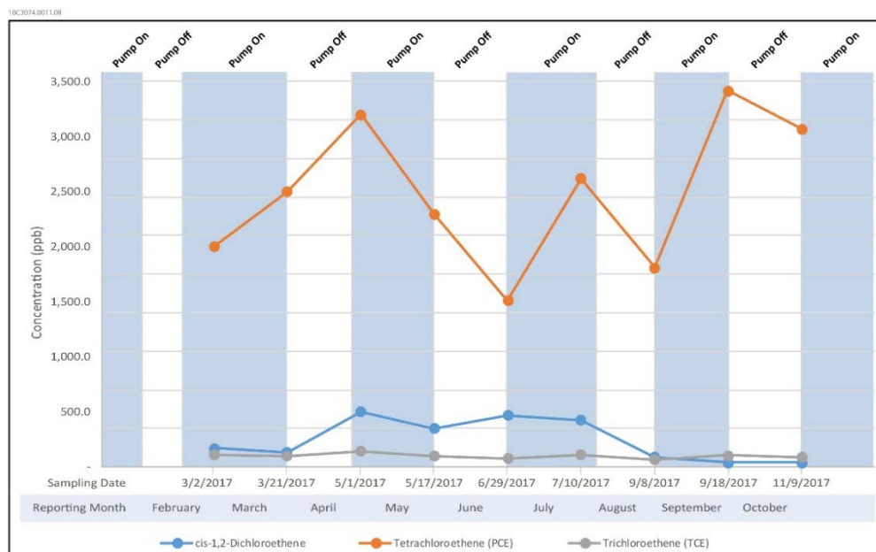
Figure 3-5 2017 Pulsed-Pumping Program Groundwater Sampling Results for Groundwater Pumping Well PW-5
