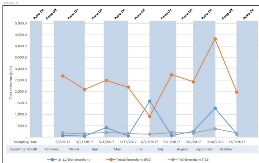
Figure 3-4 2017 Pulsed-Pumping Program Groundwater Sampling Results for Groundwater Pumping Well PW-4
