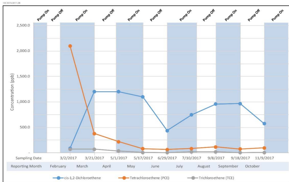
Figure 3-8 2017 Pulsed-Pumping Program Groundwater Sampling Results for Groundwater Pumping Well PW-8
