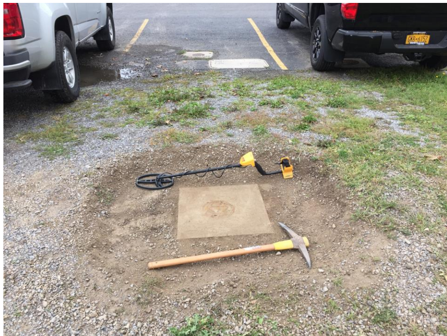
PIEZOMETER PZ-7D WAS LOCATED UNDER STONE/GRAVEL IN PARKING LOT.
