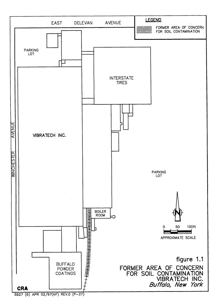
Vibratech retained CRA to prepare a plan for remediation of the contaminated soil. The remedial technology selected was on-Site treatment using ex situ soil vapor extraction (ESVE). The system design is presented in the report entitled "Soil Vapor Extraction Work Plan, Vibratech, Inc., Buffalo, New York", May 1995, prepared by CRA. This report was approved by the New York State Department of Environmental Conservation (NYSDEC).
