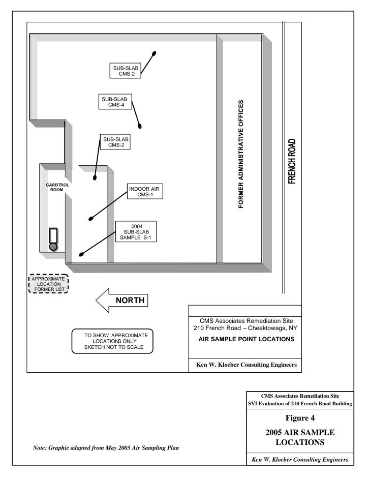
The highest sub-slab VOCs were observed at sample locations 189-S1, CMS-3, and CMS-2 (see *Figure 4*.) Sample CMS-4 exhibited lower VOCs, yet it was virtually mid-point between two of the highest readings. That indicated a potential discontinuity of the sub-slab media, or something present to block the free movement of the vapor.
