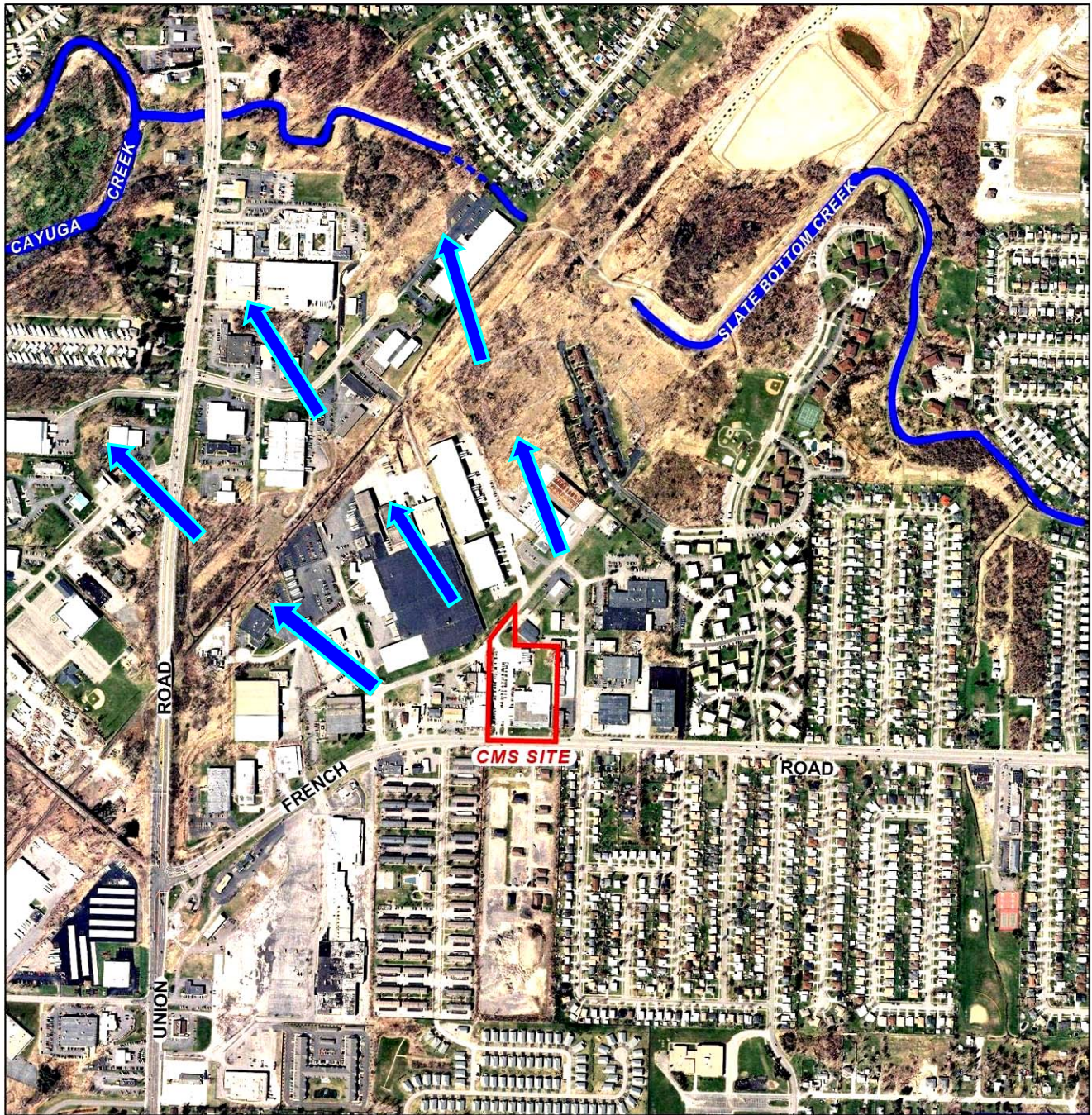
Figure 1. Aerial photograph showing the location of the CMS site relative to Cayuga Creek and Slate Bottom Creek. Blue arrows represent generalized groundwater flow directions inferred from topography and assuming both creeks are perennial streams that are continuously gaining groundwater discharge.
