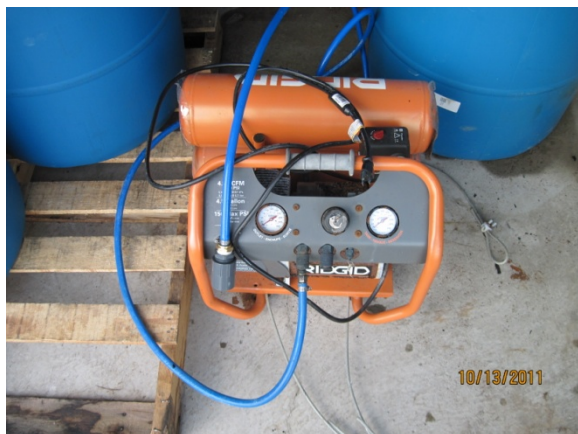
Air compressor setup used to purge remaining water from system piping.
