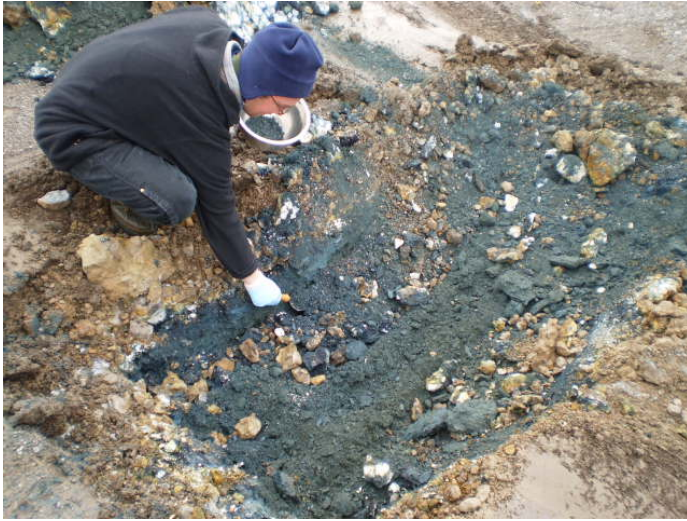
TP-6 profile: mostly MGP purifier waste (decomposed wood chips)
