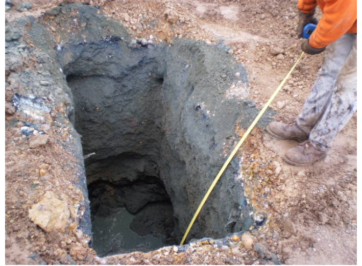
TP-6 profile: mostly MGP purifier waste (decomposed wood chips)
