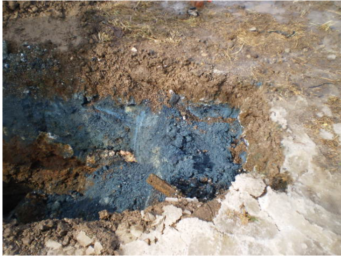
TP- 7 profile: layer of MGP purifier waste followed by rocky, cemented slag
