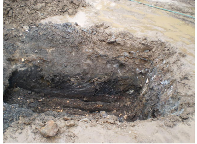
TP-4: mostly rocky slag fill, with cemented layers, unable to penetrate bottom layer
