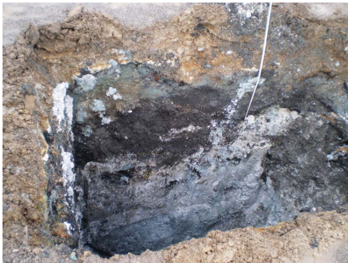
TP-1 profile: Upper layer contains slag/foundry sand like fill followed by a lime waste fill stained by MGP purifier waste
