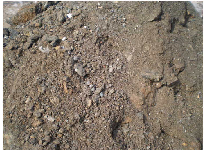
Mostly rocky slag fill spoils, with cemented layers, unable to penetrate bottom layer
