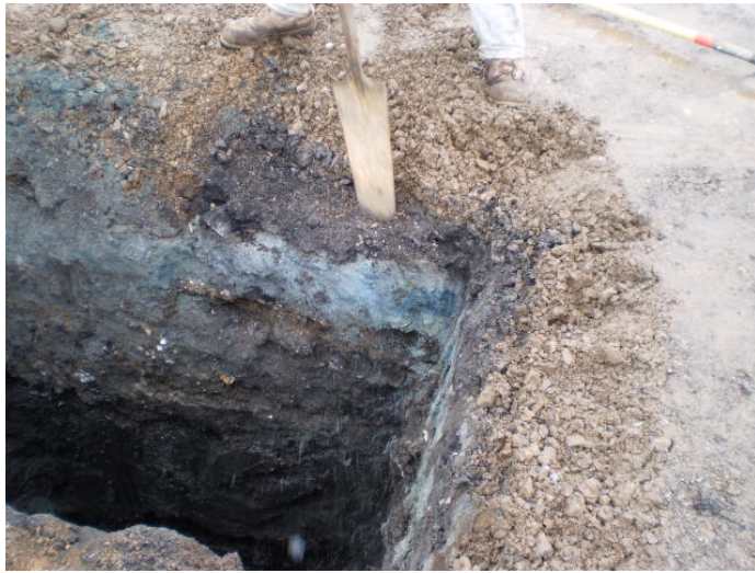
TP- 2 profile: Fine slag/foundry sand layer followed by and MGP purifier waste layer, followed by a rocky slag layer
