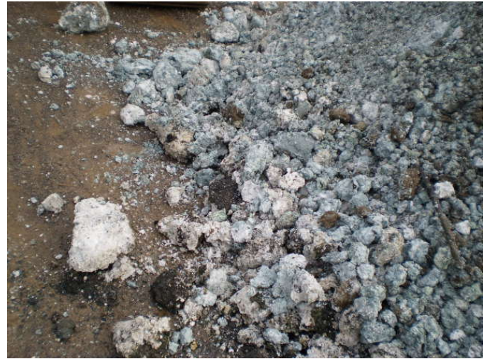
Lime waste fill, some blue staining from MGP purifier waste
