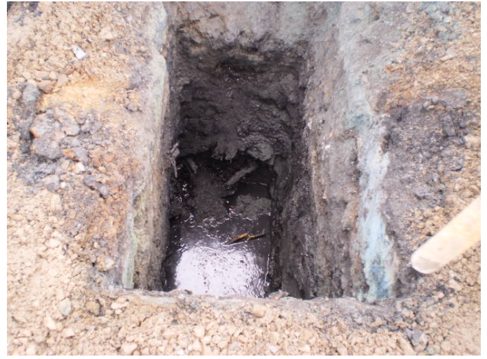
TP- 2 profile: Fine slag/foundry sand layer followed by and MGP purifier waste layer, followed by a rocky slag layer
