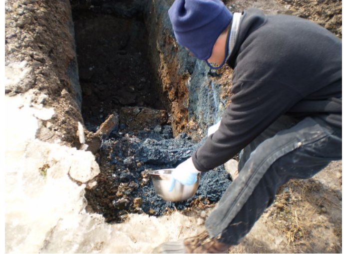
TP- 7 profile: layer of MGP purifier waste followed by rocky, cemented slag
