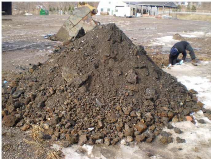
Mostly rocky slag fill spoils, with cemented layers, unable to penetrate bottom layer
