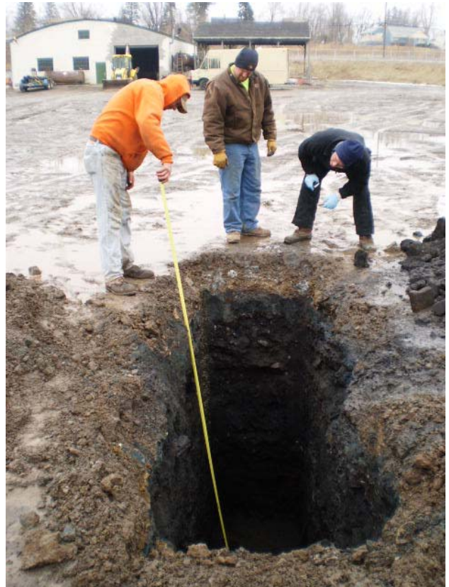
Completed test pit, note black slag fill, TP-3 profile mostly slag waste fill
