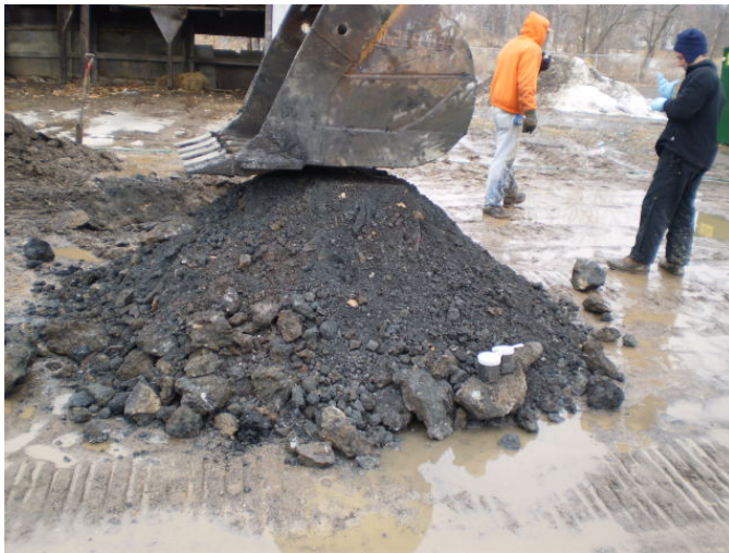
Rocky slag fill spoils with wood debris
