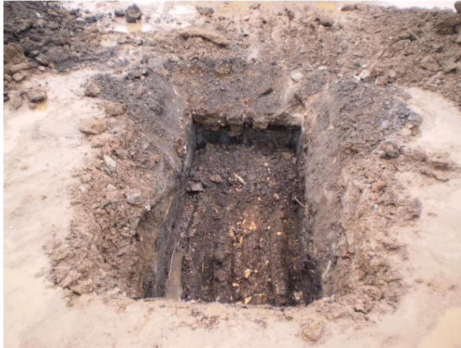
TP-4: mostly rocky slag fill, with cemented layers, unable to penetrate bottom layer
