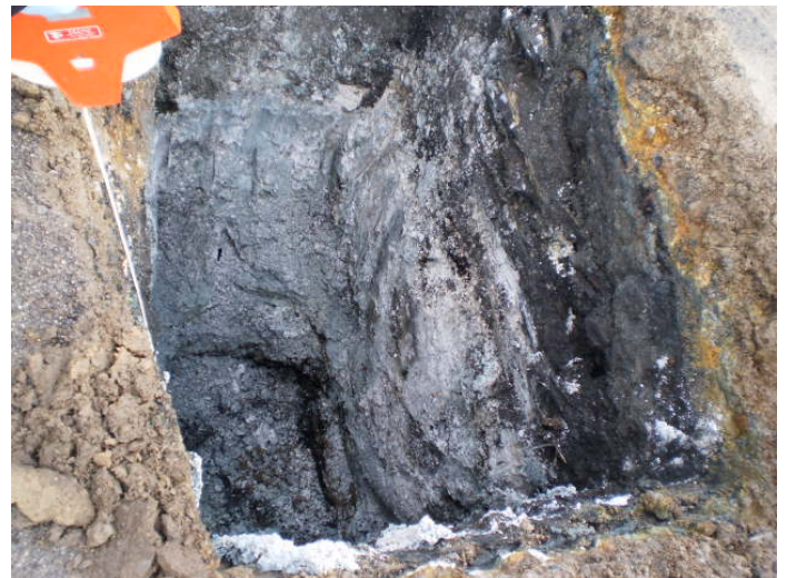
TP-1 profile: Upper layer contains slag/foundry sand like fill followed by a lime waste fill stained by MGP purifier waste
