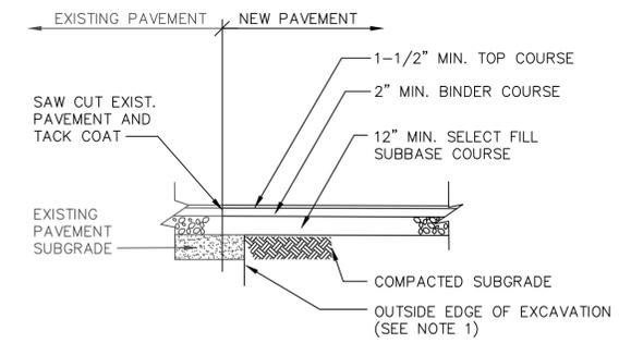
ASPHALT PAVEMENT REPLACEMENT DETAIL
