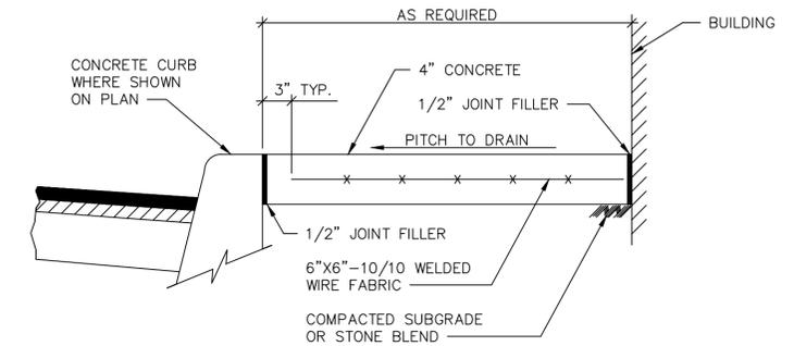
CONCRETE SIDEWALK REPLACEMENT DETAIL
