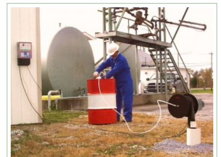
Magnum Spill Buster, Automated free phase petroleum contamination pumping system (shown with Explosion Proof Auto Seeker).
