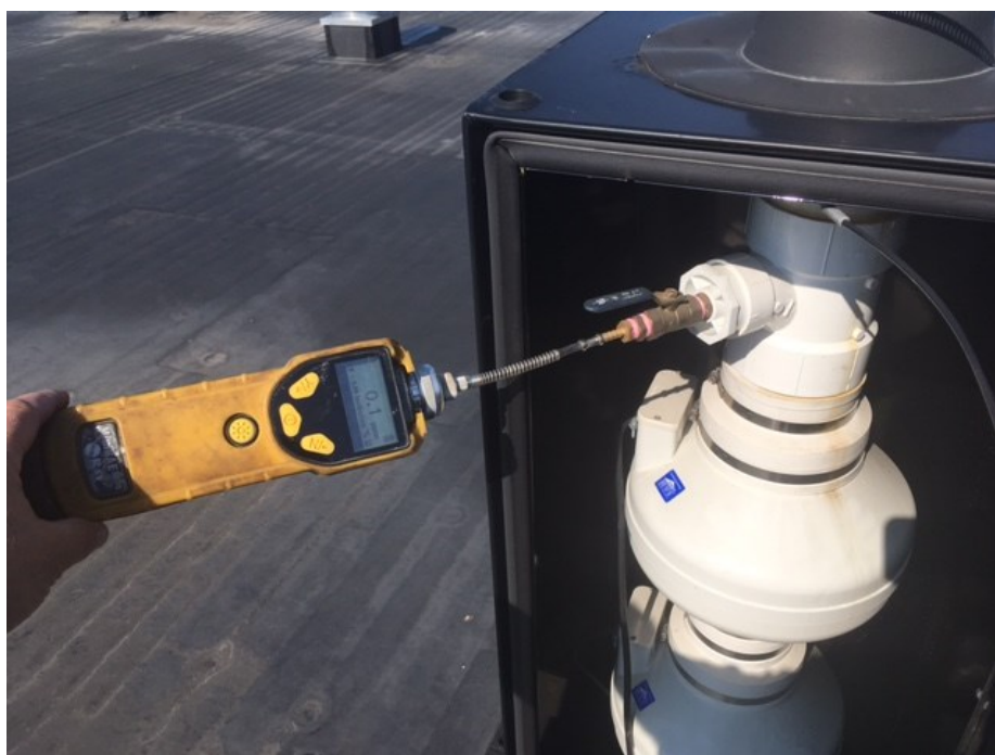
Photo #8: PID meter reading 0.1 ppmv
