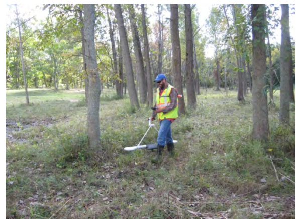
NYLD conducting the EM survey between Middle Creek and Rattlesnake Creek.
