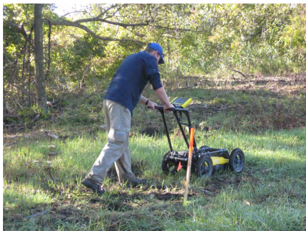
Using GPR to confirm presence of potential subsurface drums.
