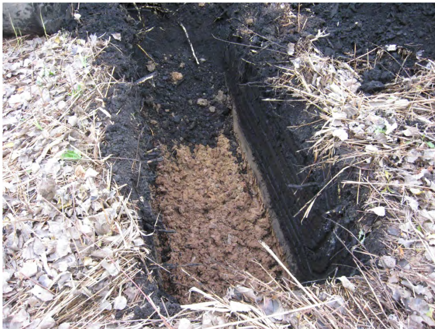
View of fill estimate test pit. Note reddish brown native clay.
