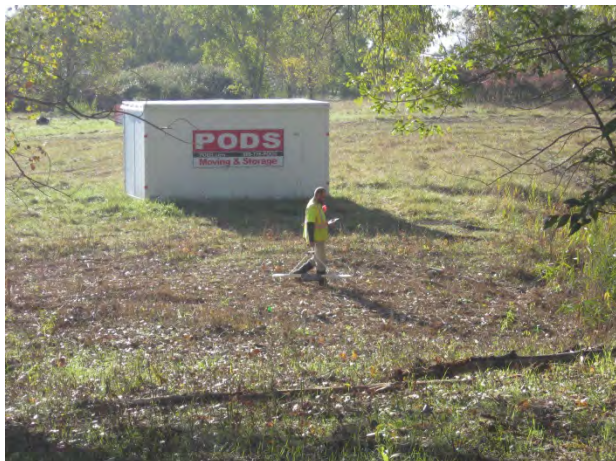
Conducting EM survey over the south creek conduit.
