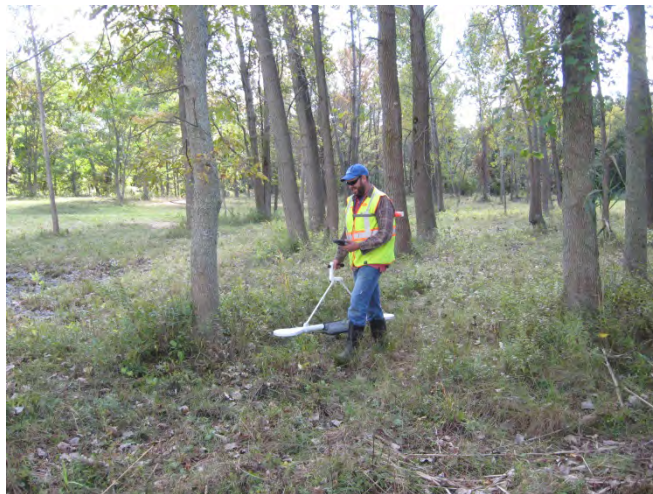
Conducting the EM survey between middle creek and Rattlesnake Creek.
