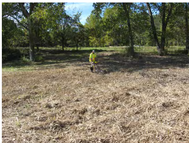
Conducting GPR survey over the south creek conduit.
