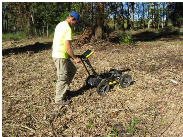
Conducting GPR survey over the Rattlesnake Creek conduit.
