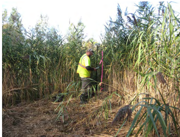
Surveying site features north of Rattlesnake Creek using RTK-GPS.
