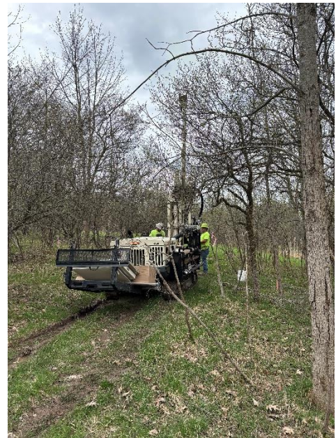
GeoProbe Rig set up & drilling at SB-A49 location
