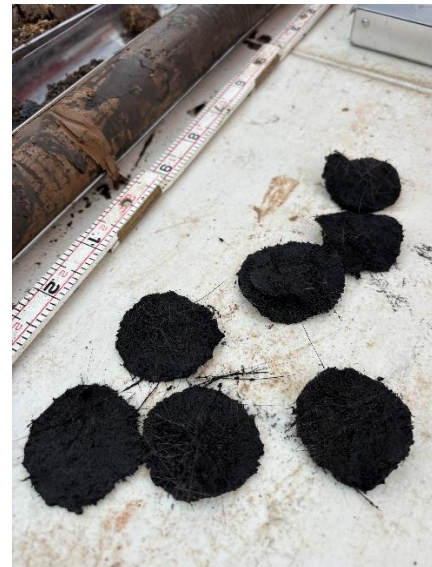
Disc-like material encountered from 10.7 to 10.9 ft bgs at boring SB-G44
