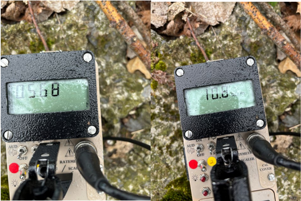
Photos from an elevated reading location showing the scaler (left) and ratemeter (right) readings
