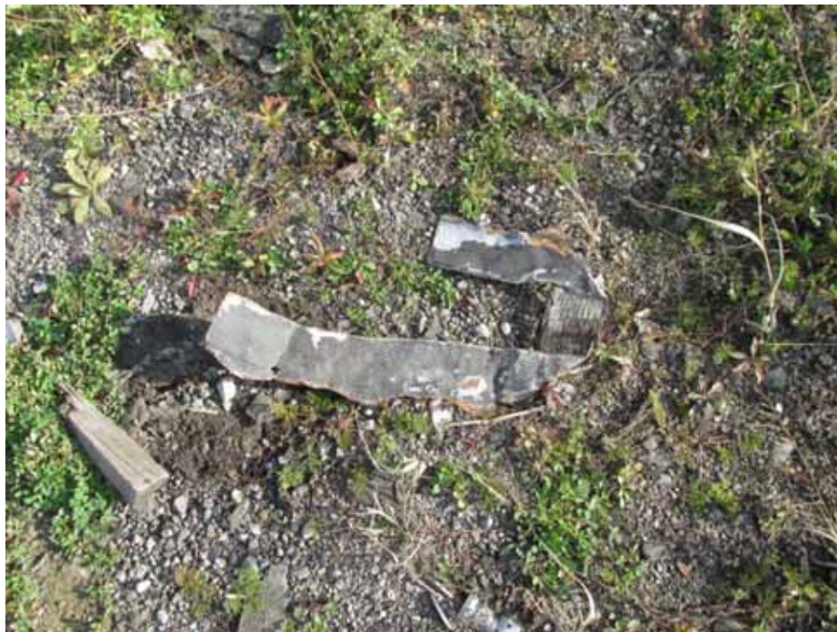
Photo 1: 11/5/13 – Example of galbestos coated metal (typical).
