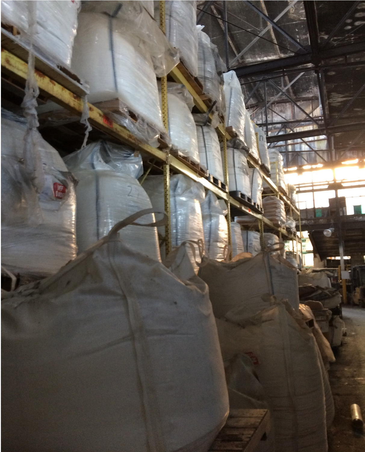
Photograph 8: View of material in super-sacks (500 – 2,500 pounds [lbs.]) overstacked in isles in Pigeon Room.
