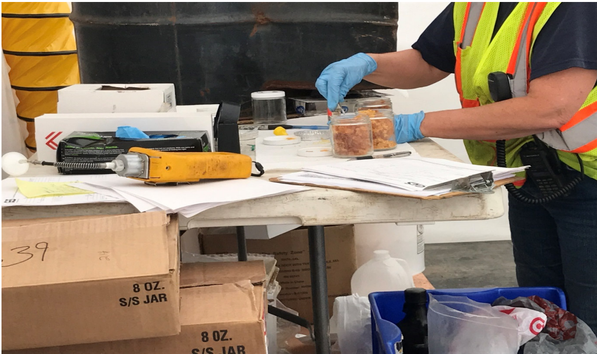
Photograph 26: View of of GES personnel performing HazCat testing.
