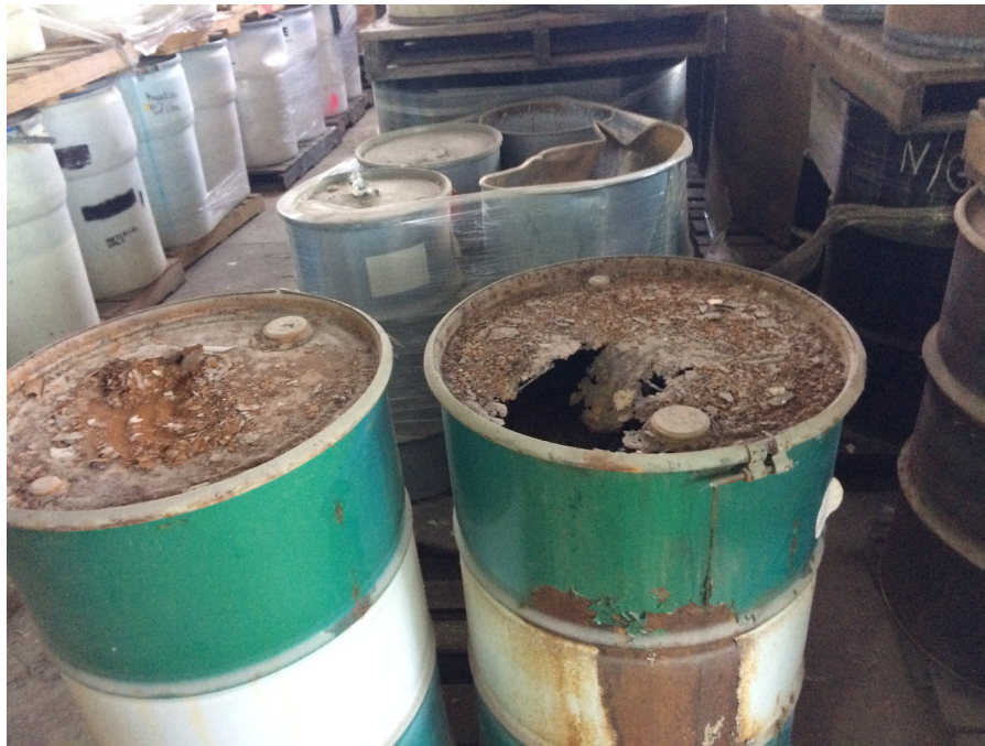
Photograph 7: View of damaged drum found in Far Back Room.
