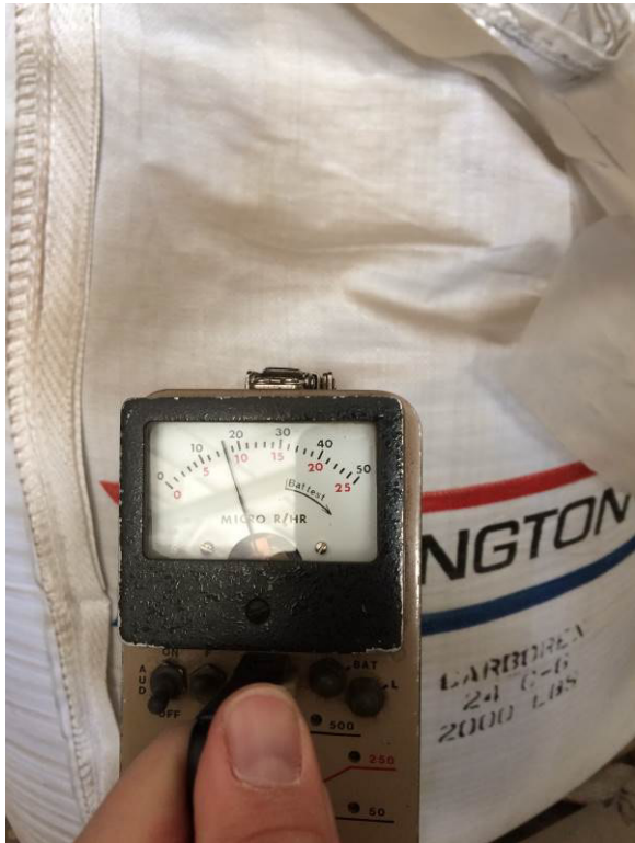
Photograph 11: View of Ludlum 19 reading approximately 18 micro roentgen per hour ( \mu\text{R/hr} ) at one of two locations where abrasive materials were stored on racks in Hallway.
