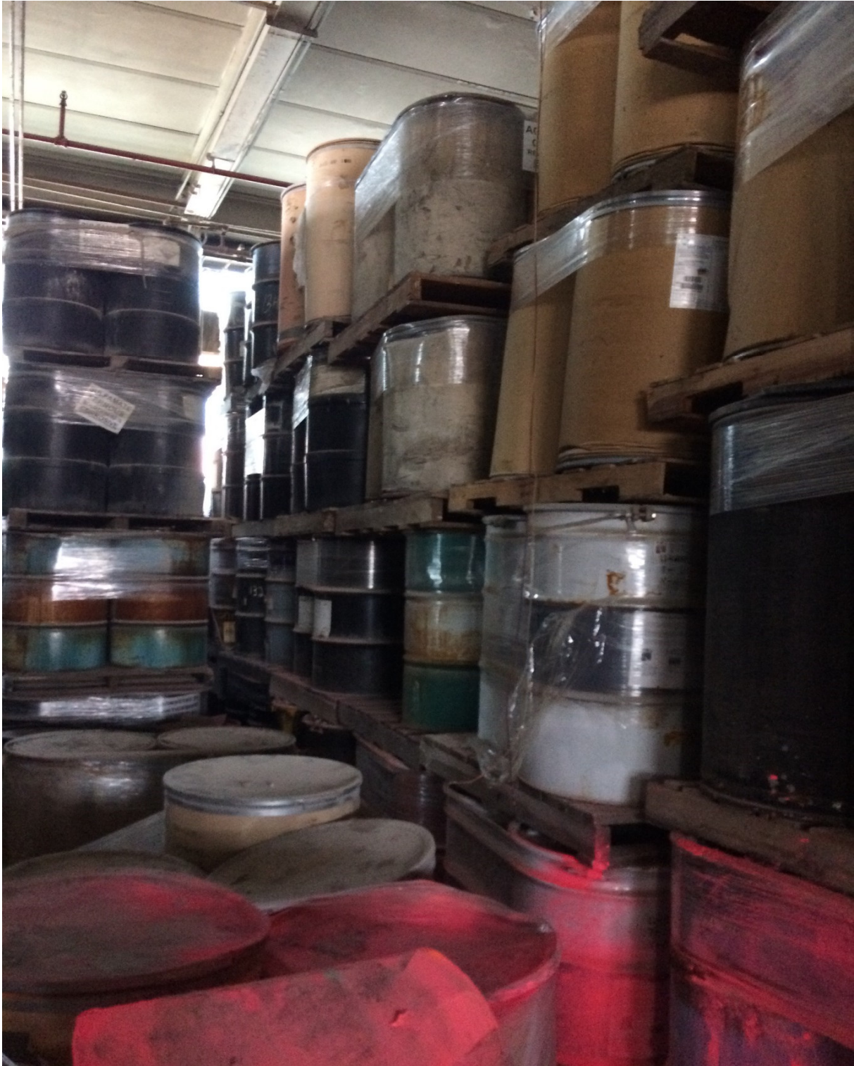
Photograph 7: View of overstacked drums (different chemicals) in Warehouse D.
