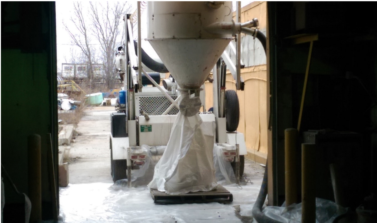
Photograph 46: View of powder material being transferred from poly drums to super-sacks using a Vacuum Unit (Hurricane 500-0339 by Industrial Vacuum).
