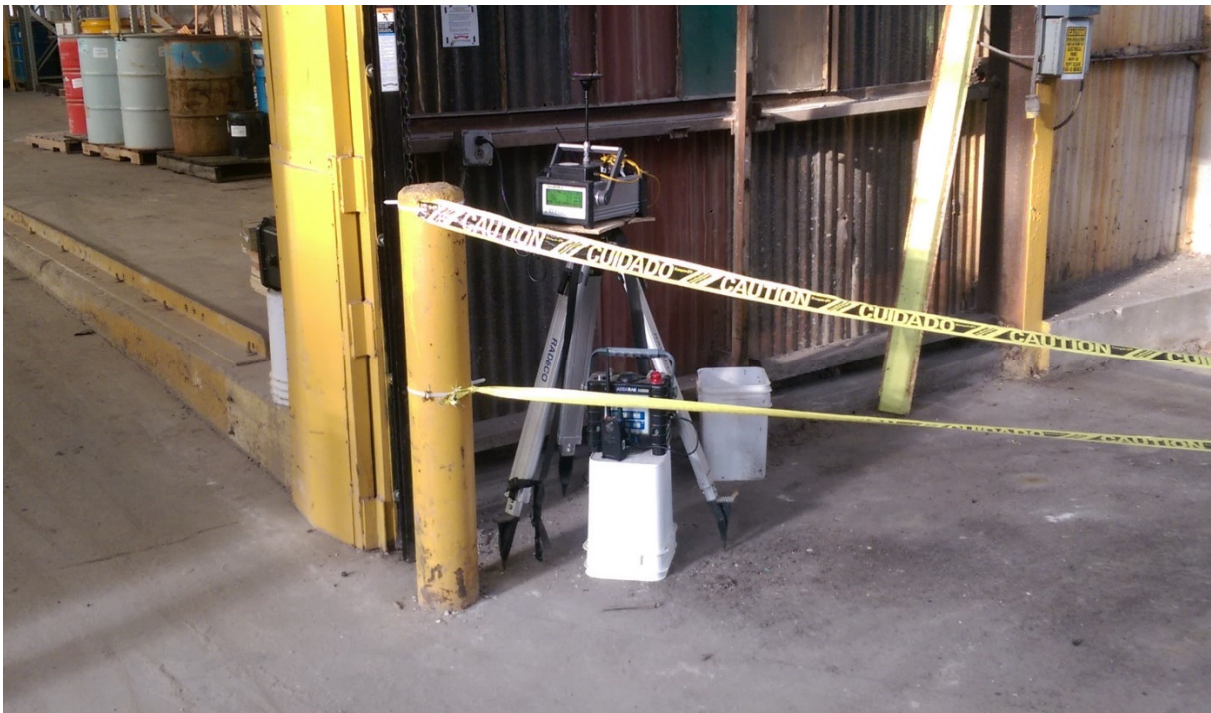
Photograph 20: View of air monitoring Station #2 comprising of a Dataram and AreaRAE in Warehouse A, entrance to Warehouse D.
