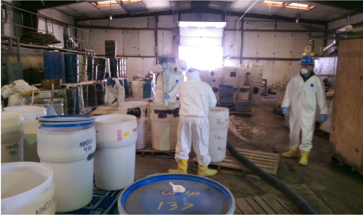
Photograph 45: View of powder material being transferred from poly drums to super-sacks.
