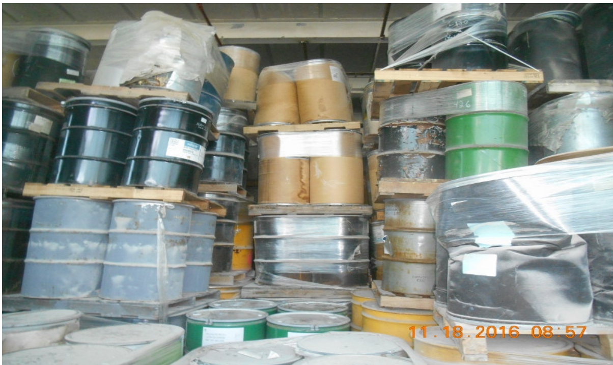
Photograph 5: View of drums piled together (flamable, corrosive, etc.) in Warehouse D.
