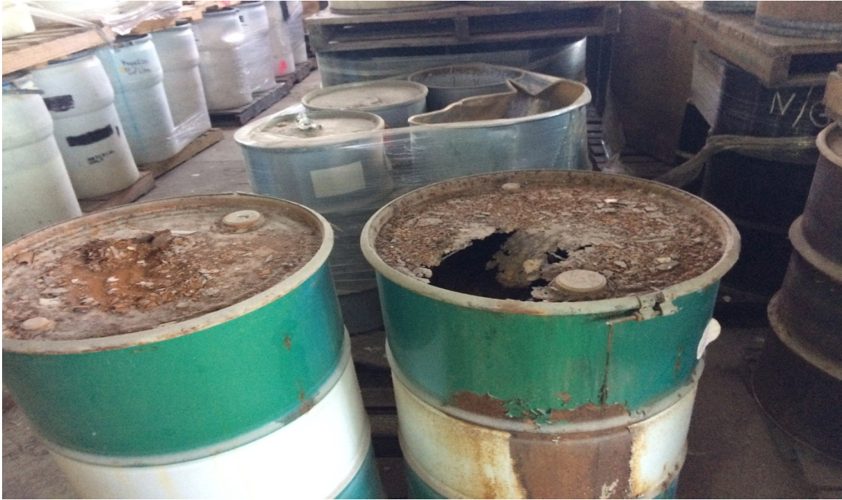
Photograph 9: View of deteriorating drums in Far Back Room.
