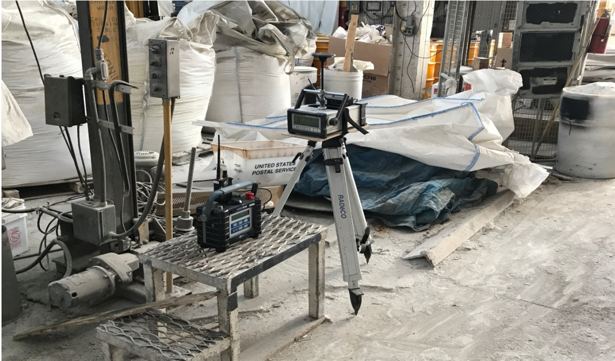
Photograph 19: View air monitoring Station #1 comprising of a Dataram and AreaRAE in Warehouse A.
