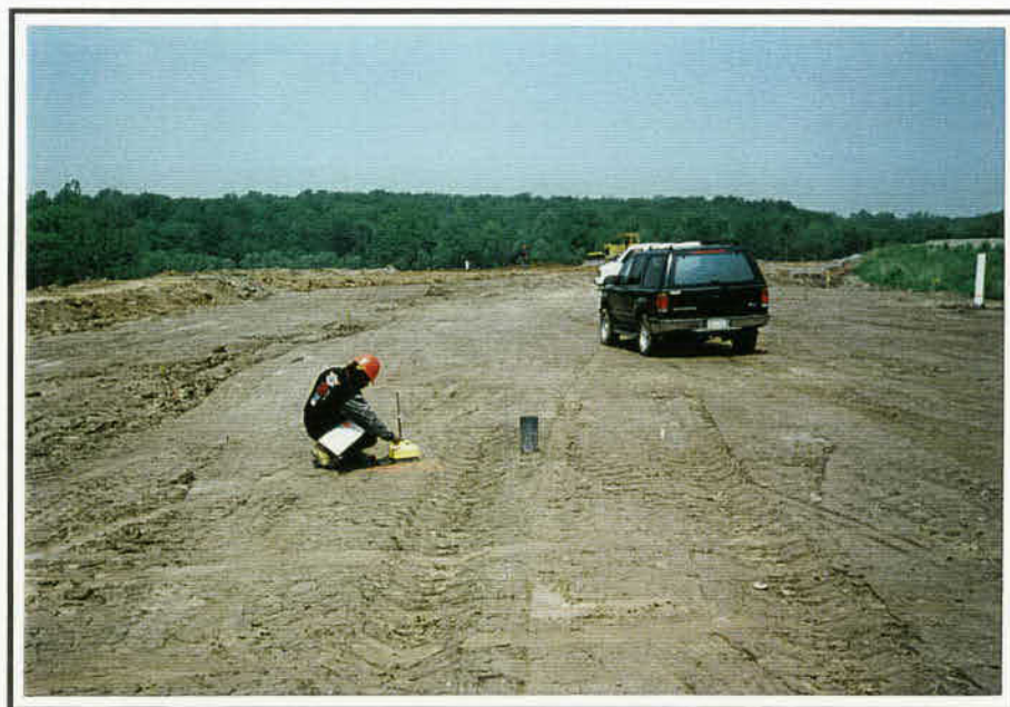
Photo #16: Moisture-Density Testing of the LPS Layer
