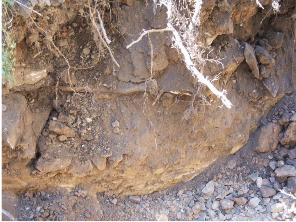
Figure 6-7. Photograph of the reworked soil in test pit SUB-60. Photograph taken by Glenn May on September 3, 2008.
