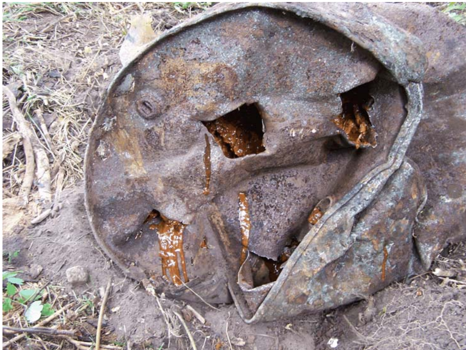
Figure 6-4. Photograph of the drum excavated from test pit SUB-8 that contained suspected paint waste. Photograph taken by Glenn May on August 28, 2008.
