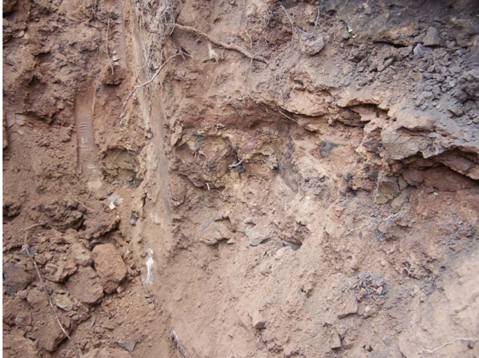
Figure 6-11. Photograph of the native silty clay in test pit SUB-78. Note the grey and black mottling in the center of the photo. Photograph taken by Glenn May on September 5, 2008.
