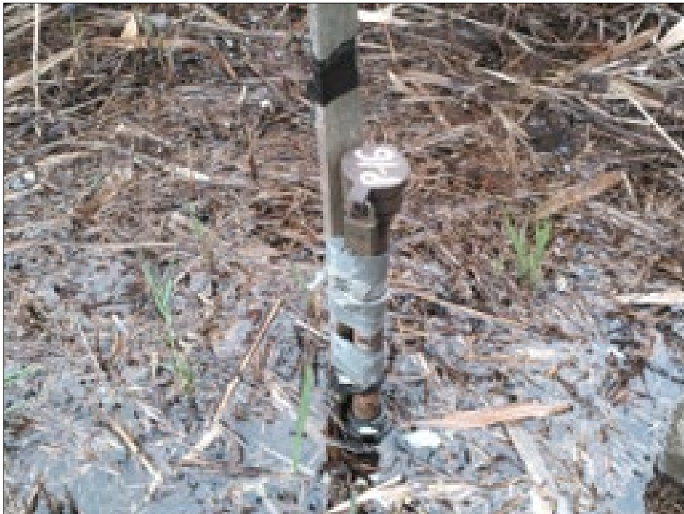
Photo 4 View of P-16 with temporary repair observed on October 6, 2021. A permanent repair was not able to be completed due to the saturated conditions at the well.
