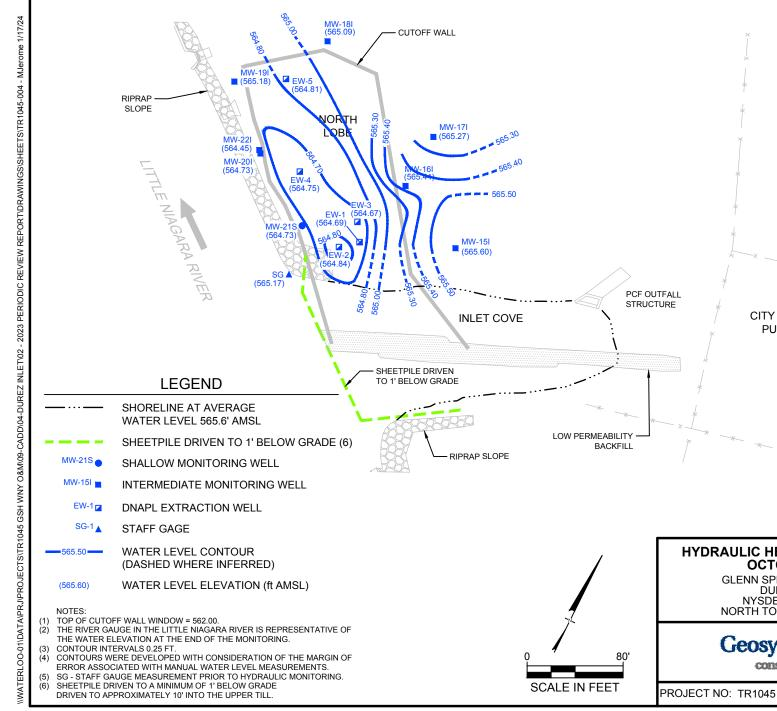
HYDRAULIC HEAD DISTRIBUTION MAP **OCTOBER 30, 2023** GLENN SPRINGS HOLDINGS, INC. DUREZ INLET SITE NYSDEC SITE NO. 932018 NORTH TONAWANDA, NEW YORK **Geosyntec**<sup>▶</sup> FIGURE
