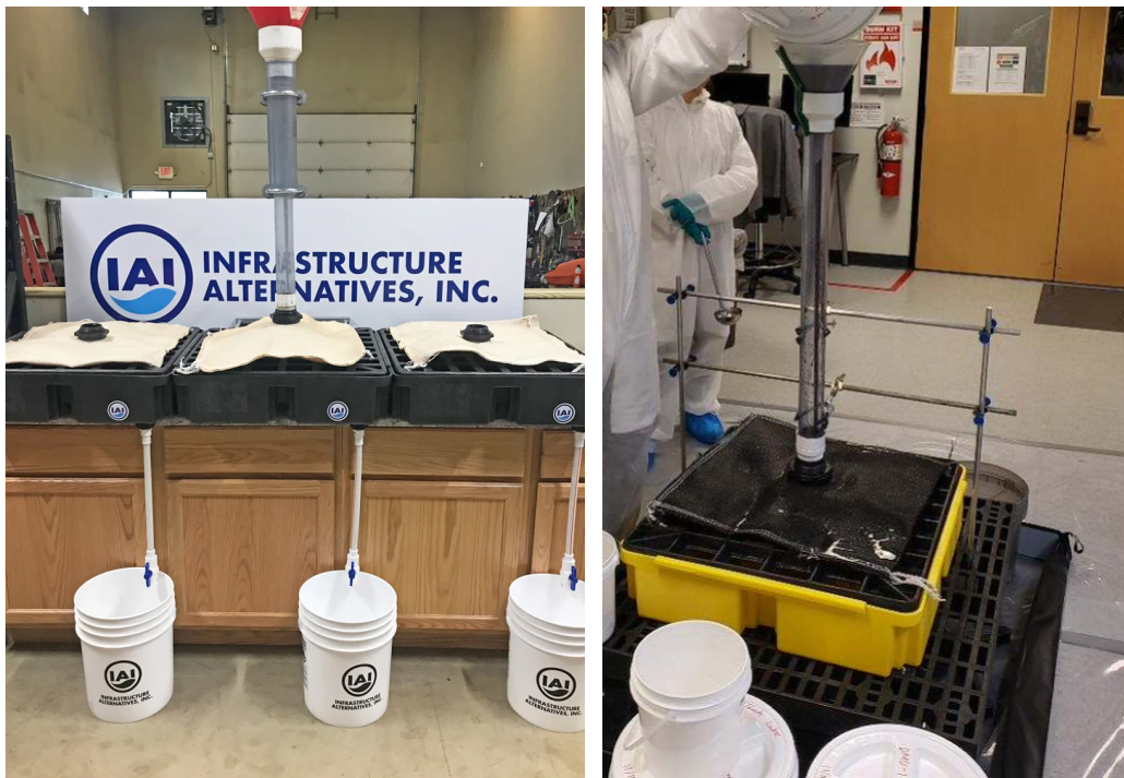
Figure 1 Example of Geotextile Tube Setup to Collect Filtrate
