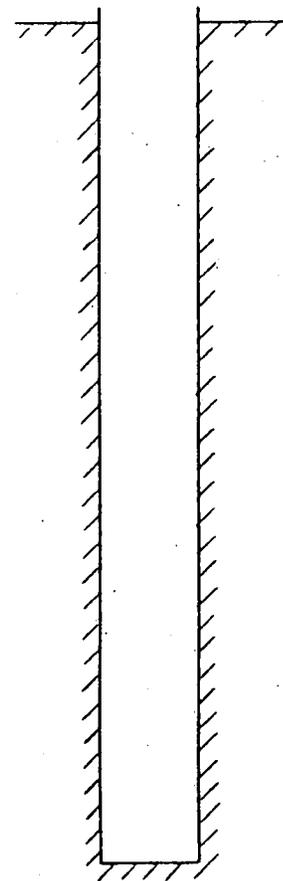
CASING ADVANCED TO NEXT SAMPLING INTERVAL AND CLEANED OUT
