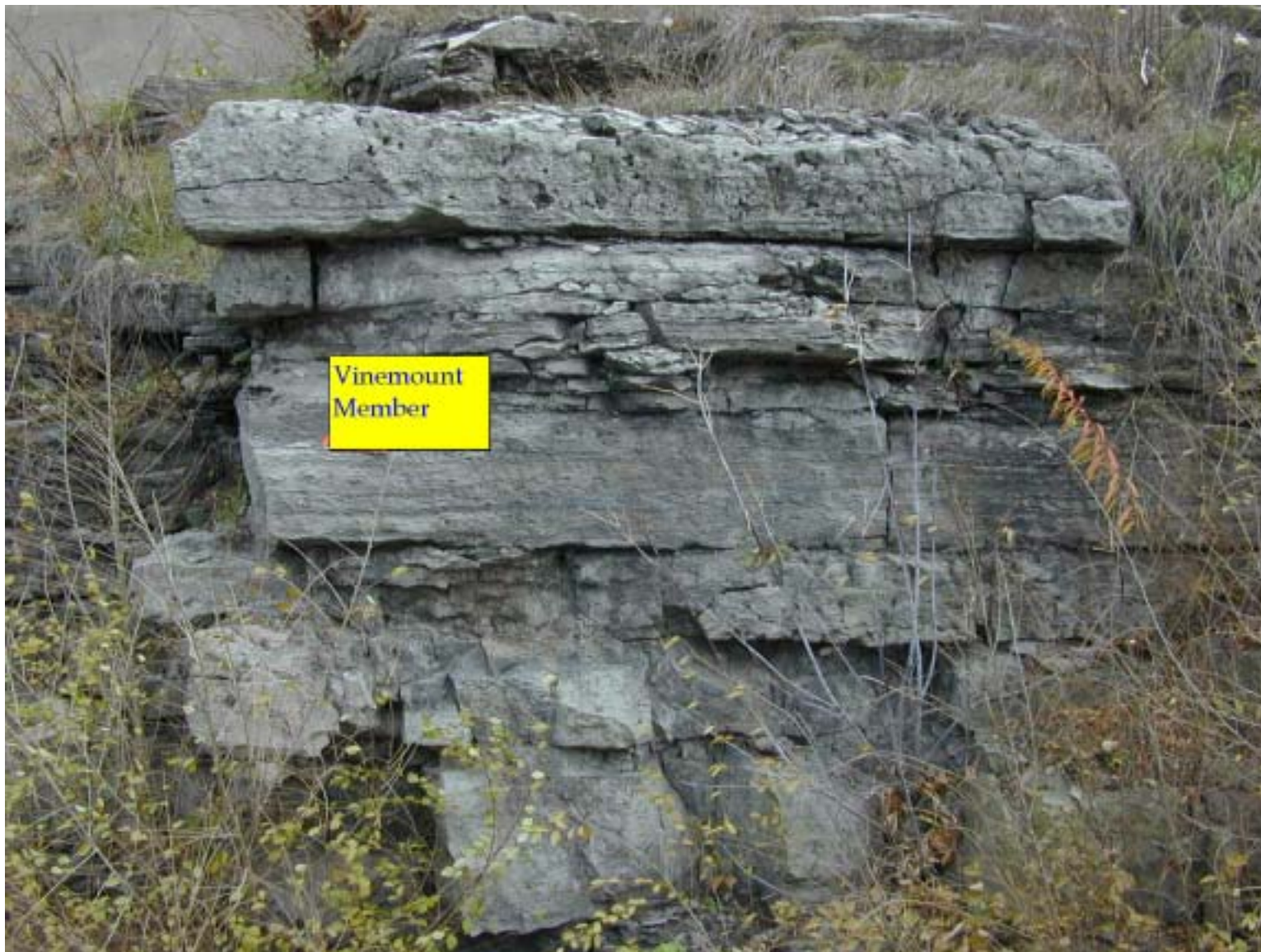
Photograph 1. Horizontal bedding, bedding plane fractures, and vertical fractures in the Vinemount Member of the Goat Island Formation. NYPA Access Road.
