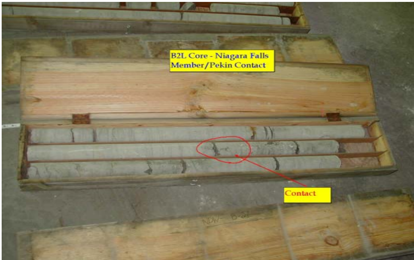
Photograph 17. B2L core showing Niagara Falls Member/Pekin Member contact.
