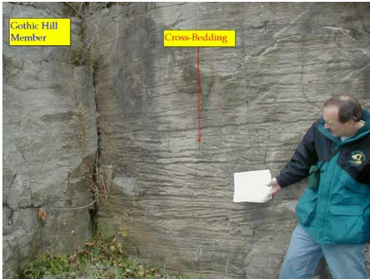
Photograph 8. Cross-bedding within the coarse-grained Gothic Hill Member of the Gasport Formation. Note the vertical joint and lack of bedding plane fractures. NYPA Access Road.
