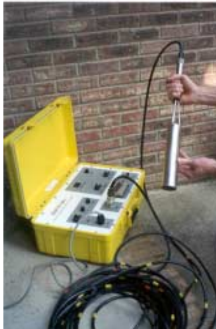
Figure 2: The Electromagnetic Borehole Flowmeter System
