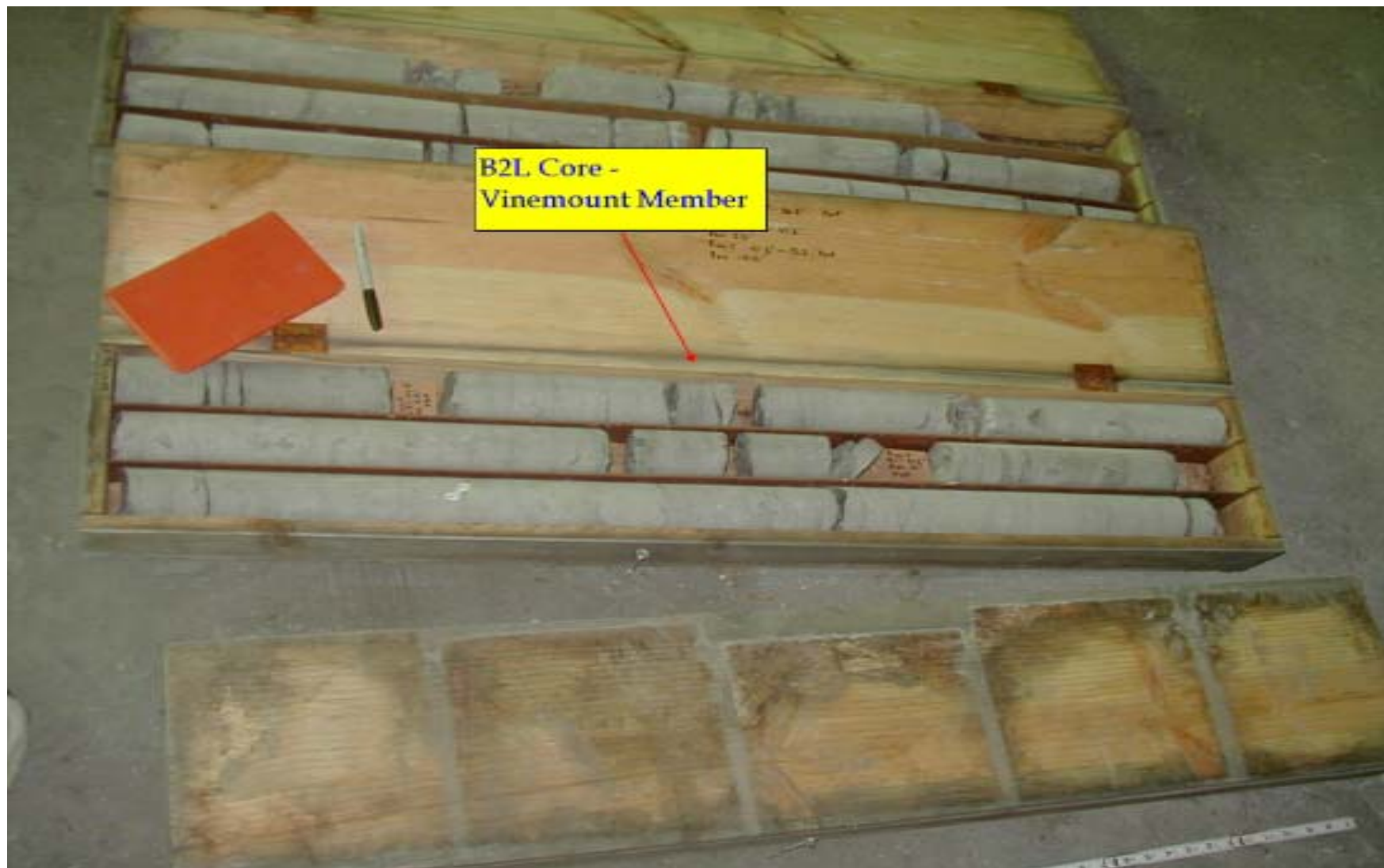
Photograph 14. B2L core showing Vinemount Member of Goat Island Formation.
