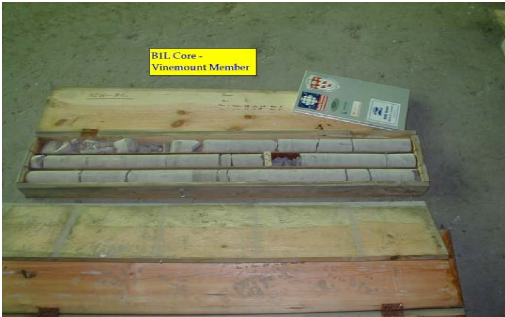
Photograph 15. B1L core showing Vinemount Member of Goat Island Formation.
