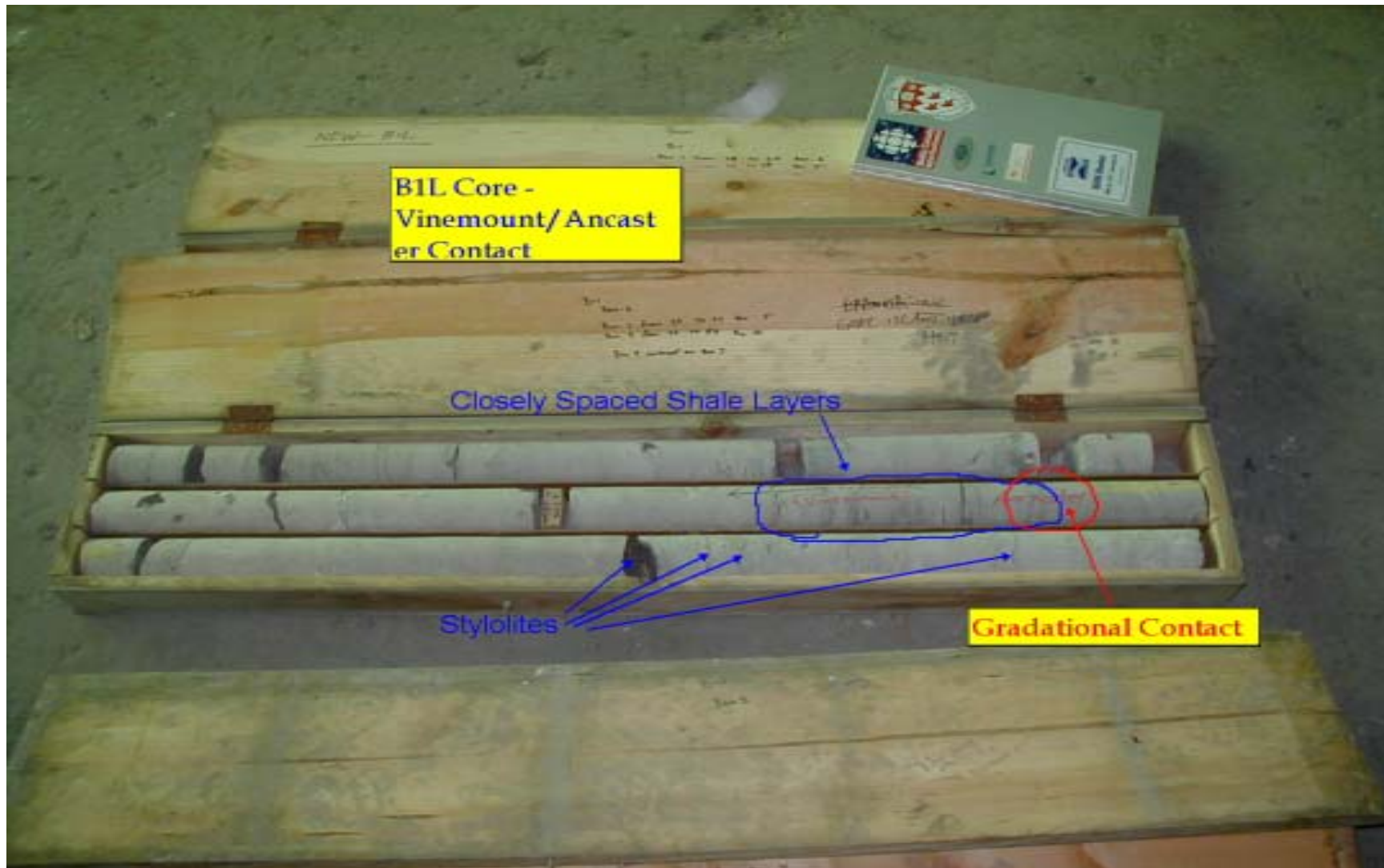
Photograph 16. B1L core showing Vinemount Member/Ancaster Member contact.
