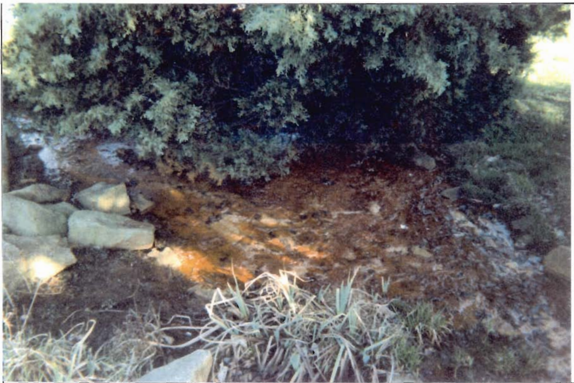
D-13 Botanical Gardens. Facing south. Exfiltrating groundwater flowing in water fountain overflow channel. Note iron staining. April 7, 1998.
