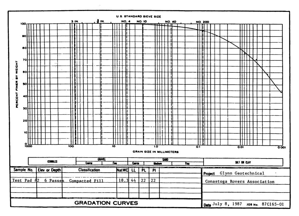
CLIENT: GLYNN GEDTECHNICAL PROJECT LOCATION: CONASTOGA ROVERS SAMPLE NO.: TEST PAD 2 DESCRIPTION:8 PASSES COMPACTED FILL CLAY
