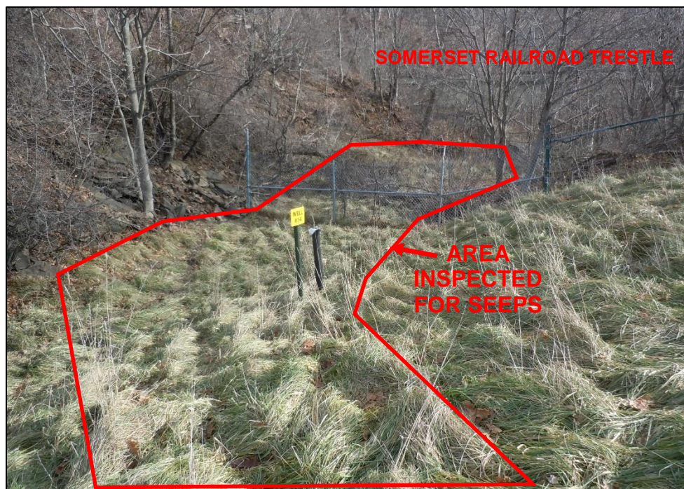
Southeastward view (downslope) near monitoring well VDM-14 showing area inspected for leachate seeps.
