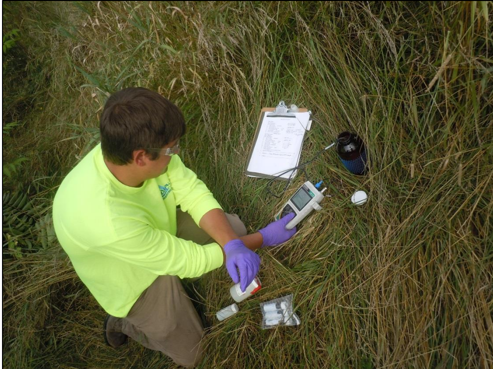
Taking sample pH measurement at well VDM-9R.
