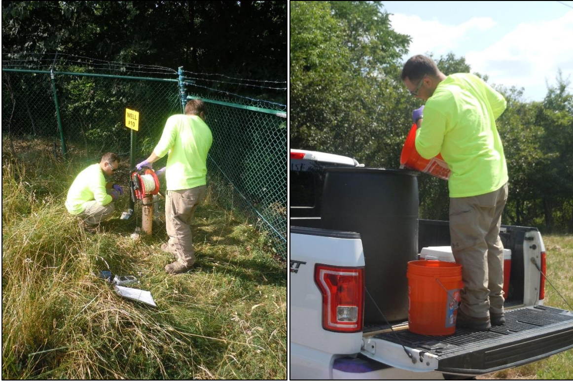
Taking depth to water and bottom measurements at well VDM-10 (left) and containerizing purge water for future characterization and disposal (right).
