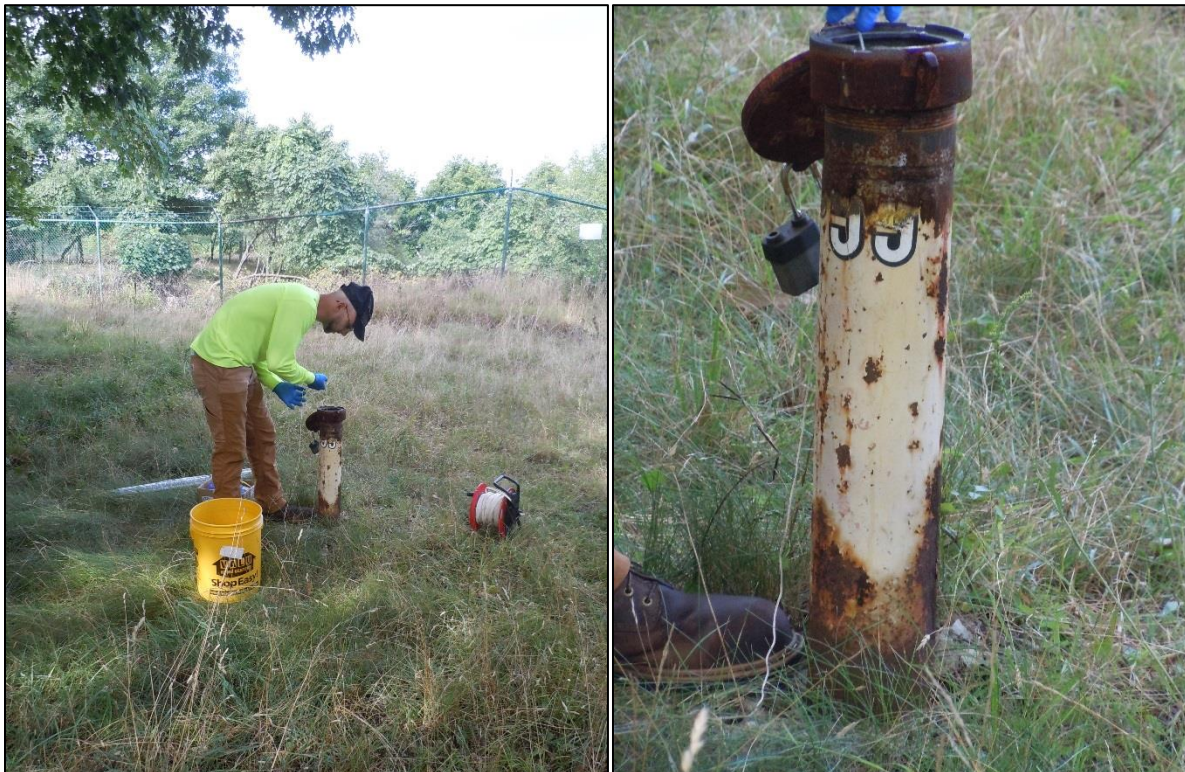
Views of upgradient monitoring well D-55. Top of protective casing was repaired.
