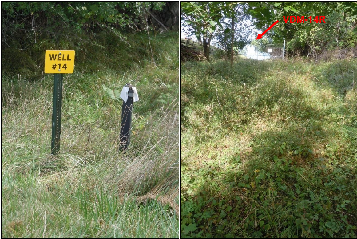
Closeup view of monitoring well VDM-14R (left) and a view from outside the landfill upslope toward VDM-14R (right) showing no signs of seeps.
