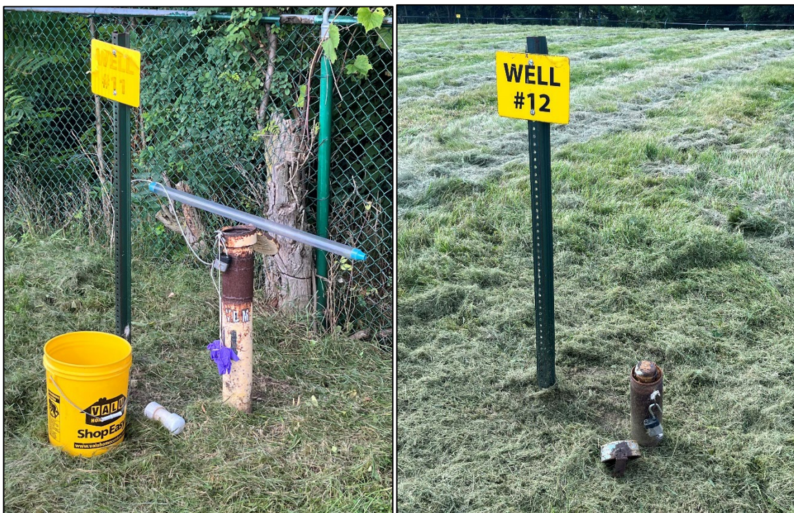
Views of monitoring wells VDM-11 and VDM-12. Note dedicated bailer used for purging/sampling on VDM-11.
