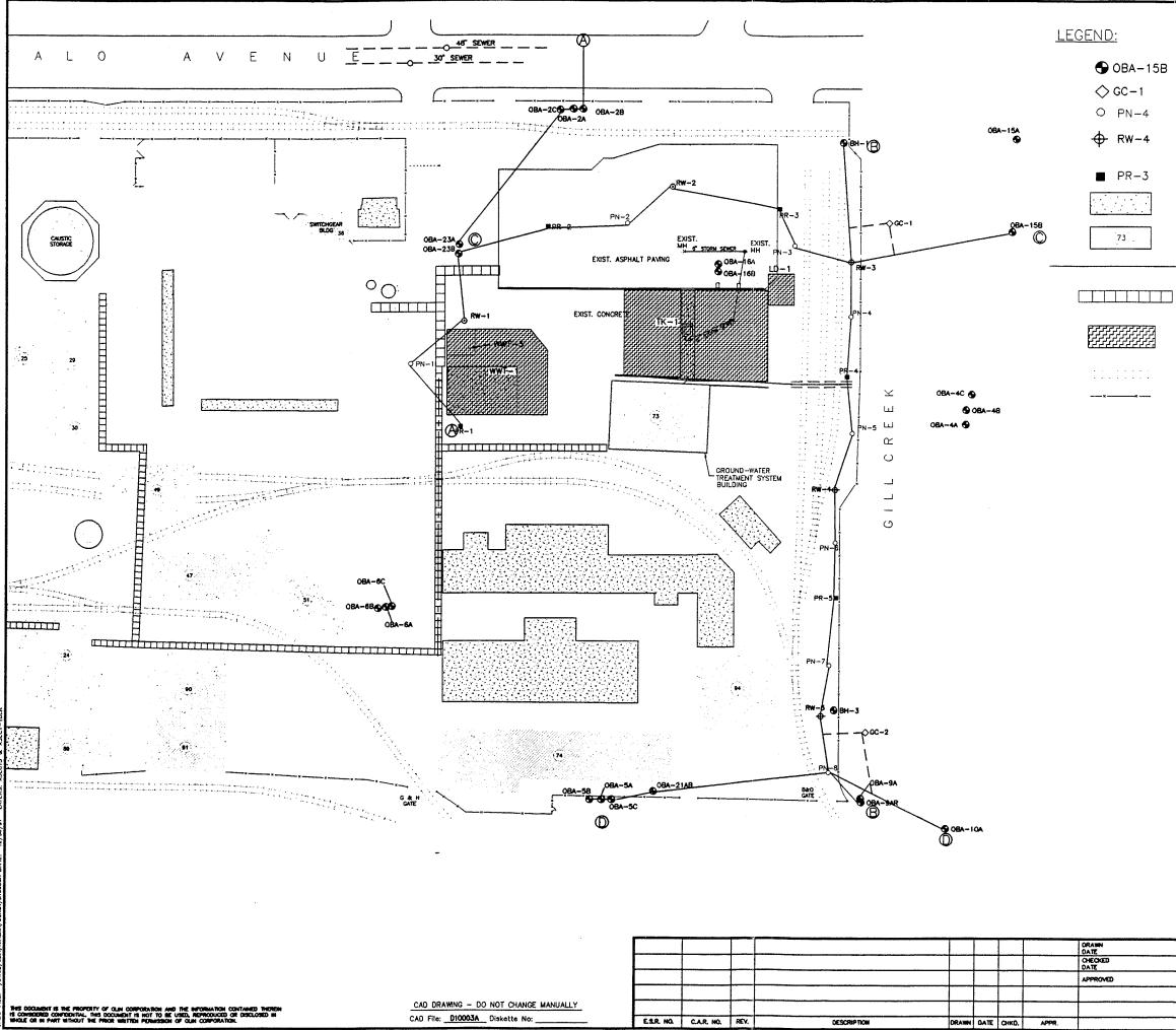
WATER QUALITY MONITORING WELLS GILL CREEK MONITORING POINTS A/B-ZONE PIEZOMETER NESTS GROUND-WATER RECOVERY WELLS PASSIVE RELIEF WELLS CONCRETE SLAB (FORMER BUILDING OR EQUIPMENT FOUNDATION) REMAINING BUILDING AND BUILDING NUMBER OLIN PROPERTY LINE EXSITING PIPE BRIDGE APPROXIMATE LIMITS OF IDENTIFIED SOLID WASTE MANAGEMENT UNITS RAILROAD TRACKS FENCE LINE
