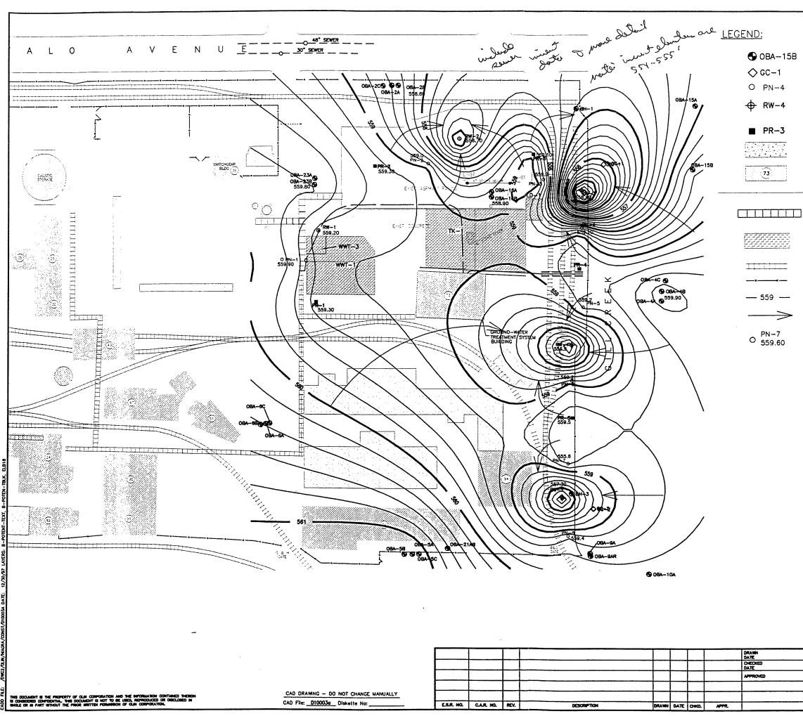
WATER QUALITY MONITORING WELLS GILL CREEK MONITORING POINTS A/B-ZONE PIEZOMETER NESTS GROUND-WATER RECOVERY WELLS PASSIVE RELIEF WELLS CONCRETE SLAB (FORMER BUILDING OR EQUIPMENT FOUNDATION) REMAINING BUILDING AND BUILDING NUMBER OLIN PROPERTY LINE EXSITING PIPE BRIDGE APPROXIMATE LIMITS OF IDENTIFIED SOLID WASTE MANAGEMENT UNITS RAILROAD TRACKS FENCE LINE GROUND-WATER ELEVATION CONTOUR LINE GROUND-WATER FLOW DIRECTION WELL ID WITH MEASURED GROUND-WATER ELEVATION (FEET)
