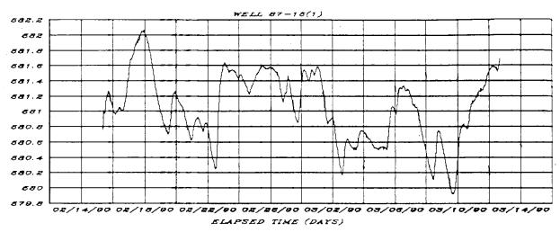
NOTE: FLUCTUATIONS DUE TO DISCHARGE OF WATER FROM ROCKET TESTS.
