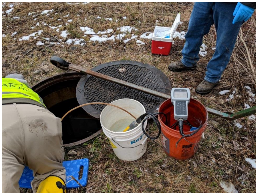
Checking field parameters for purge from monitoring well EW-4
