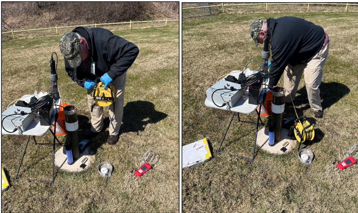
Performing air monitoring and depth to water/bottom measurements at 19-01(1) (left; red meter is combination PID/H 2 S/LEL/O 2 meter) and purging well 19-01(1) (right).
