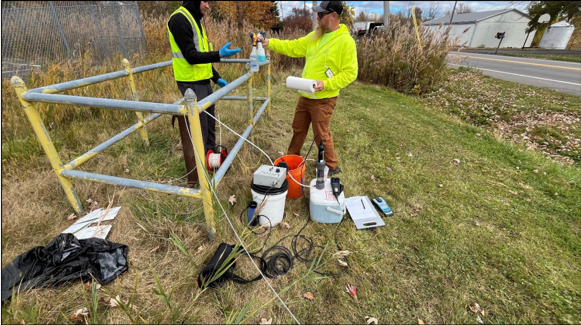
On 10-24-2024, APTIM crew performing depth to water/bottom measurements and preparing to low-flow purge/sample well 87-19(1) with a peristaltic pump.
