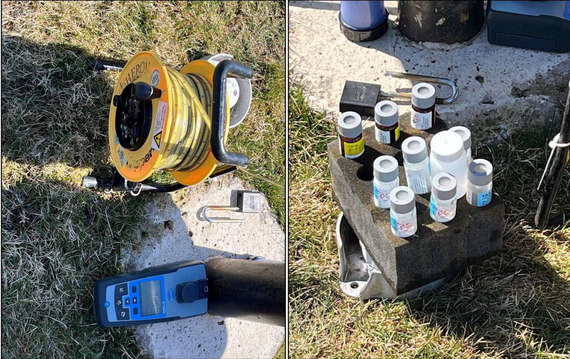
Heron Dipper-T electronic water level indicator and Hach 2100Q Turbidimeter (left) and Sample Bottle Set (right).
