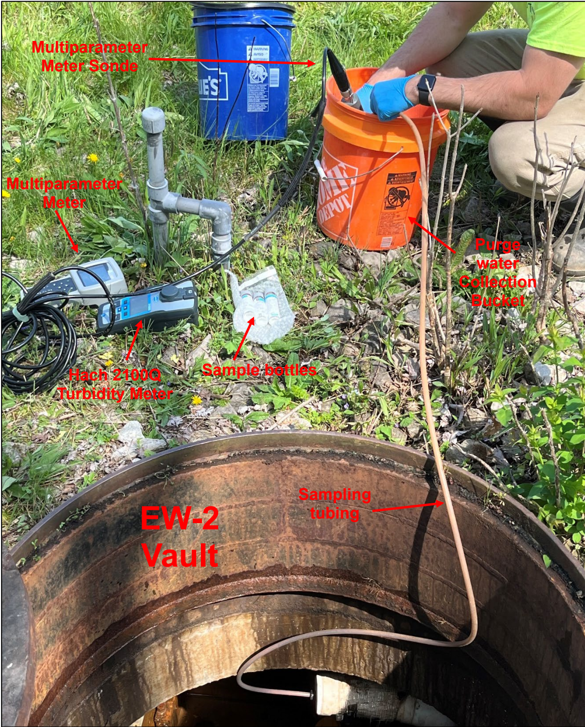
Sampling equipment setup at extraction well EW-2.
