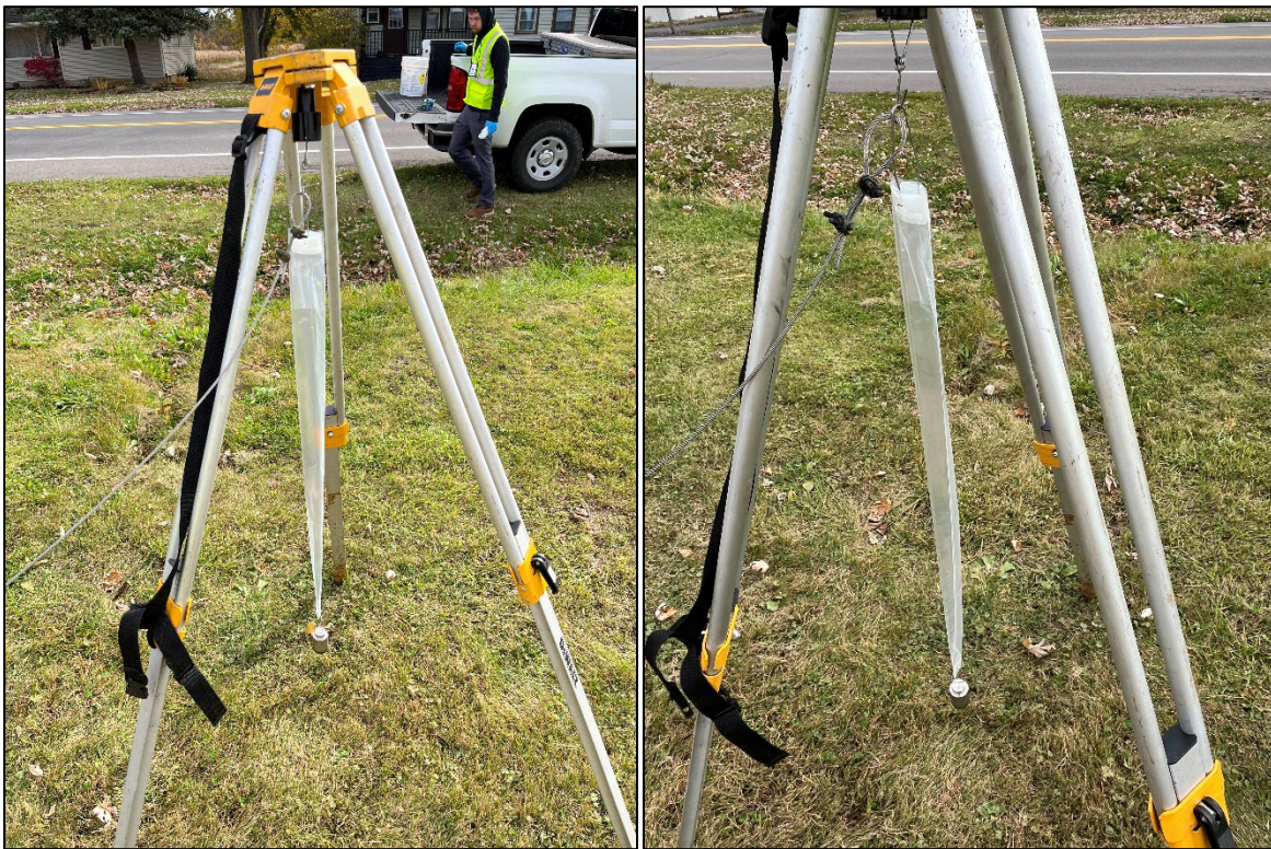
On 10-24-2024, views of a HydraSleeve sampler removed from well 87-19(1). APTIM is performing a pilot test of HydraSleeve samplers in 5 wells; samples were also collected via low-flow techniques with a peristaltic pump for analytical results comparisons.
