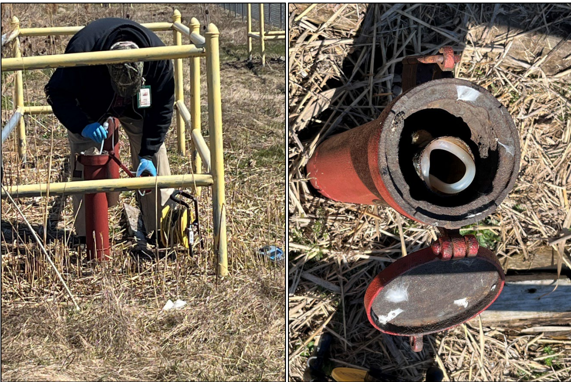
Taking water level/depth to bottom measurements at 87-14(1) (left) and 87-14(1) well head (right).
