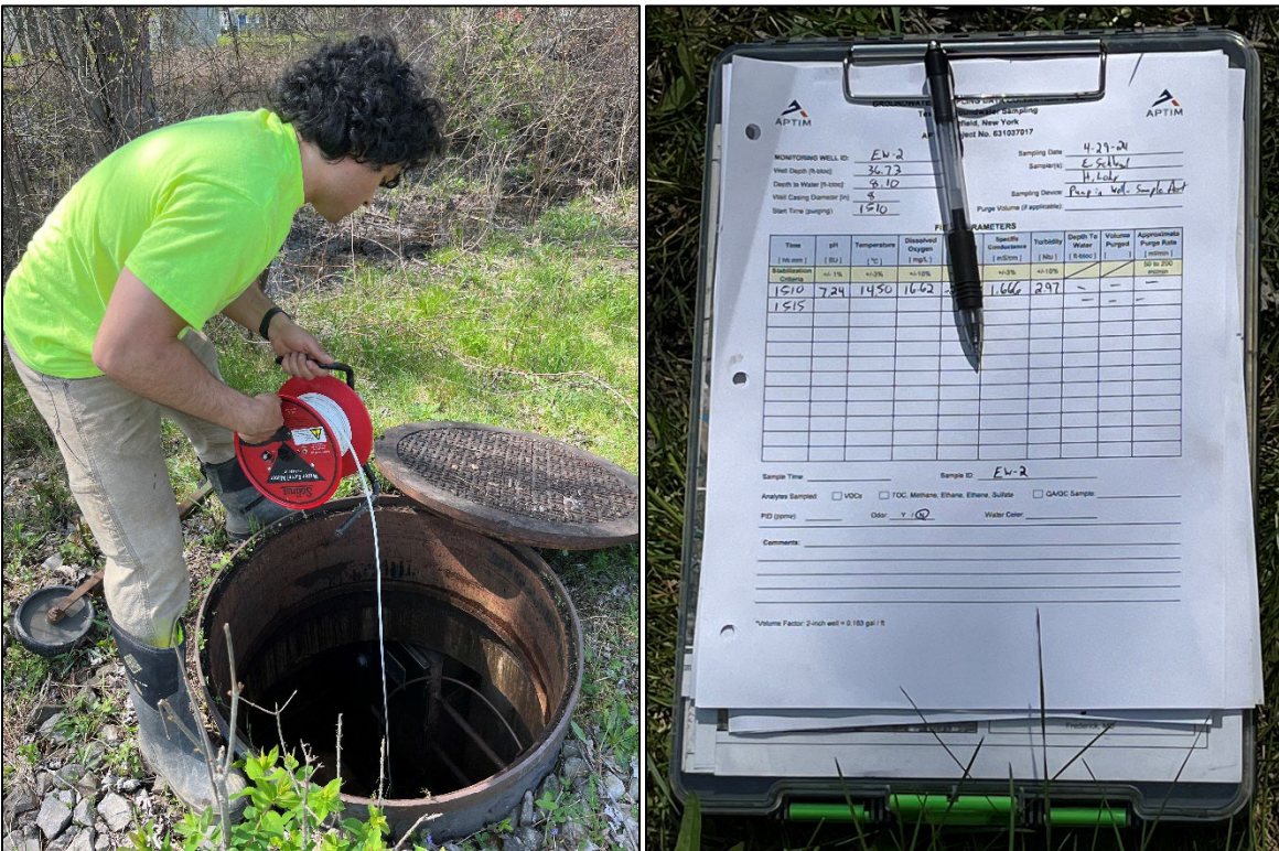
Taking water level/depth to bottom measurements at EW-2 (left) and field sampling log sheet (right).
