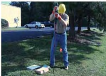
Slide hammer and tile probe
