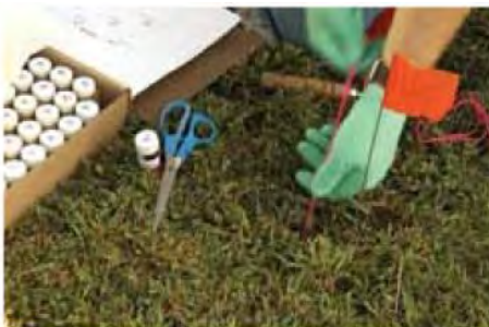
Pull string to remove sampler from hole
