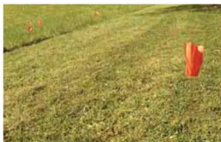
Lay out sampling grid prior to drilling holes
