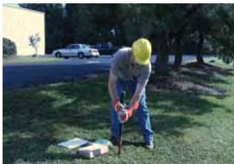
Make 0.5 to 1 inch hole 36 inches (1m) deep
